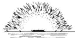
**Figure 6.39** Schematics of telltale features of parallel machining cracks. These origins are common in biaxial disks, pressure-loaded plates, and transversely-ground flexural or tension strength specimens. Low-angle grazing illumination facilitates their detection with optical microscopy. Some have elongated mirrors along the surface, an important telltale sign.
