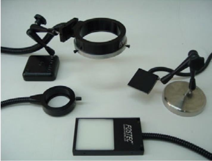
*Figure 3.16* Illumination sources for use with a stereomicroscope. Clockwise from the middle left: a ring light intended to be clamped to the objective lens, a ring dark light illuminator on an adjustable stand, a line light source on a stand, and a transmitted light platform.
