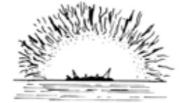
(e) “V machining crack”
