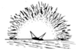
(f) “coarse grinding parallel crack”
