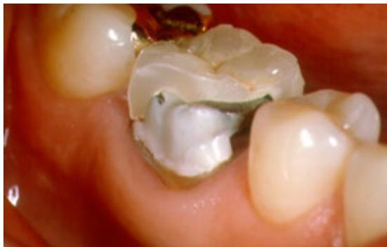
**Figure 10.23** A fractured Dicor<sup>®</sup> glass ceramic molar crown. (courtesy of S. Scherrer)
