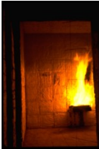
Figure 5.15: Photo of a 100 kW fire with the burner located against the rear wall of one of the small compartments in the NBS Multi-Compartment test Series.
