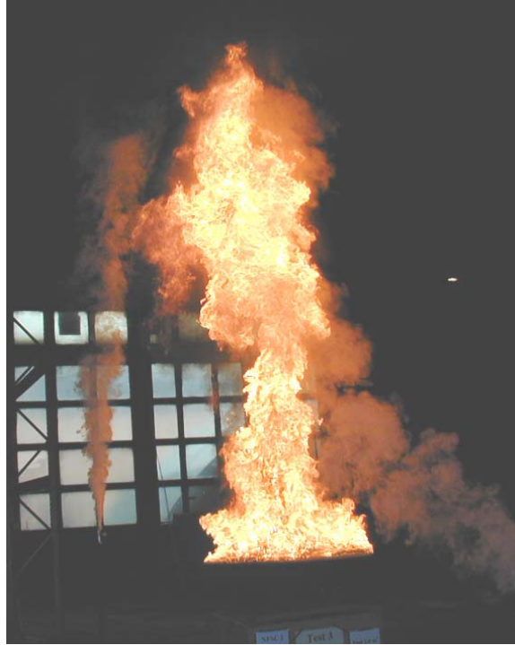
Figure 5.4: Photo of a 2 MW heptane fire during the VTT large hall tests. Photo provided by Simo Hostikka, VTT.
