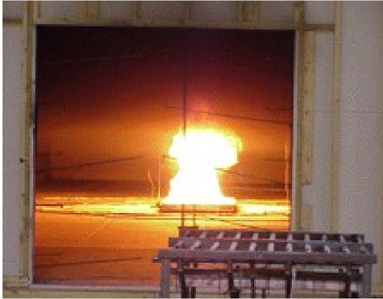
Figure 5.6: Photograph of a 1 MW heptane fire seen through the open doorway. Photo provided by Anthony Hamins, NIST.
