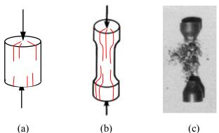
**Figure 4.31** Compression strength specimens. Cylindrical specimens (a), are very susceptible to end splitting shown by the red cracks. Dumbbell specimens (b) are also susceptible to end splitting if the loading anvils are not carefully chosen or are misaligned. (c) shows a valid compression fracture whereby the gage section is pulverized but the end caps are intact. (c is courtesy C. Tracy).
