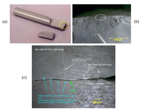
**Figure 6.29** A fractured silicon nitride pin. Examination of the fracture surface (b) alone might lead one to conclude that machining damage was the origin flaw, but closer examination of the outer surface (c) shows it actually was a scratch. Notice how the origin flaw has the same arc as the scratch.
