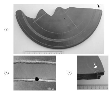
**Figure 10.16** Fractured SiC furnace setter plate (a). The curvy pattern is typical of a center-heated plate fracture as shown in Chapter 4. The arrow marks the origin which is a hole through the plate. The machined grooves were chipped and had ragged edges as shown in (b). The plate was 36 cm round and 1.9 cm thick. (c) shows the origin hole from the bottom surface. There is spall and evidence of a chemical reaction with a mounting bolt or washer. (plate courtesy of B. Mikijelj)
