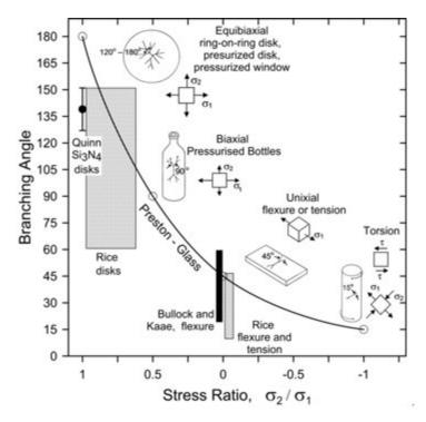
**Figure 4.4** Branching angle versus stress state. The solid line is the trend for glass shown by Preston.<sup>2</sup> The shaded bands show Rice's data<sup>4</sup> ranges for several ceramics and Bullock and Kaae's range for a glassy carbon.<sup>5</sup> The author's data for silicon nitride ring-on-ring disks are also shown.<sup>6</sup>
