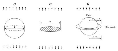
*Figure 7.27 Factors that cause calculated and measured crack sizes to differ (continued on next page)*
