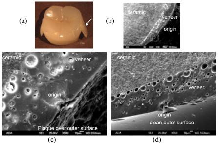
**Figure 6.63** Dental plaque is a common contaminant on ceramic restorations. (a) shows the broken middle ("pontic") piece of a lithium disilicate bridge that broke after 7 weeks in vivo. (b) shows the overall fracture surface. (c) and (d) show the origin site before and after cleaning to removal plaque. Plaque can be removed with bleach as described on page 3-6. See Figure 6.74 for additional images of this bridge.
