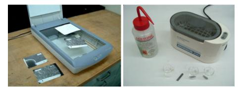
*Figure 3.60* Other useful equipment for a fractography laboratory. Digital scanner (a) and ultrasonic cleaning bath (b).
