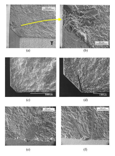
**Figure 6.22** Examples of large grain fracture origins. (a,b) show a cluster of large grains at a chamfer in a 99.9% alumina bend bar. (c,d) show an oversized grain in a silicon nitride. The material had small interlocking elongated grains intended to enhance fracture toughness. Notice how these are legitimate material flaws, and the chamfer preparation was completely satisfactory. (e, f) show examples of acicular large grains in sintered alpha silicon carbide.
