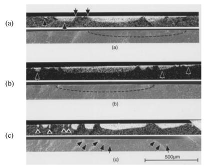
**Figure 3.58** Grinding cracks in silicon nitride revealed by palladium nitrate solution impregnation. These are paired views of fracture surfaces for three different specimens. The first image in a pair is a palladium map. The second is a conventional backscattered SEM image at the same magnification. (Courtesy of W. Kanematsu).
