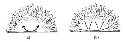
*Figure 5.16* Two scenarios that could account for mirror elongations along the surface from long flaws. (a) shows how a crack could unzip or propagate quickly along the surface. (b) shows that criticality could be reached at several points on the flaw periphery and fracture commences accordingly.
