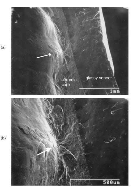
**Figure 10.31** SEM images of the origin. Notice all the wake hackle in the veneer aiming away from the interior. The crack ran from the inside to the outside. The inside surface is uneven and there are mold or tool marks in the vicinity. This region is directly opposite a region of extensive localized contact damage on the outer veneer surface.
