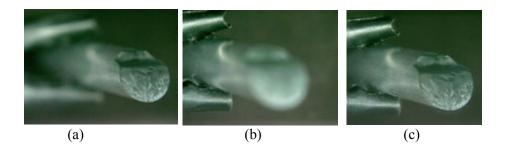
**Figure 3.12** A silicon nitride 6 mm diameter rod broken in flexure (801 MPa). (a) and (b) show stereoptical microscope digital images. Even though the microscope has great depth of field, the cantilever curl and holder are out of focus in (a). (b) shows the holder in focus. (c) shows the digitally reconstructed composite image from 15 separate images.
