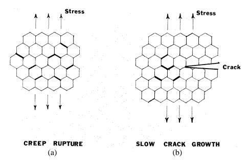
*Figure 5.62* Creep fracture and slow crack growth usually are intergranular at high temperature. In creep fracture (a), cavitation and microcrack nucleation occur throughout the body. In slow crack growth (b), the processes are confined to the crack tip region.
