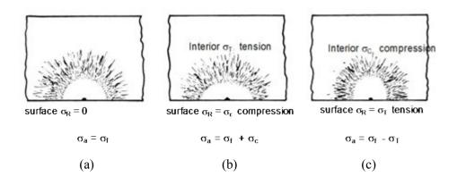
**Figure D.13** Surface residual stresses also may alter a mirror shape.  $\sigma_a$  is the applied stress to cause fracture and  $\sigma_f$  is the fracture stress in an annealed plate. (a) shows a surface mirror in an annealed plate. (b) shows the mirror shape in a plate with surface compression stresses that decrease into the interior and become tensile. (c) shows a mirror in a plate with surface tensile stresses that diminish into the interior and become compressive.
