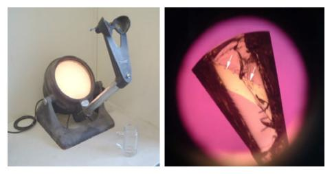
*Figure 3.59* (a) shows an old but still very useful polariscope. (b) shows a twin band (arrows) in a complex single crystal sapphire part. The photo was taken by a simple digital consumer camera held up to the eyepiece.
