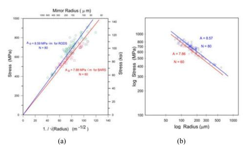
*Figure D-16 Fracture minor data for silicon nitride.*<sup>6,7</sup> *The round blue symbols are for 60 rods and the square red symbols are for 80 bars.*
