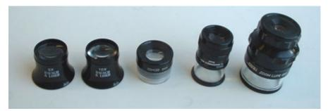
*Figure 3.2* Hand loupes and optical comparators. From the left, 5X and 7X watchmaker loupes; a 20X loupe, a 7X comparator with an internal 20 mm scale marked in 0.1 mm increments, and a 8X to 16X zoom comparator with an 16 mm scale marked in 0.1 mm increments.
