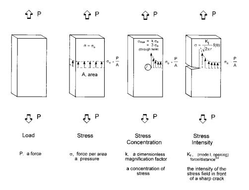
**Figure 7.12** A force P acts upon the object. Fracture occurs at a critical force that depends upon the material properties and the object's size. (b) stress is the force normalized by the cross sectional area. (c) discontinuities such as a thorough-hole <u>concentrate</u> stress and magnify it in the vicinity of the discontinuity. (d) sharp discontinuities such as cracks <u>intensify</u> the stress field in front of the discontinuity.
