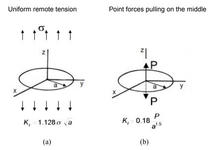
**Figure 7.17** The stress intensity  $K_1$  for penny-shaped circular cracks for two loading configurations. (The three-dimensional axes make the flaws appear elliptical in this view.) (a) shows a far-field tensile stress  $\sigma$ , and (b) shows opposed forces P pulling directly on the middle of the crack.  $K_1$  increases with crack size in (a), but decreases with crack size in case (b).
