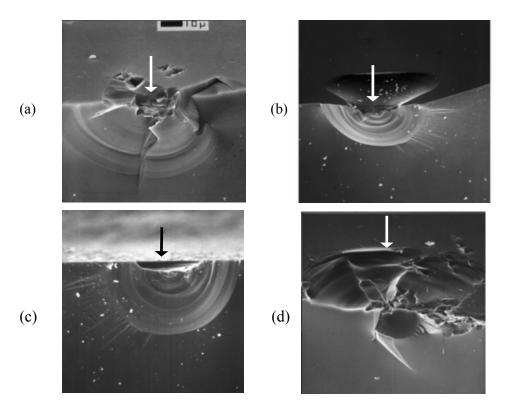
**Figure 6.30** Examles of sharp particle imact origin. in glass. The direction of impact is shown by the arrows. All of the impacts have created penetrating median – radial cracks. (b) and (d) have pronounced lateral cracks as well. In each case the impact site has been pulverized or crushed, unlike blunt impact sites.(a-d courtesy J. Varner).
