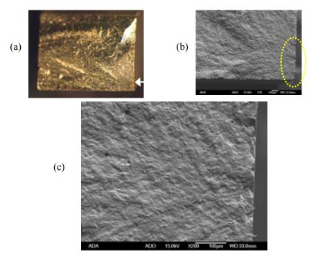
**Figure 6.46** Fracture surface of a feldspathic porcelain bend bar. (a) shows the entire surface of the 3 mm x 4 mm bar with a gold coating. The origin is on the right side wall (arrow). (b) and (c) show SEM images of the damage along the right side wall. Notice the slightly greater roughness of the fracture surface along the right side as compared to the fracture mirror centered on it.
