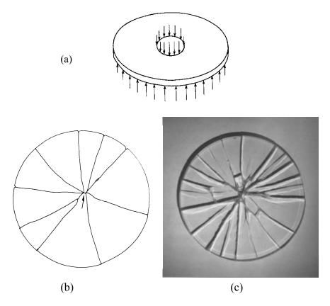
**Figure 4.2** Fracture patterns in a moderately-strong glass disk tested in ringon-ring biaxial strength test. (a) shows the test arrangement, (b) shows a schematic of a fracture pattern. The arrow marks the origin. (c) shows an example in a BK-7 borosilicate crown glass disk.
