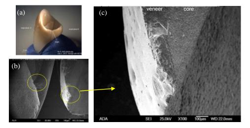
*Figure 10.33* Alumina incisor that broke in vivo at an unreported time. Fracture started at the margin from cracks and chipping in both the veneer and core. The crown split in half from the mesial to distal side. The margin is too thin and the core portion is exceptionally thin. (clinical case 8).
