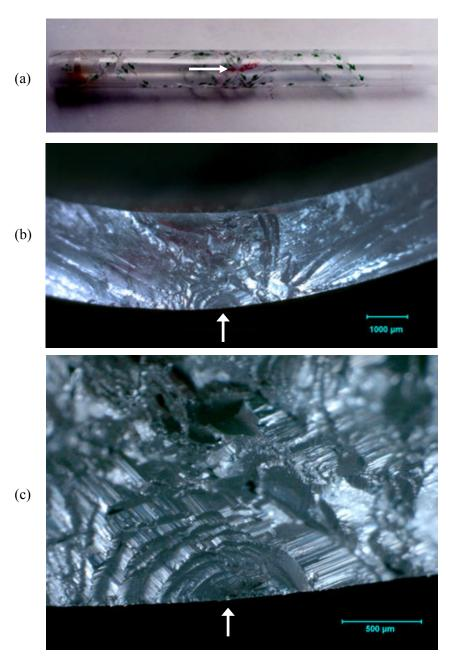
**Figure 8.26** Example of basal plane fracture in a c-axis sapphire tube that fractured from severe thermal shock (a). The origin is at the tube mid length (large arrow) and is perpendicular to the tube axis. The thermal stresses acted in the axial direction. (b) and (c) show the mirror and origin on the outer tube surface.
