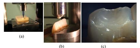
**Figure 4.27** Edge chipping. (a) shows the test machine with a 120° sharp diamond scriber making a chip in a dental stone material. (b) and (c) show a ceramic ball indenter chipping brittle denture material tooth specimens.
