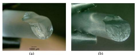
Figure 1.1 Fractured glass (a) and ceramic (b) rods.
