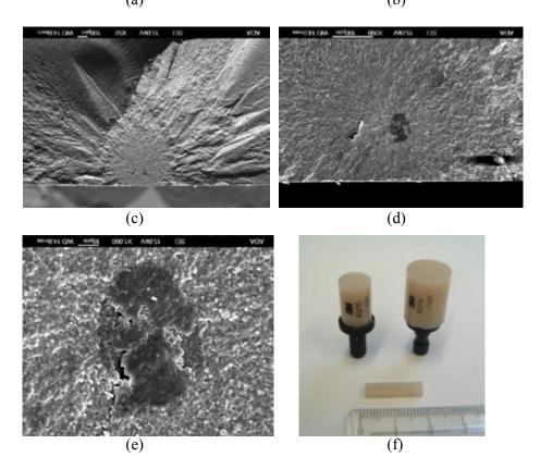
**Figure 9.6** Filled resin-matrix composite fractography. (a) shows the fracture mirror in an uncoated Paradigm MZ 100 bend bar, with transmitted light from under the bar, (b) shows the same view, but with reflected light after gold coating. (c) - (e) show SEM images of the mirror and the flaw, a calcium-rich inclusion. (f) shows the original blanks and a machined bend bar. (a-e courtesy J. Quinn)
