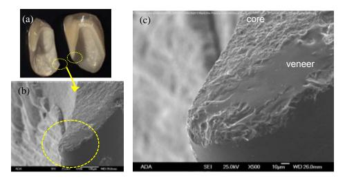
Figure 10.32 Alumina central incisor that broke in vivo after 1 year. Fracture started at the margin from cracking in both the veneer and core. The margin is too thin, and even worse, the core portion is exceptionally thin. The origin is chipping damage at the margin. (clinical case 2)
