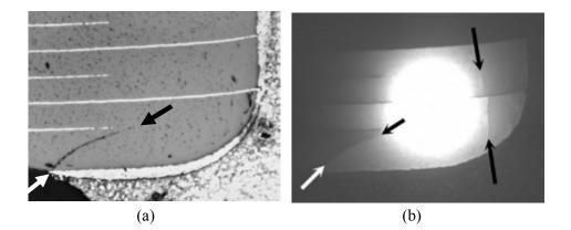
**Figure 3.20** Bright field reflected light (a) and vicinal illumination (b) of a multilayer ceramic capacitor. Both images are at the same magnification. Only one crack is apparent in (a). Vicinal illumination revealed the second crack on the right in (b). These are from a compound optical microscope. The aperture was stopped down for the image in (b). (Courtesy of S. Hull, NASA, Goddard Research Center.)
