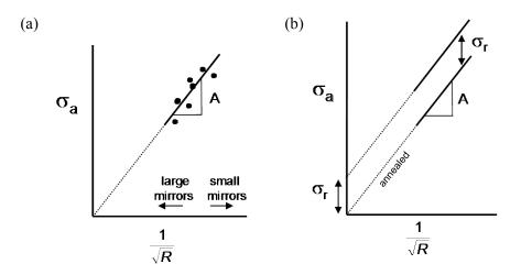
**Figure D.7** (duplicate ) Plot of applied stress,  $\sigma_a$ , versus  $1/\sqrt{R}$ , the preferred regression method. (a) shows the trend for parts with no residual stress. (b) shows the effects of residual stresses. Compressive residual stresses move the line up with a positive intercept  $\sigma_r$ , but with the same slope. Tensile residual stresses shift the data downwards.
