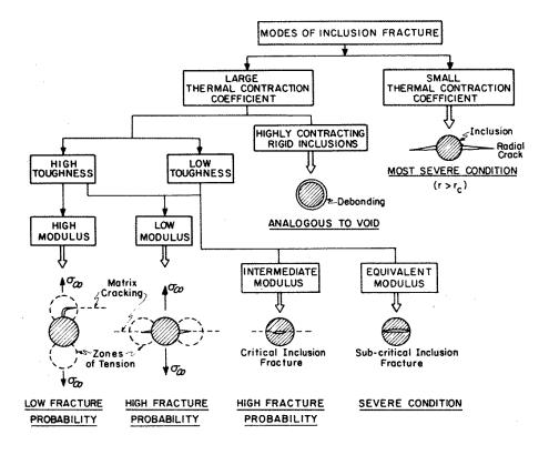
*Figure 6.18* The mismatch in properties between an inclusion and a matrix determine how severe an inclusion will be. From Evans, ref. 15.
