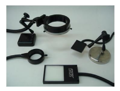
**Figure 3.16** Illumination sources for use with a stereomicroscope. Clockwise from the middle left: a ring light intended to be clamped to the objective lens, a ring dark light illuminator on an adjustable stand, a line light source on a stand, and a transmitted light platform.
