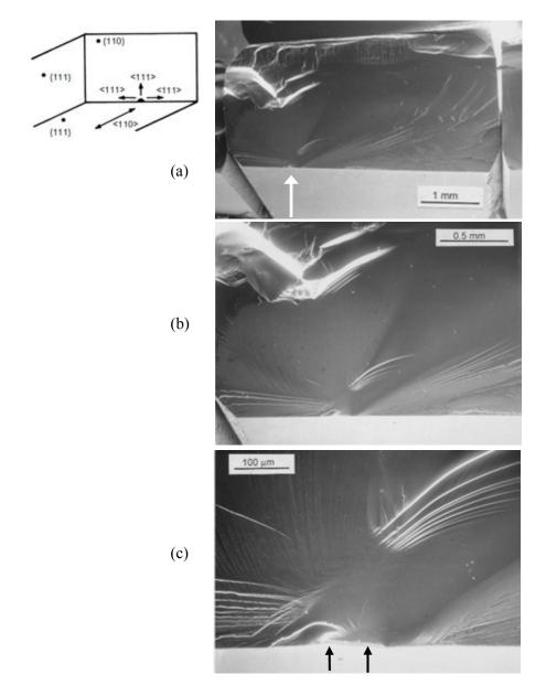
**Figure 8.14** Another example of a spinel bend bar with a {111} tensile surface and <110> tensile axis designed to cause fracture on a {110} plane. (261 MPa) (a) shows the whole fracture surface, (b) shows a "**skewed mirror**" with "**whisker lances**" and (c) shows the grinding crack fracture origin (black arrows) which is at a slight angle to the tensile stress axis and the fracture surface). (Case G2, table 8.2) (Courtesy R. Rice)
