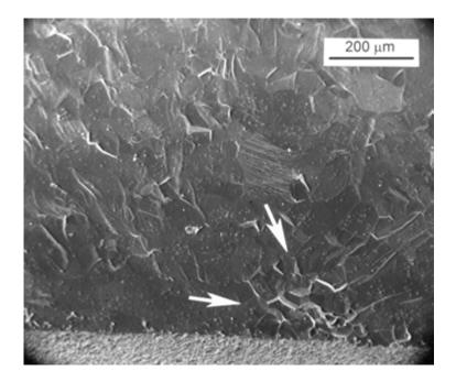
*Figure 5.58* Intergranular slow crack growth in a pure AlON at elevated temperature. The slow crack growth zone (arrows) formed in the short time that was needed to break the specimen in a strength test. (1200° C, 155 MPa, 22.5 ksi)
