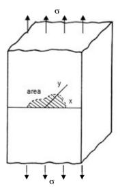
*Figure 7.25* An irregular planar shaped surface crack in a tension stress field. (After Murakami, ref. 50.)
