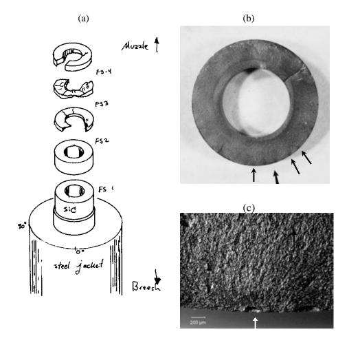
**Figure 10.8** Fractured  $\alpha$ -SiC gun barrel. (a) is a schematic sketch. (b) shows the fracture surface of one of the ring shaped fragments. Contact cracks are spaced periodically around the outer rim and appear as shadows in this view (arrows). The bore diameter is 12.7 mm. (c) shows a close-up of one of the contact cracks.
