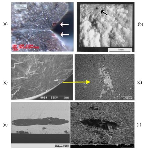
**Figure 6.16** Examples of inclusion origins. (a) is a red iron inclusion in sintered silicon nitride bend bar at an edge chamfer. (b) is an inclusion in a silicon nitride tension specimen. (c) and (d) are an iron inclusion in a silicon nitride. (e) is an alumina inclusion in a 3Y-TZP zirconia biaxial disk specimen (courtesy J. Eichler), and (f) is a vanadium inclusion in a binderless tungsten carbide bend bar. (courtesy J. Swab)
