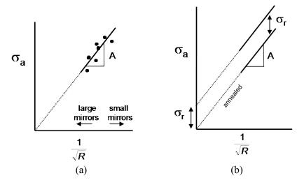
**Figure D.7** Plot of applied stress  $\sigma_a$  (at the origin) versus  $1/\sqrt{R}$ . (a) shows the trend for residual stress-free parts. (b) shows it for parts with residual stresses. Compressive residual stresses move the locus up with a positive intercept  $\sigma_r$ , but with the same slope. Tensile residual stresses shift the data downwards with a negative intercept (not shown).
