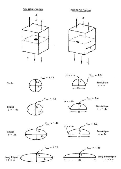
**Figure 7.19** The stress intensity shape factors Y for surface and internal round and elliptical for internal (volume) cracks and surface cracks for <u>far-field tension stresses</u>. Minimum Y factors for the surface cracks are shown in parenthesis. The Y factors for the surface flaws may also be used for parts loaded in bending if the flaw depth a is small relative to the specimen thickness (a/t is small).
