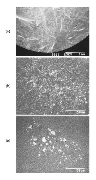
**Figure 3.44** A cluster of iron particles acting as an origin in a silicon nitride rod broken in flexure. The origin is below the surface. The stress at the origin was 682 MPa. (a) and (b) show secondary electron images and (c) is the backscattered image at the same magnification as (b).
