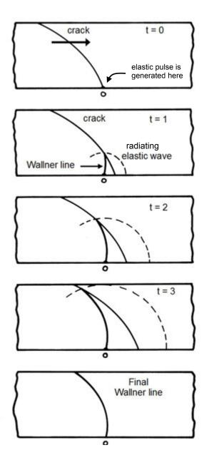
**Figure 5.37** Primary Wallner lines. This schematic series shows the progressive advance of the crack at successive time intervals. The elastic wave that forms the Wallner line (thick line) is generated when the advancing crack hits a surface irregularity "O". The crack leads on the bottom surface, but is moving at constant velocity in this example.
