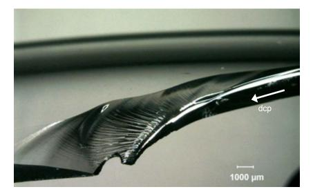
**Figure 5.32** Shear hackle in a glass plate. The crack was perpendicular to the glass surface and was slowing as it moved in the direction of the white arrow. It then turned 90° parallel to the surface and finally broke through to the surface at about 45°, producing the spectacular fan-shaped shear hackle. Shear hackle is a variant of twist hackle.
