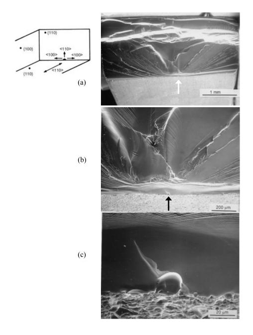
**Figure 8.12** Spinel bend bar with a {110} tensile surface and <110> tensile axis designed to cause fracture on a {110} plane. (361 MPa) (a) shows the whole fracture surface, (b) shows the "**gull wing mirror**," and (c) shows the grinding crack fracture origin. (Case C, table 8.2) (Courtesy R. Rice)
