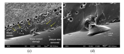
**Figure 6.74** A gold-coated lithium disilicate glass ceramic bridge pontic unit (courtesy S. Scherrer). It broke in vivo on the palatal side of a connector. The origin was a sharp contact damage crack in the vulnerable veneer. Notice the arrest lines marked by arrows in (c), the helpful wake hackle lines from the bubbles in the veneer seen in (c) and (d), and even the concentric tertiary Wallner lines typical of impact in (d). See also Figure 6.63.
