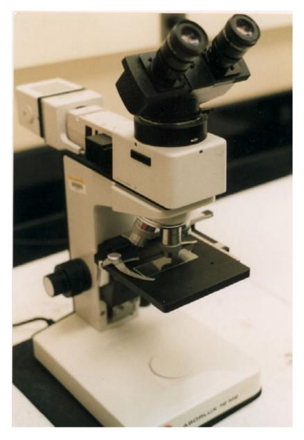
**Figure 3.29** Compound reflected light microscope. Although the microscope has twin eyepieces, they both view the same image collected by the objective lens. Overall magnifications can be as much as 1000X, but the working distances and the depths of field are very small. Only relatively flat specimens may be examined.
