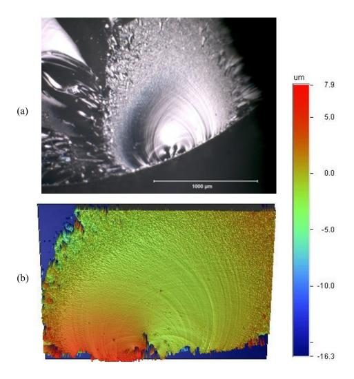
**Figure 3.50** Matching (a) optical microscope and (b) lateral scanning optical profilometer images of a fracture mirror in a ground glass rod. (b) shows an area 1.0 mm tall x 1.3 mm wide. The colors correspond to the scale range shown on the right (+7.9  $\mu$ m to -16.3  $\mu$ m). Wallner lines and mirror mist are readily detected and displayed. The origin is a surface crack from a scratch. (b is courtesy of R. Gates)
