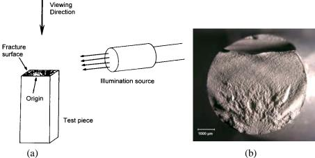
**Figure 3.18** Low-angle grazing illumination (a) is effective in highlighting fracture surface topography as shown in (b), which is the fracture surface of a ceramic rod broken in flexure.
