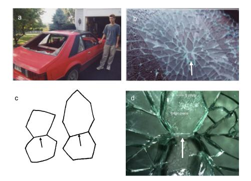
**Figure 4.18** Tempered glass fractures in the author's son's car. Flying debris from a tornado in College Park, Maryland in September, 2001 caused the impact fractures (a, b, d). The arrows show the actual origin in one window and (c) shows some variations of shape of typical matching origin pieces. The fracture surface of the origin piece is shown in Figure 5.19b
