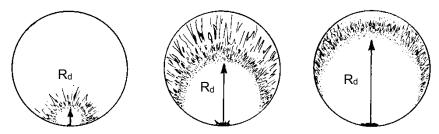
*Figure D.8 Mirrors surrounding surface origins in rods or fibers loaded in direct tension. (after Ref. 17) Measure both the mirror-mist radius (shown) and mist hackle radii into the depth as shown.*
