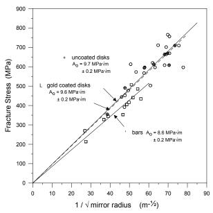
**Figure 7.11** Fracture mirror size data for a 3 mol % yttria-stabilized tetragonal zirconia (3Y-TZP) from Ref. 35. Figure 7.8 shows one of the mirrors. Figure 3.24 shows a mirror both coated and uncoated. Bend bars produced a smaller mirror constant, either due to a geometric effect or simply the scatter in the data.
