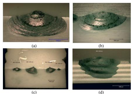
**Figure 4.28** Edge chips formed in (a) dental lithium disilicate glass ceramic; (b) dental 3Y-TZP zirconia; (c) dense alumina; and (d) laminated alumina/alumina-zirconia ceramic. The chips were stained with a green felt tip pen to make the fracture surfaces easier to see in these translucent materials.
