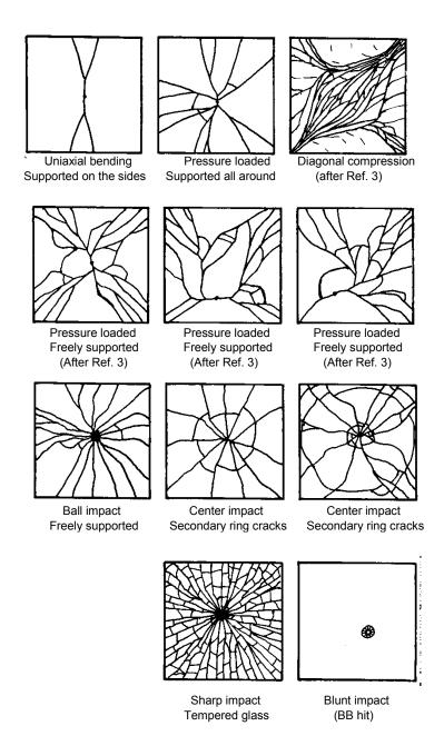
*Figure 4.17 Plate and window fracture patterns. Figure 4.14b shows an example of a center impact plate with secondary ring cracks*
