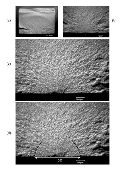
**Figure D.3** Silicon nitride bend bar with a Knoop surface crack (449 MPa, Ceralloy 147-31N, Refs. 6,7). The mirror is incomplete into the stress gradient, but the mirror sides can be used to construct boundary arcs in (d). Radii are measured in the direction of constant stress along the bottom.
