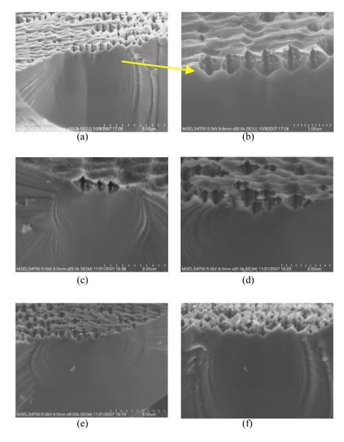
*Figure 8.21* Fracture origins in single crystal silicon theta specimens. (b) is a close-up of (a). The "cathedral mirrors" are very clear. The origins are etch pits from the DRIE processing. The cusps between them are very sharp and probably initiated cracks. Figure 6.69 shows other sharp cusp origins.
