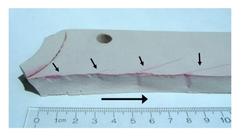
*Figure 3.54* Fractured porcelain part with dye penetration by a common felttip pen. The dye reveals crack branching patterns (small arrows) and thus the direction of crack propagation (large arrow).
