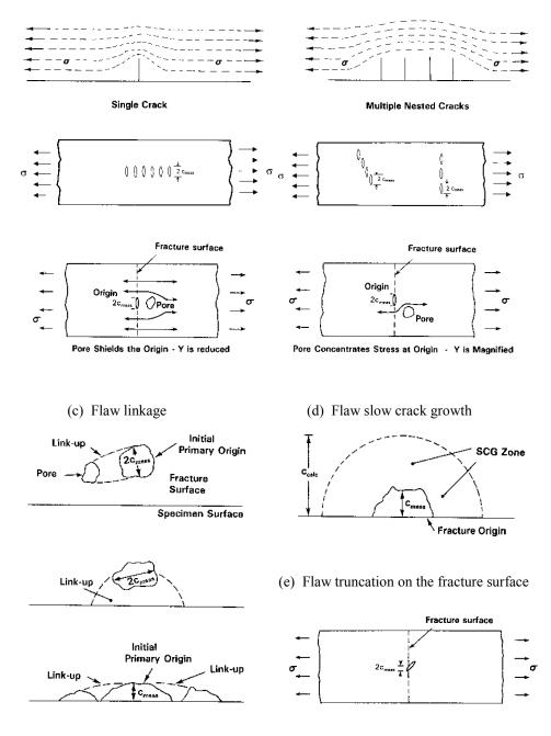
*Figure 7.27 continued* Factors that cause calculated and measured crack sizes to differ.
