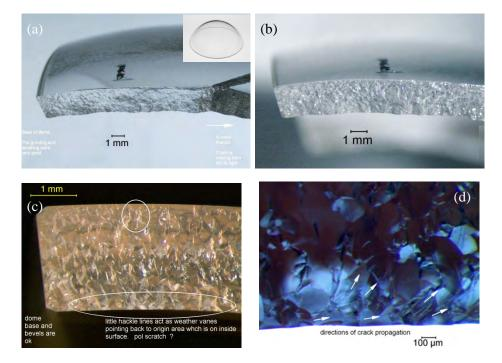
*Figure 10.14.* AlON infrared missile dome. (a) shows how the branch on the right leads away from the origin area. (b) shows the fracture surface with the coarse microstructure.
