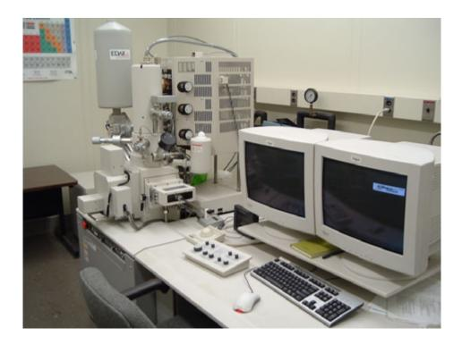
Figure 3.49 A field emission scanning electron microscope
