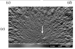
**Figure 6.19** Examples of inclusion origins in a highly-filled resin-matrix dental composite (Paradigm MZ 100) (a) and (b) show a calcium rich inclusion. (c) – (e) show the same aluminum inclusion with: transillumination (c), conventional reflected light (d), and in the SEM (e).
