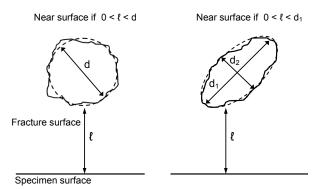
**Figure 6.2** Near surface (NS) origins are no deeper (l) than the flaw diameter or major axis length.
