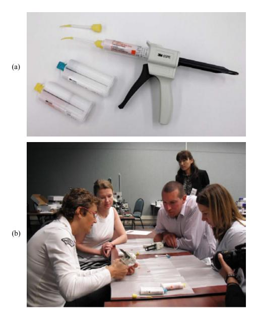
*Figure 3.33* Dental replica equipment. (a) shows a typical PVS applicator gun which has interchangeable tips and compounds. (b) shows Dr. S. Scherrer demonstrating the technique in a dental materials fractography class.
