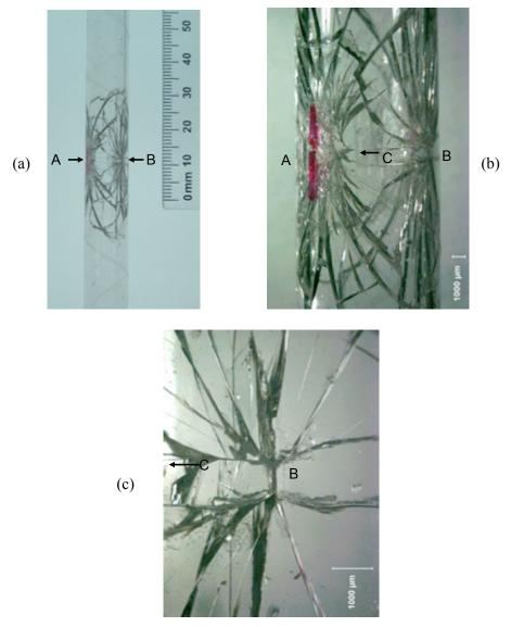
**Figure 4.22** Small glass tube loaded diametrally at opposing points A (only the front is shown). Fracture started at the side hinge point B which generated an array of radiating cracks. One of these is the "leader crack" C (arrows in b and c) which went to the loading site A where it branched repeatedly and fanned out yet again. (Tube courtesy of W. Haller.)
