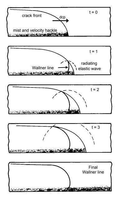
**Figure 5.40** Secondary Wallner lines are formed by the crack itself. This schematic series shows the progressive advance of the crack and the elastic pulse that forms the secondary Wallner line (dark line) in a plate with a stress gradient. Notice the hook final shape, a consequence of the stress gradient caused by the variation in the crack velocity from a maximum on the bottom to close to zero at the top.
