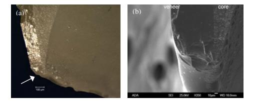
**Figure 10.34** Alumina molar #37 that broke in vivo at 7 months in vivo. It split in half from the mesial to distal side. Fracture started at the margin from cracks and chipping in the veneer which extends to the very tip and even onto the inside surface as evident in (a) Notice the tiny wake hackle lines in the veneer in (a) that show the origin was at the margin. (a) also shows chipping elsewhere on the margin. (clinical case 9).
