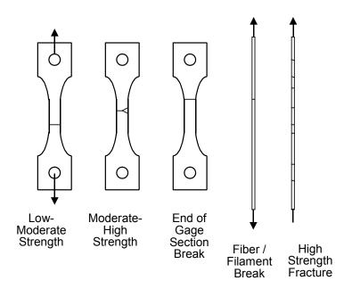
Figure 4.7 Tension specimen and fiber fractures.
