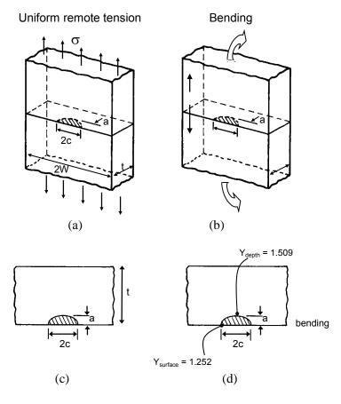
**Figure 7.18** Surface cracks in plates or bars in far-field tension (a) or bending (b). The stress intensity factor equations by Newman and Raju<sup>40</sup> are applicable to these configurations. The Y factors for case (a) and (b) are the same for very shallow cracks,  $a/t \rightarrow 0$ . (c) is a view of the cross section. (d) shows the same but labeled with the Y factors at two locations for the flaw dimensions given in the example on page 7-31 in Section 7.5.2.1.
