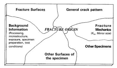
*Figure 1.4. Fractographic analysis is more than examining fracture surfaces.*<sup>5</sup>
