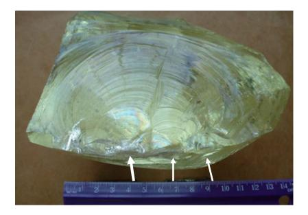
**Figure 5.42** Tertiary Wallner lines in a large chunk of glass that was hammered into pieces. There are multiple impact sites marked by arrows, the most prominent of which is marked by the larger white arrow. Notice how the tertiary Wallner lines are concentric about the impact sites. This was one of Professor Fréchette's demonstration pieces.
