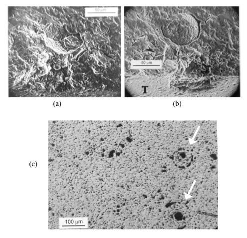
**Figure 6.4** Fracture origin in a sintered alpha silicon carbide flexure specimen. (a) suggests the origin is a pore, but (b), which shows the mating half, shows it is an agglomerate. (c) shows a polished microstructural section for this material that reveals the agglomerates (arrows).
