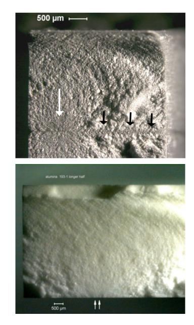
**Figure 6.38 (cont'd)** Examples of parallel grinding cracks. (f) shows back-toback halves of a silicon nitride bend bar with coarse grinding (150 grit) cracks. A zipper crack is at the origin (large white arrow). The small black arrows show that there also is a machining crack "skin zone" along the entire surface. (g) is an alumina bend bar with low-angle grazing illumination from the side revealing a zipper crack.
