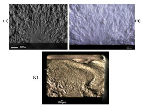
**Figure 5.8** Fracture mirrors in ceramics. (a) is a SEM image of a strong bend bar (1024 MPa) of Y-tetragonal zirconia polycrystal (Y-TZP) for dental crowns. (courtesy J. Quinn) (b) is a stereoptical microscope of another Y-TZP bend bar (486 MPa) for an engine application. (c) is a stereoptical image of a silicon nitride bend bar (487 MPa).
