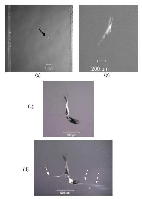
**Figure 6.57** Chill check cracks on the outer surface of unbroken glass plates. (a) and (b) show the same chill check. (c) and (d) show two close-up views of another chill check. Note how different illumination can dramatically alter the appearance and apparent extent of the flaw. Much more of the cracking is evident in (d). (Specimens courtesy V. Fréchette and J. Varner)
