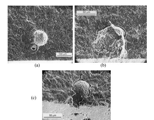
**Figure 6.14** Examples of agglomerate fracture origins. (a - c) show spray dry agglomerate fracture origins in sintered alpha silicon carbide. Agglomerates often sinter away from the matrix leaving a void-like crack.
