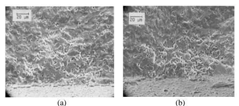
**Figure 10.11** Fracture origins in 1200 °C  $\alpha$ -SiC specimens that fractured at 863 h (a) and 1460 h (b) from surface-connected porous regions.
