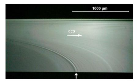
*Figure 5.36 Primary Wallner line in a glass slide broken in bending. A simple scratch on the surface (arrow) triggered the strong Wallner line as the crack ran from left to right. Other tiny faults triggered fainter primary Wallner lines.*
