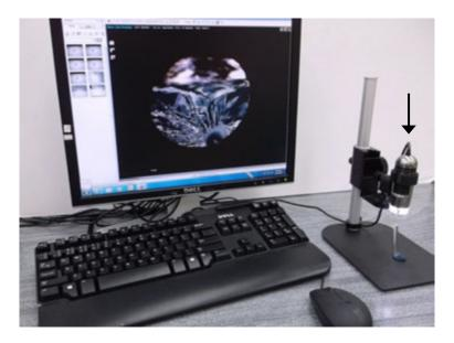
**Figure 3.15** Digital microscopes are a new tool for the fractographer. This simple digital microscope (arrow) is mounted in a stand on the right. It is focused on the fracture surface of a broken glass rod. The monitor and computer (not shown) are separate components
