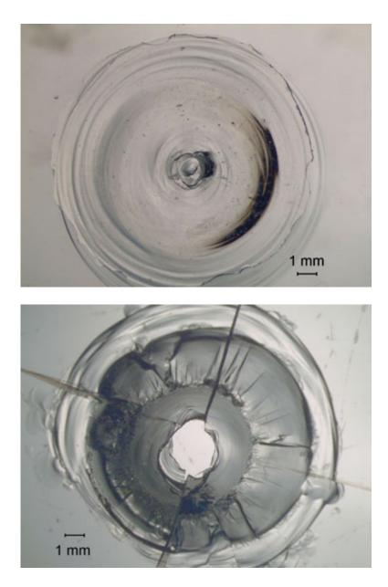
**Figure 6.34** Blunt impact origins in glass plates. (a) shows a mild – moderate impact with cone cracks. The plate did not break into pieces. (b) is a severe impact that was sufficient to create cone and radial cracks. The latter caused plate fracture. (Specimens courtesy of J. Varner and V. Fréchette, Alfred University)
