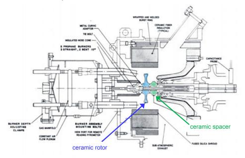
Figure 10.2 The Ford hot spin test rig (Ref. 2).
