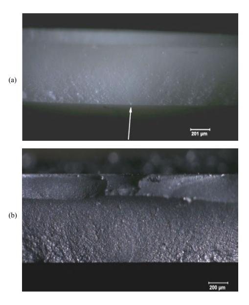
*Figure 3.24* Two views of a fractured yttria-stabilized tetragonal zirconia disk with reflected light illumination. (a) shows the uncoated fracture surface and (b), the same region after a thin gold coating was applied.
