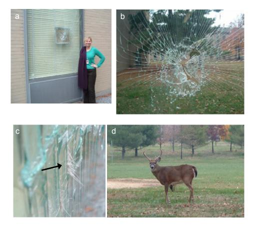
**Figure 4.14** Dr. J. Quinn with a window fracture problem at NIST. Evidence collected at the scene included foreign material attached to the impact site as shown in (c). The crack patterns indicated impact from the exterior. That, plus the height of the impact above the ground, the tuft of fur, the time of the year (November, the rutting season) and similar occurrences elsewhere suggested the cause of failure shown in (d). The deer saw its reflection in the window and attacked it!
