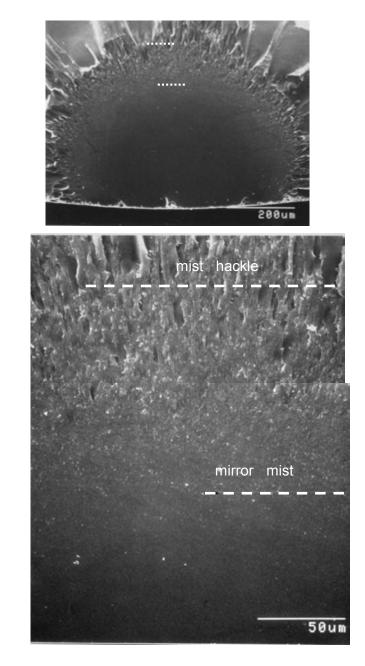
**Figure D.1 continued** (c) is an SEM image of the same mirror and at the same magnification as (a) and (b). The mist is indistinct in the SEM image. (d) is a composite of two SEM images showing the transition from mirror to mist to hackle. The locations of the boundaries as assessed by <u>optical</u> microscopy (as shown in (b))are marked by dashed lines on the SEM images.
