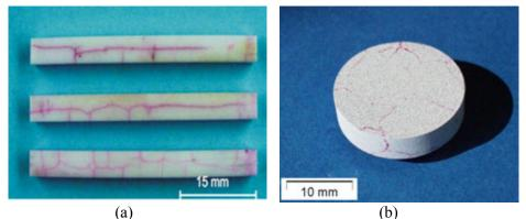
**Figure 4.30** Thermal shock cooldown cracks in alumina bend bars (a), and a disk (b). The cracks are highlighted by red dye penetrant. (courtesy of R. Danzer and T. Lube, Mountain Univ. Leoben)
