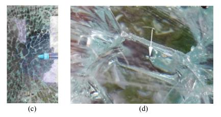
*Figure 3.10* Cell phones can be used for fractographic analysis (a) shows an obsidian arrowhead as viewed at 2X magnification in a cell phone; (b) a street photo near Santo Stefano Basilica in Bologna, Italy in 2014; (c) a close-up of the tempered glass fracture pattern, and (d) the close-up at 5X of the internal inclusion origin (arrow). The author was on his hands and knees for (d), which was shot at 5X about 60 mm above and aiming through the glass at an angle.
