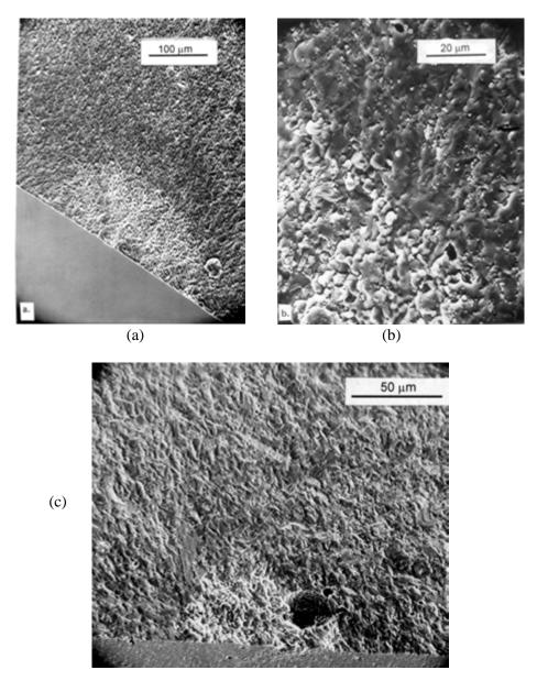
**Figure 5.59** Elevated-temperature slow crack growth in sintered alpha SiC tested in stress rupture at 1400 °C in air (a). The close-up (b) shows the boundary between the intergranular SCG and the transgranular fast fracture zones. (c) shows another alpha SiC specimen wherein the slow crack growth appears to have originated near a pore.
