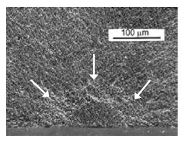
**Figure 5.57** Knoop flaw (dark semiellipse) in silicon nitride showing stable crack extension (white arrows). The local residual stresses underneath the indentation provided the impetus for the extension. Traces of the very shallow, elongated Knoop indentation can be seen on the bottom surface.
