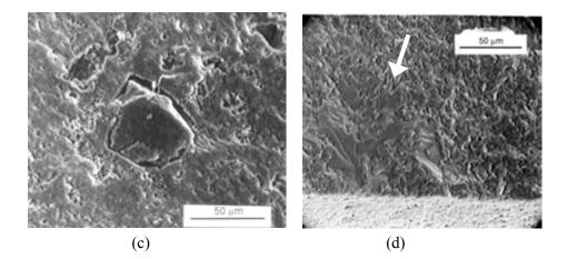
**Figure 6.20** Examples of compositional inhomogeneity fracture origins. (a) and (b) show an example of an aluminum rich zone in a hot-pressed silicon carbide. Aluminum is an element in the sintering aid. (c) shows an unreacted silicon globule that pulled away from the matrix in a reaction-bonded silicon nitride. (d) shows a silicon lake in a siliconized silicon carbide.
