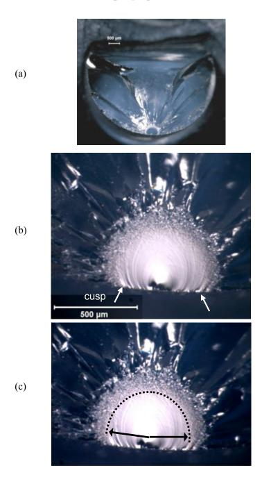
**Figure D.12** Fracture mirror in a fused silica rod (a), illustrating the cusps in the mirror near the outer surface (b). Mirror measurements should not include the inward bend of the mirror and may be made as shown in (c).
