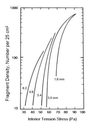
*Figure 7.4* The interior tension stress in tempered soda lime glass plates may be estimated from the fragment density when the plate is broken. Each line corresponds to the plate thickness shown. (After Akeyoshi et al., Ref. 11)
