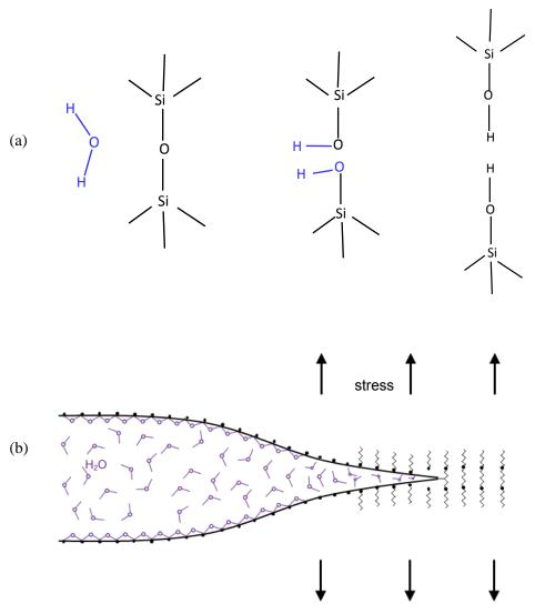
**Figure 5.54** Stress corrosion cracking can cause slow crack growth in glasses. The polar water molecule, either in liquid or gaseous form, attacks strained silicate bonds. (after Michalske and Freiman<sup>50</sup> and Michalske, Bunker, and Freiman<sup>51</sup>)
