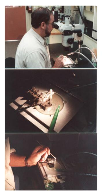
**Figure 3.25** A simple but effective coating technique for white ceramics is to stain the surface with a green felt tip pen. The staining can be watched in real time through the microscope. The green stain can be easily removed with ethanol alcohol on a cotton swab applicator and the process repeated.
