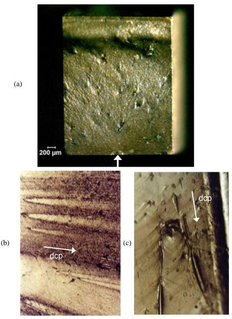
**Figure 5.26** Wake hackle (a) shows wake hackle from inclusions in a lead zirconium titanate bend bar. They point back to the origin on the bottom. The tensile surface is on the bottom and a compression curl is on the top. The origin is a semielliptical surface crack (arrow) generated by a Knoop indentation. (b) and (c) show parabolic double wake hackle tails triggered by inclusions in obsidian glass. (b,c courtesy A. Tsirk)
