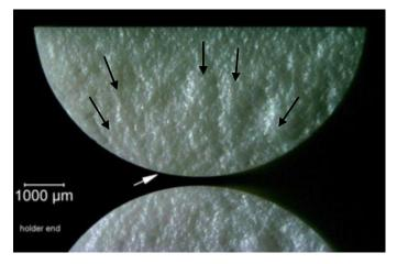
**Figure 5.22** Coarse microstructural hackle. Matching fracture surface halves of a split cylinder flexural strength specimen of a coarse-grained (50 µm to 80 µm) Mg partially-stabilized zirconia. It has a very rough clumpy fracture surface. Low-angle grazing illumination shows the coarse hackle lines (black arrows) radiating from the origin region (white arrow).
