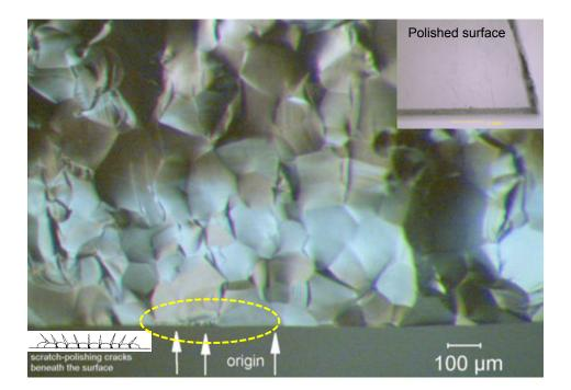
**Figure 10.15** Wake and twist hackle within cleaved AlON grains lead back to the inside surface and to tiny zipper machining crack hackle lines within one or two large grains. This image was taken at the maximum magnification (125X) of the stereoptical microscope that was used for the examination. The insert shows the outer polished surface with polishing scratches and a well-ground bevel-chamfer.
