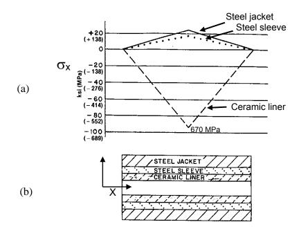
**Figure 10.7** Axial stress distribution,  $\sigma_x$ , as a function of position x in the assembly along the bore (a). The stresses correspond to the three parts shown in a sectional view in (b) which is a simplified version of the assembly shown in the previous figure. The stresses included those from shrink fitting and projectile firing. (Figure from Ref. 6)
