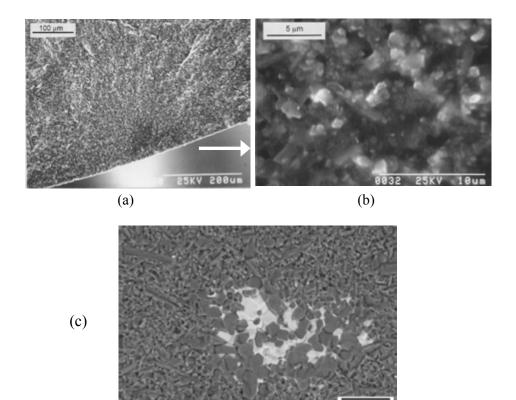
**Figure 6.21** Examples of compositional inhomogeneity fracture origins. (a) and (b) are an example of a local excess of sintering aid in a sintered reactionbonded silicon nitride. (c) is a yttria-alumina agglomerate in a silicon nitride bend bar. (c is courtesy T. Lube and R. Danzer)
