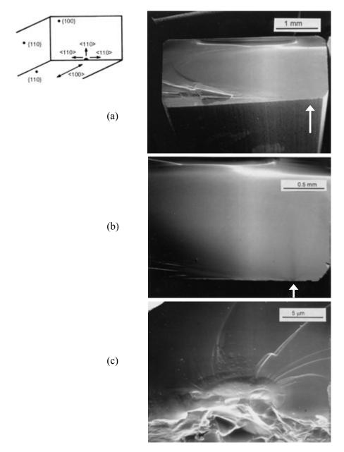
**Figure 8.8** Spinel bend bar with a {110} tensile surface and <100> tensile axis designed to cause fracture on the {100} cleavage plane. (170 MPa) (a) shows the whole fracture surface which is flat except for the cleavage steps on the side and the cantilever curl. Other similar specimens had no cleavage steps. (b) shows the origin site and (c) shows the grinding crack fracture origin. (Case D, Table 8.2) (Courtesy R. Rice)
