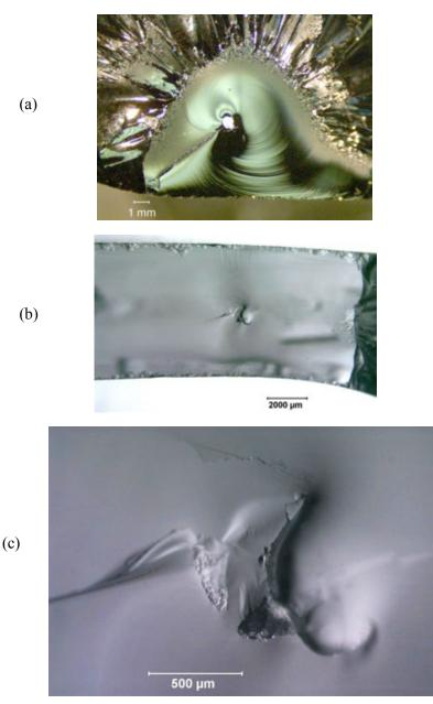
**Figure 6.55** Stone origins exposed on glass fracture surfaces. (a) is an example in a large-screen television picture tube and broke from transient thermal stress during manufacture. (specimen courtesy of J. Varner and V. Fréchette). (b) and (c) show a stone in the middle of the wall of a heat-strengthened consumer glassware.
