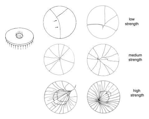
**Figure 4.12** Fragmentation patterns in ring-on-ring loaded specimens. The small arrows mark likely origin areas. In low strength parts, after the first break has occurred, the larger remnant may still bear load from the inner loading ring, and it in turn will break in bending. In moderate to high strength disks, secondary circumferential cracking occurs near the inner loading ring.
