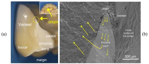
**Figure 6.73** Glaze interfaces can be preferred sites of fracture initiation. This is an in vivo broken six-unit zirconia bridge with a poor design. The origin is the pore cluster at the interface between the veneer and core apex. (images courtesy U. Lohbauer and S. Scherrer)
