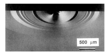
*Figure 5.66* Concentric <u>arrest lines</u> in a plate of soda lime silica that was cyclically loaded in flexure. The lines are due to slight variations in the crack growth planes on each loading cycle. (courtesy of D. Green, Penn State University, same as Figure 5.47c)
