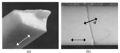
**Figure 4.11** A twisted fracture surface in a misaligned alumina bend bar in a fixture that did not articulate properly. (a) shows the fracture surface, and (b) the tensile surface of both halves. The principal stress direction (solid black arrow) was 14 degrees off the expected direction (dotted arrows). Twisted or angled fracture planes should prompt the tester to check the fixture articulation and specimen alignment procedures.
