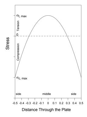
Figure 5.19 Residual stresses in thermally-tempered glass pieces.
