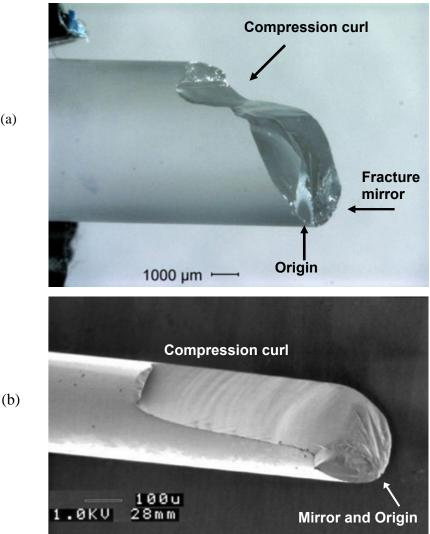
*Figure 5.1 Classic fracture patterns. (a) shows* a low-power stereoptical microscope image of a *fused silica rod fractured in bending at 88.5 MPa (12.8*) ksi) (b) shows an SEM image of a chalcogenide fiber fractured in bending at 368 MPa (53.4 ksi). (b is courtesy of J. Quinn and V. Nguyen)
