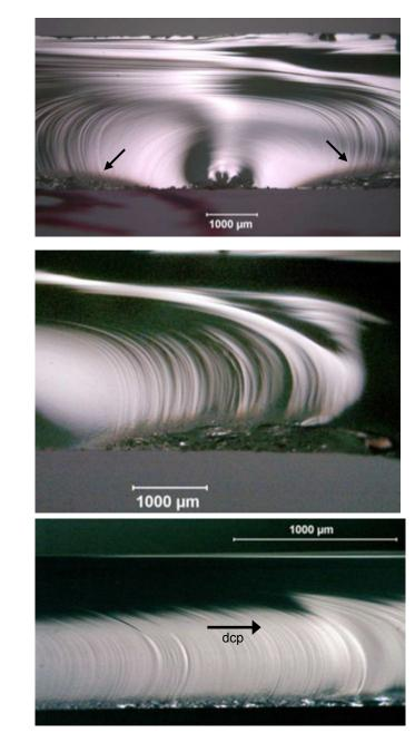
**Figure 5.41** Examples of secondary Wallner lines in glass microscope slides. (a) and (b) show Wallner lines from the sides of a mirror. (b) is a close-up of the right side of (a). Mist and hackle triggered the secondary Wallner lines. There also are fainter primary Wallner lines inside the mirror. Notice their different arcs. (c) is a slide broken in bending.
