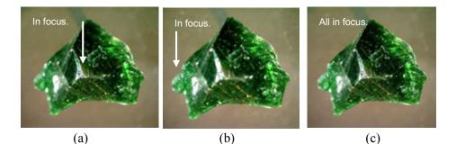
**Figure 3.13** A 25 mm glass fragment. (a) and (b) show typical images made by a stereoptical microscope at low magnification. Although the microscope has excellent depth of field, portions of the fragment are out of focus in each view. (c) shows the digitally reconstructed image made from 16 separate images focused from the top to bottom of the fragment. The digital reconstruction took less than 1 minute.
