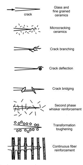
Figure 7.16 Crack interactions with microstructure.
