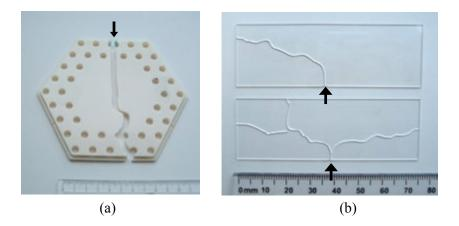
**Figure 4.20** Thermal fractures with origin marked by arrows. (a) shows an alumina furnace baffle plate. Fracture started from grinding cracks associated with a hole. (b) shows glass slides broken by simply heating them on a hot plate.
