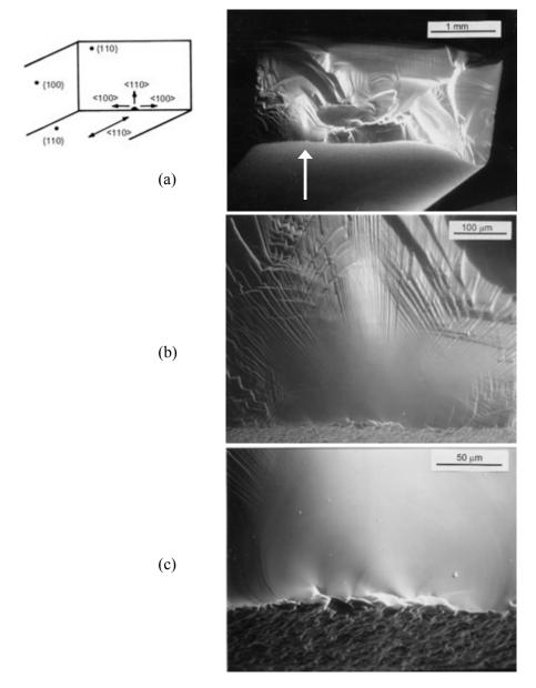
**Figure 8.11** A second example of a spinel bend bar with a {110} tensile surface and <110> tensile axis. (172 MPa) The fracture surface (a) is very rough as in the previous figure. The mirror (b) is somewhat more symmetric than in the previous figure. This mirror was shown in an earlier publication (Figure 29 of Ref. 13), but with a typographical mistake identifying it as {110}<100>. (Case F2, table 8.2). (Courtesy R. Rice)
