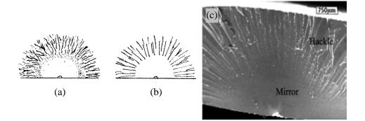
**Figure 5.7** Mixed-mode loading creates fracture mirrors without mist but with a systematic array of "lance hackle." (a) shows a normal mirror from pure opening mode I loading. (b) and (c) show mirrors from mixed opening/shear modes I/II, (c is courtesy J. Mecholsky).
