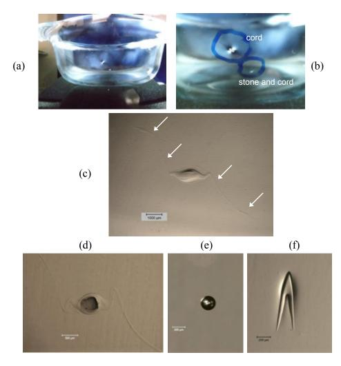
**Figure 6.56** Flaws in a borosilicate glass cookware. (a) – (c) show a <u>chord</u>. (crossed polarizers highlighted the internal strains in views (a) and (b). (c) is a close-up of the cord with a mix of transmitted and reflected illumination. The striae - stringers are marked by arrows. (d) shows a close-up of a <u>stone</u> with striae - stringers. (e) is a <u>seed</u> (a bubble). (f) is an odd internal hairpin flaw.
