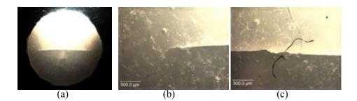
**Figure 3.19** Vicinal illumination of a PEG dental resin with amorphous calcium phosphate filler. The disk specimen (a) broke in a biaxial strength test, but there was insufficient stored elastic energy to fully break the specimen. (b) is a close-up of one crack tip, and (c) is a close-up of the tensile surface at the fracture origin. The flaw is a trapped hair or fiber. This was confirmed by examination of the fracture surfaces once the specimen was snapped in half by hand.
