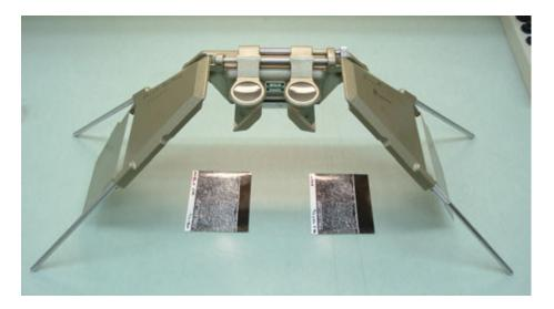
*Figure 3.48* Stereoscope. The two photos are placed under the viewer and the viewer looks into the two eyepieces. The photos are moved around slightly until they appear as one image in three dimensions.
