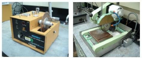
Figure 3.61 Wafering and cut off wheel machines.
