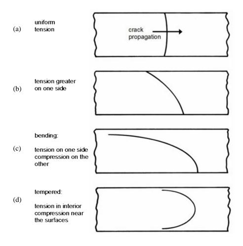
**Figure 5.35** Crack front variations due to stress distributions through the thickness. (a) shows a crack front in a uniform tensile loaded plate. (b) a plate with greater tensile stress on the bottom. (c) a plate in bending such that the bottom is in tension and the top in compression. (d) a tempered plate with tensile stresses in the interior and compressive stresses at the surface.
