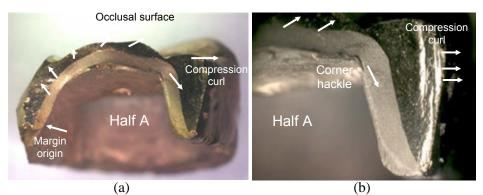
**Figure 10.25** Procera alumina molar crown. The crown split vertically into two halves. The fracture surfaces have been gold coated. (b) is a close-up of the compression curl on the side away from the origin site. The veneer glass is dark and the core ceramic is a lighter shade. The arrows show the dcp from: corner hackle around the inside corner, the compression curl, and from veneer wake hackle. (c) – (g) are on the next page.
