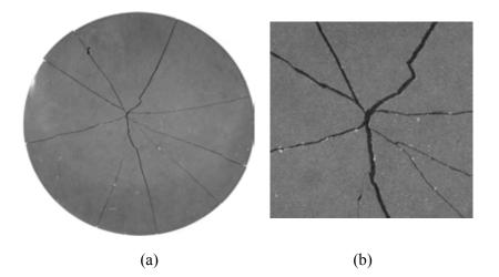
**Figure 4.6** Fracture pattern in a 44.5 mm silicon nitride ring-on-ring (10 mm x 40 mm) equibiaxial strength test disk. The stress at fracture in the inner ring was 447 MPa. The branching is curved near the origin. Successive secondary branching occurs over short distances. (b) is a close up of the origin area showing that the initial branch angles are 140° and 145°. Additional branching is minimized as the crack propagated into lower stress areas away from the disk center.
