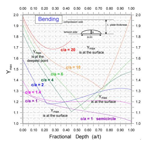
**Figure 7.23** The maximum stress intensity shape factor Y for semielliptical surface cracks in a bending stress field in a plate or bar of thickness t. In the limit as the flaw is very small relative to the plate thickness,  $a/t \rightarrow 0$ , the solutions are the same as for the uniform tension case. The kink in the loci corresponds to where the maximum Y changes from the surface to the deepest point in the interior or vice versa.
