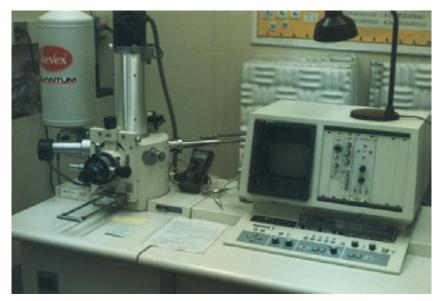
Figure 3.36 A conventional scanning electron microscope.
