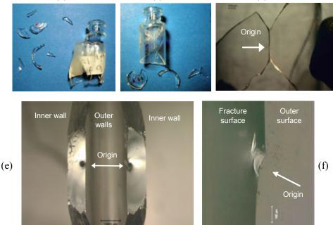
**Figure 4.23** Pressurized thin-walled vessels. (a) shows that the side walls are stressed in biaxial tension. Hoop stress is double the axial stress and therefore the first fracture is usually vertical as shown in the medicinal vial shown in (b)–(f). (e) shows the matching fracture surfaces at the origin. There is a distinct fracture mirror centered on the origin. (f) shows the origin was an arc shaped crack in the outer wall, a clear indication of blunt contact damage.
