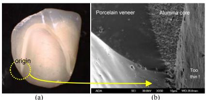
**Figure 6.70** A "feather tip" margin in an alumina dental crown that broke in a patient's mouth ("clinical 22"). The margin is only 30  $\mu$ m wide and was extremely vulnerable! Hoop stresses caused fracture from some of the tiny flaws at the margin tip. (crown courtesy of M. Øilo)
