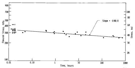
**Figure 10.10** Stress rupture curve at 1200 °C in air for sintered  $\alpha$ -SiC.<sup>7-9</sup> Every time-dependent fracture was from a pore or porous zone and only if it was surface connected. The hollow points with arrows to the left are breaks on loading and are consistent with the fast fracture strength which was about 350 MPa. The slow crack growth exponent N was 40.8.
