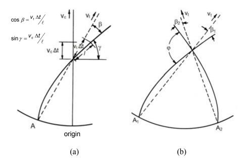
**Figure 7.30** Analysis of Wallner lines to determine the crack velocity if a crack radiates outwards from an origin. (a) shows a case where the location of the Wallner line elastic wave pulse (site A) and the direction of the crack extension are known. (b) shows the case where the precise crack growth direction is not known, but the origins ( $A_1$  and  $A_2$ ) of the Wallner lines are known.
