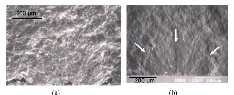
**Figure 3.42** Comparative secondary electron (a) and backscattered electron (b) images of the fracture surface of a Knoop semi-elliptical precrack in a silicon nitride fracture toughness test specimen. The edge charging in (a) emphasizes certain features, but (b) shows that the flattening effect of the backscattering mode tends to better reveal the overall crack (arrows).
