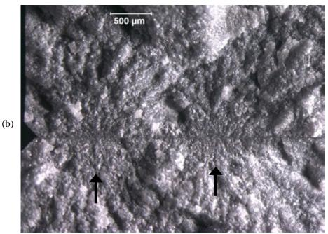
*Figure 5.11* Multiple mirrors from grinding damage in a silicon nitride bend bar. (b) is a close-up of (a). Grinding damage caused fracture in these examples and the origins in each mirror were nearly identical. (*Ref. 35*)
