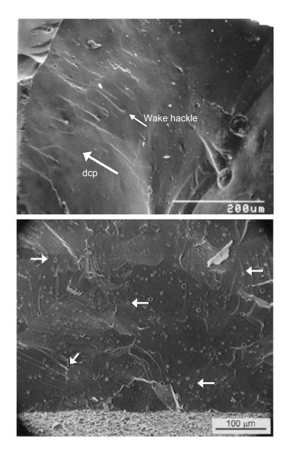
**Figure 5.25** Wake hackle. (a) shows an array of wake hackle from pores in an Empress II dental crown veneer. The direction of crack propagation is marked by the arrow. Notice that some hackle is triggered even though the crack did not cleave the pore (small white arrow). (b) shows an example of transgranular fracture from a large grain origin in polycrystalline AlON. Wake hackle was triggered by grain boundaries and tiny pores (small arrows).
