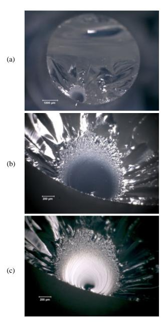
**Figure 5.2** Three views of a fracture mirror in fused silica glass rod broken in bending at a high stress level (96.2 MPa, 13.9 ksi). (a) shows the entire fracture surface. (b) is a close-up of the mirror, and (c) is the same region but with the illumination adjusted. Maximum tension was at bottom center in view (a). The mirror is asymmetric due to the bending stress field.
