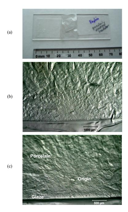
**Figure 3.32** Cellulose acetate replica of a fracture surface of a porcelain electrical insulator. (a) shows the replica taped to a glass microscope slide. (b) and (c) show close-ups of the replica which reveals the fracture mirror and an inclusion flaw.
