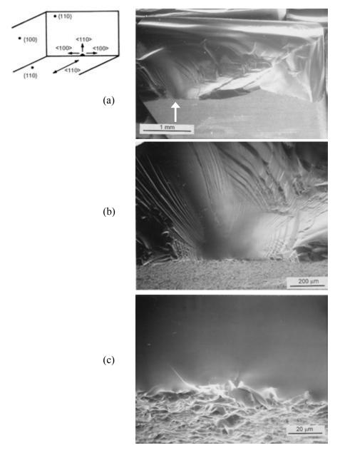
**Figure 8.10** Spinel bend bar with a {110} tensile surface and <110> tensile axis designed to cause fracture on a {110} plane. (283 MPa) (a) shows the whole fracture surface, (b) shows the mirror with "whisker lances" radiating outward, and (c) shows the grinding crack fracture origin. (Case F1, table 8.2) (Courtesy R. Rice)
