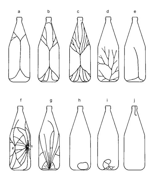
**Figure 4.21** Bottle fracture patterns. (a-c) sidewall fractures due to internal pressure at progressively greater pressures; (d) internal pressure fracture starting from the base; (e) is a thermal fracture from sudden cooling of the base; (f) is an impact fracture on the right side (labeled 1) with a hinge fracture on the side (labeled 2); (g-i) show water hammer fractures and (j) shows a fracture from diametral rim clamping.
