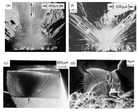
**Figure 8.1** Examples of single crystal fractures. (a) and (b) show fracture mirrors on the  $\{100\}$  type planes in MgO, but with two different tensile surface orientations. (c) and (d) show a cubic zirconia bend bar with curved linear lance like markings emanating from the origin area and the grinding crack origin. (courtesy R. Rice)
