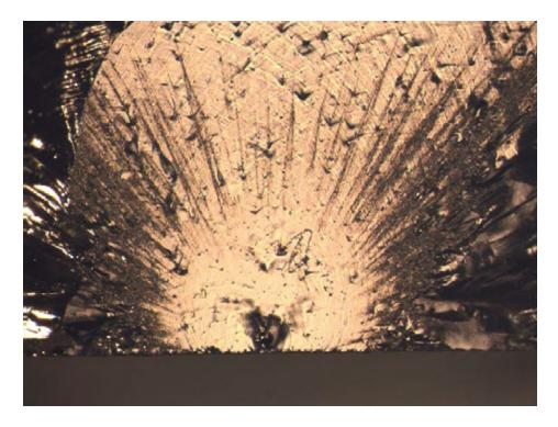
**Figure 11.2** Fracture surface of a dental glass-porcelain, flexural strength bar. One can see an origin that is a row of grinding cracks that interacted with a near-surface bubble. One also sees the fracture mirror, Wallner lines, gull wings, wake hackle, mist, and velocity hackle. (unpublished, found in Dr. J. Quinn's computer after her death.)
