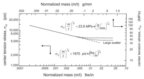
**Figure 7.5** The interior tension stress in tempered soda lime sheet and plate glass may be estimated from the average fragment mass. Center tension stress is plotted versus mass normalized by the plate thickness, t. Data for five different thickness plates and sheets from 3.2 mm to 9.5 mm (1/8 in to 3/8 in) fall on the same curve. (After Barsom, ref. 13)
