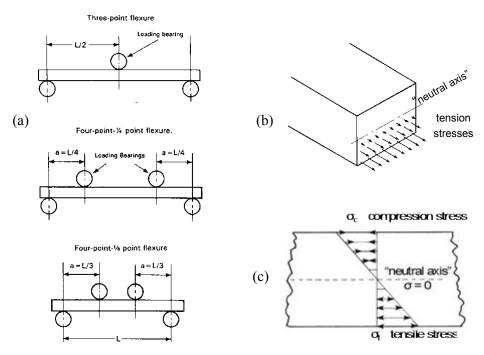
*Figure 4.8 Three- and four-point flexure test configurations are shown in (a). The stress distribution on a cross section is illustrated in (b) and (c).*
