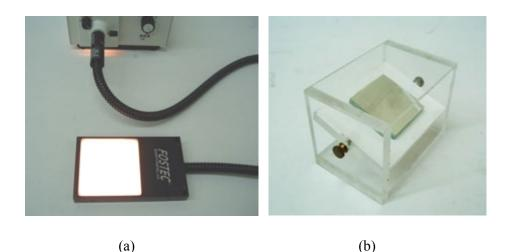
**Figure 3.22** Transmitted light can be from an illuminator plate as shown in (a) or in (b), an improvised stage made of Plexiglas, and white paper or a mirror for transmitted illumination. A fiber optic light source can be directed onto the tiltable inclined plane so that light is reflected up through a specimen mounted on the top. (Thanks to Dr. D. Shechtman for suggesting this to the author.)
