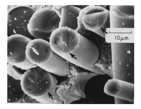
**Figure 9.5** SEM image of the fracture surface of a SiC (Nicalon) ceramic fiber – zirconia matrix composite. The arrows mark fracture origins and mirrors in several fibers. (Ref. 2, courtesy of R. Rice)
