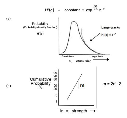
**Figure 7.41** The Weibull distribution can be derived from the flaw size distribution shown in (a). H'(c) is the probability for occurrence of a flaw of size c. n' and  $\alpha$  are constants. The largest flaws control strength and that portion of the distribution can be modeled by an inverse power law with exponent n'. (b) shows the Weibull distribution for strength. The Weibull modulus m is equal to 2n'-2.
