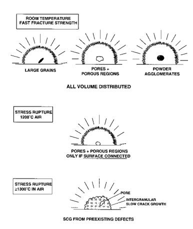
Figure 10.12 Fracture origins in  $\alpha$ -SiC.
