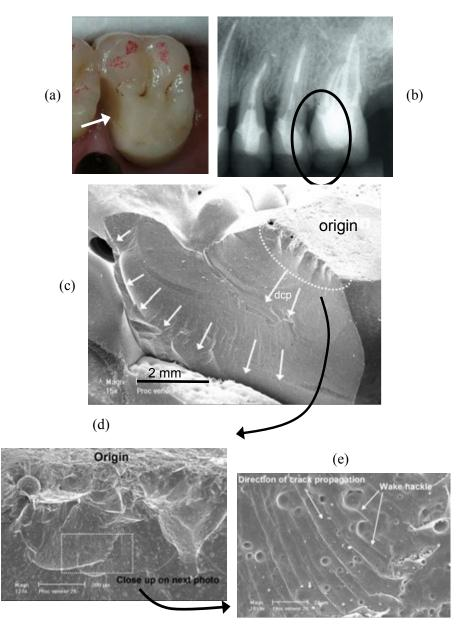
**Figure 6.81** Failure of a first upper-left molar crown. (a) shows a view onto the occlusal surface (the crown top) and the chipped porcelain veneer on the side of the crown (arrow). The porcelain veneer was inadequately supported by the alumina core as shown in the x-ray image (b). (c) – (e) show progressive close-ups of the fracture surface on an epoxy resin replica. This is the same crown as shown in Figure 3.34 on replica techniques. (All courtesy S. Scherrer, Univ. Geneva)
