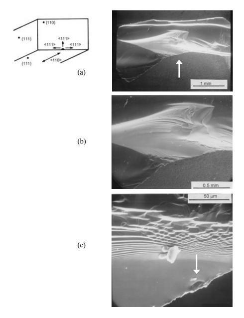
**Figure 8.13** Spinel bend bar with a {111} tensile surface and <110> tensile axis designed to cause fracture on a {110} plane. (unknown stress) (a) shows the whole fracture surface and the major crack redirection on the mirror sides. (b) shows the "**skewed cathedral mirror**," and (c) shows the grinding crack fracture origin from the matching fracture piece. (Case G1, table 8.2) (Courtesy R. Rice)
