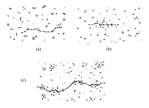
*Figure 6.75* Schematics of "microfault pockets." The fracture origin may be an array of tiny microstructural faults that are linked by microcracking. Tension stress is applied vertically. (a) is similar to a schematic by Sines and Okada.<sup>56,57</sup> (b) shows an origin site that has a greater local concentration of the irregularities. (c) shows random pockets of greater than average concentration. Fracture may entail linkage of these pockets by microcracking.
