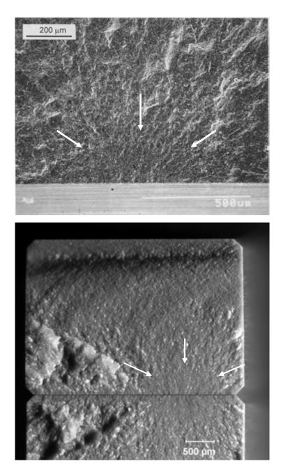
*Figure 5.18* Sideways-elongated mirrors from grinding flaws in ceramic bend bars. (a) "zipper machining crack" (section 6.7.6) in sintered reaction bonded silicon nitride. (542 MPa) (b) zipper crack in sintered silicon nitride. (432 MPa)
