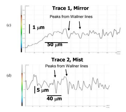
**Figure 3.51** Matching stereoptical (a) and confocal microscope (b) images of a glass rod fracture mirror. Height profiles for tracks 1 and 2 are shown in (c) and (d). The major peaks are from Wallner lines. The minor peaks show the inherent roughness in the mirror and mist regions. (b) and traces are courtesy of J. López-Cepero Borrego and A. Ramirez de Arellano Lopez, Univ. Seville.)
