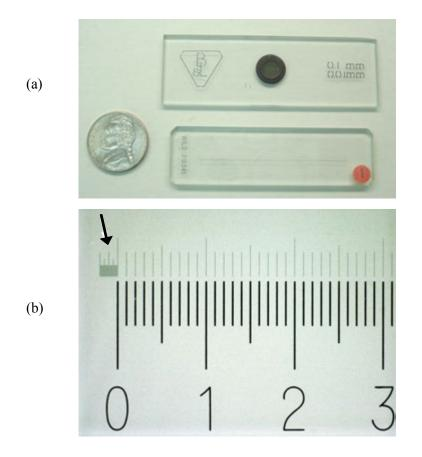
**Figure 3.27** Two stage micrometers (a). A close-up of the bottom one is in (b). The numbers show 1 mm spacings. The thin lines on the top right are 100  $\mu$ m apart. The thin lines on the top left (arrow) are 10  $\mu$ m apart. This model was accurate to an amazing 0.01 %.
