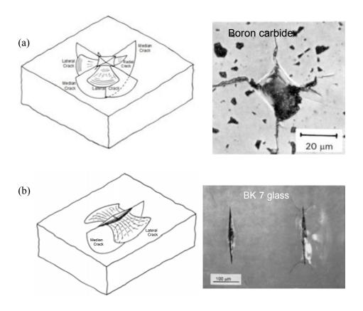
*Figure 7.36* Indentation generated damage sites. (a) and (b) show common crack patterns and examples around Vickers and Knoop indentations. The author prefers the Knoop indenter since it makes a simple crack system.
