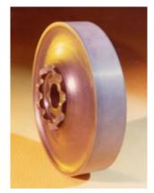
*Figure 10.1.* A Ford silicon nitride 95 mm diameter model gas turbine rotor that survived 25 h intact. The outer rim is thicker than a real rotor in order to simulate the mass of the vanes that would be attached in a real rotor.
