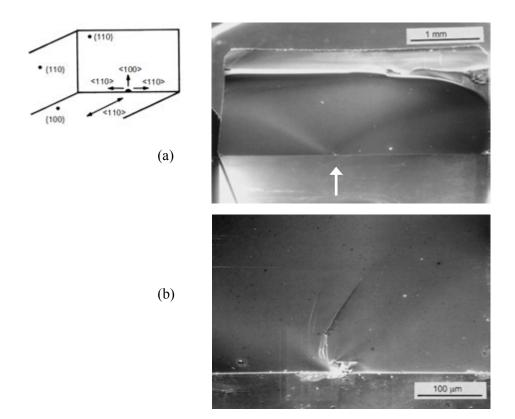
**Figure 8.9** Spinel bend bar with a {100} tensile surface and <110> tensile axis designed to cause fracture on a {110} type plane. (169 MPa) (a) shows the whole fracture surface which is flat and featureless except for the cantilever curl. The arrow shows the origin. (b) shows the grinding crack fracture origin. Fracture stays on a {110} type plane. (Case B, table 8.2) (Courtesy R. Rice)
