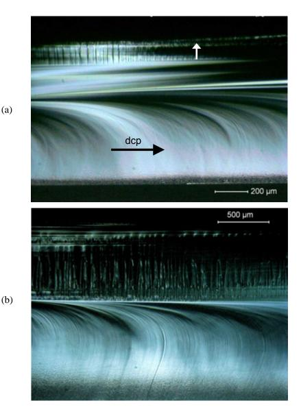
**Figure 5.29** Twist hackle. (a) shows a glass microscope slide that was broken in bending with a little superimposed torsion. The main crack fracture from left to right, leading on the bottom surface as attested to by the profusion of mist and secondary Wallner lines and an occasional primary Wallner line (described in the next section). Final break-through to the top surface (white arrow) created the twist hackle along the top. (b) shows a similar pattern but with a tempered glass fragment.
