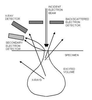
**Figure 3.41** The electron beam interacts with the specimen surface and volume creating emissions that may be analyzed. Signals are generated in all directions, but they come from different depths of the material. The beam is rastered over the surface and an image is sequentially formed.
