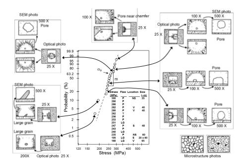
*Figure 6.80 Schematic of a fractographic montage.*
