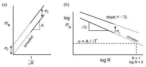
**Figure 7.38** Systematic deviations in the fracture mirror size trends for applied stress,  $\sigma_a$ , as a function of mirror radius are indicative of residual stresses. (a) shows that residual stresses create nonzero intercepts. (b) shows that residual stresses alter the slope.
