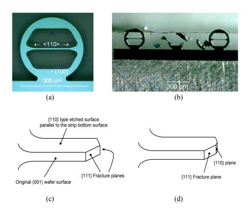
**Figure 8.20** Tiny silicon theta test specimens. The ring shown in (a) is compressed on its rim on the top and bottom in a nanoindenter causing the 7.5  $\mu$ m tall by 100  $\mu$ m thick web section in the middle to stretch in uniaxial tension. (b) shows a fractured specimen on a strip. (c) shows that the web fractures usually occurred on {111} planes which are the cleavage planes. A few initiated on {110} planes but then changed to {111} planes. Origin flaws are shown in the next figure.
