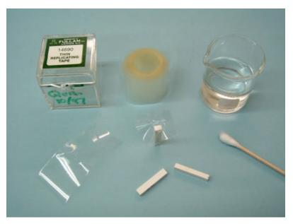
*Figure 3.31 Thin cellulose acetate replica tape, acetone, applicator, and bend bar specimens. These are used to make reversed (negative) replicas.*
