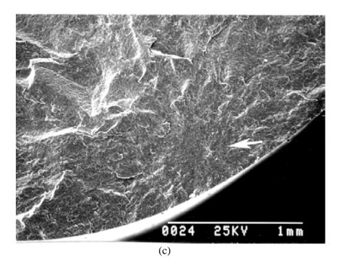
**Figure 5.9** Fracture mirrors in ceramics. (a) is a hot-pressed silicon carbide tensile specimen (371 MPa). (b) is a silicon carbide tension specimen and (c) is a silicon nitride rod broken in flexure. Many beams and rods broken in flexure have internal flaw origins if the specimens are ground carefully.
