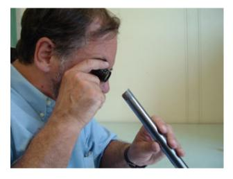
*Figure 3.3* Loupes (5X to 20X) may either be held by the eye or by hand. The part is a single crystal silicon rod.
