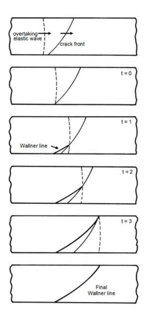
*Figure 5.43* Schematic showing the stages of formation of a tertiary Wallner line for a curved crack front overtaken by an elastic wave from behind the crack. The Wallner line has a similar concavity as the crack front, but the loci are different.
