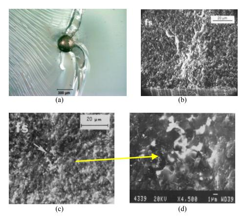
**Figure 6.17** Examples of inclusion origins. (a) is nickel sulfide in tempered glass plate that spontaneously fractured. (b) is an irregular iron and chrome inclusion in a sintered SiAlON bend bar. (c) and (d) are views of a tungsten inclusion in a hot-pressed silicon nitride bend bar.
