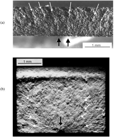
*Figure 5.23* Coarse microstructural hackle. (a) is a broken O-ring specimen of a ceramic membrane material. (b) is a silicon nitride bend bar with a Knoop indentation flaw on the bottom middle (black arrow). Coarse microstructural hackle lines (white arrows) guide the observer back to the origins. The only other fractographic feature observable is the compression curl in (b). Both specimens are so weak that fracture mirrors are larger than the cross sections.
