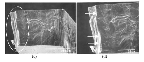
**Figure 10.22** A broken notched miniature SiC tensile specimen. (a) shows the whole specimen. (b) shows a close-up of the gage section notches. Transillumination through the green single crystal SiC grains created the light patches. They are individual grains. (c) and (d) show the fracture surface. Fracture started at the bottom of the round notch (arrows), from a etch groove linked with a single long and large columnar SiC grain that ran from the top to the bottom.
