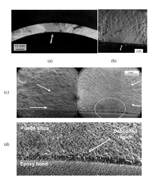
**Figure 10.20** Sintered fused silica radome fracture. (a) shows the origin site on the inside wall. (b) is a close-up showing a fracture mirror centered on a feature on the inside wall of the ceramic at the top of the bond line. (c) is a composite of two SEM photos of the origin area. The origin is less obvious, but hackle lines point back (white arrows) to the circled area. (d) shows there is no significant material flaw at the origin, but the ceramic and the epoxy are debonded at the origin.
