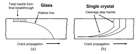
*Figure 8.6* Schematics showing (a) a Wallner line and twist hackle in a glass plate loaded in bending and (b) "cleavage step hackle" in a single crystal plate loaded in bending. In both cases the crack was leading on the bottom surface.
