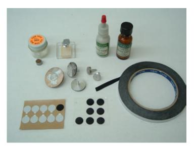
**Figure 3.39** SEM specimen preparation tools. Clockwise from the top left are two SEM length calibration standards, two silver paint bottles, a double-sided conductive adhesive tape roll, two sheets of double-sided conductive adhesive disks, and an assortment of aluminum stubs.
