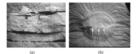
*Figure 6.51* Delaminations revealed on the fracture surfaces of two tape-cast PZT bend bars. (a) has severe delamination between tape cast layers. (b) was processed much better but still had a very small horizontal delamination (arrows). The curved lines are arrest lines on the fracture surface. (courtesy C. Wu.)
