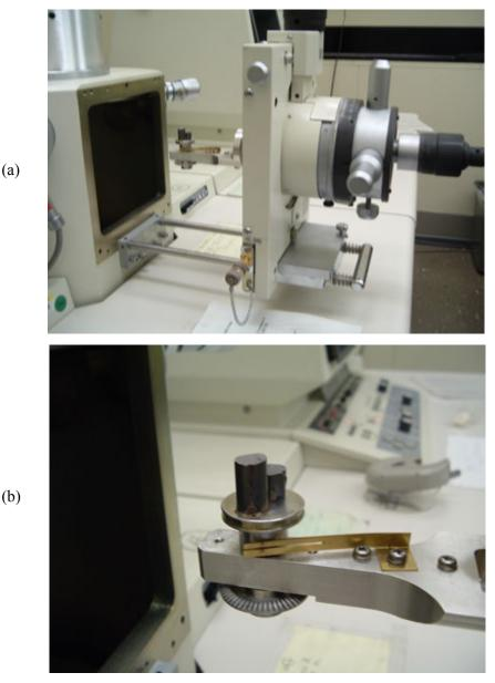
*Figure 3.37* (a) shows an open SEM vacuum chamber showing the specimen station on the left and the positioning controls on the right, outside of the chamber. (b) shows a close up of the two fracture specimens on their stub on the examination mount. Both fragments had to be cut from longer pieces to fit in the chamber. This model has a large opening and the stage can accommodate specimens as tall as 25 mm.
