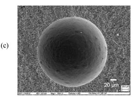
**Figure 6.10** Internal pore-bubbles in ceramics and glass ceramics. (a) and (b) show an internal spherical pore fracture origin in a cordierite glass ceramic bend bar (315 MPa). The pore was from a bubble in the original glass. The material crystalized around the bubble during the ceraming step. The arrows mark the hackle boundary of the fracture mirror. (courtesy D. Lewis, III) (c) shows a large internal seeded-pore origin in alumina. (courtesy T. Bernthaler)
