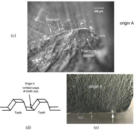
Figure 10.5 Fracture surfaces showing a fracture mirror and the origin site *A*, which is a surface crack from grinding. (b) and (c) highlight the fracture mirror and grinding crack origin at site "A." The primary fracture origin was contact crack damage at site "h" on the curvic coupling teeth as shown in (d) and (e). Origin "h" is marked by the larger arrow on the right. Notice how the radiating hackle lines converge on it.
