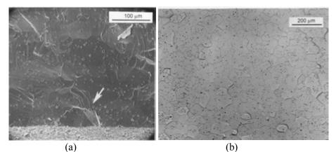
**Figure 6.68** Baseline microstructure flaw in a sintered aluminum oxynitride four-point flexure bar. (a) shows a single grain that was the fracture origin. The origin in this case may actually be the grain boundary around the grain. (b) shows a polished section view of the microstructure.
