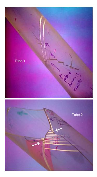
*Figure 8.25* Twin bands became very apparent when the sapphire tubes were illuminated by light from crossed polarizers. Cracks initiated at twin band intersections (white arrows) and then were propagated by cool down thermal stresses. (Photos courtesy R. Pingree)
