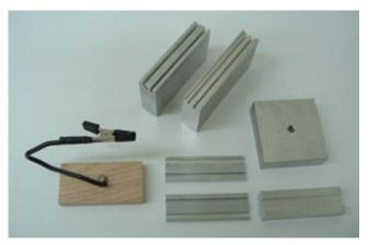
**Figure 3.5** Specimen holders. Clockwise from the lower left are: a bend bar holder made with an alligator clip on a bendable (10 gage electrical) wire with electrical tape wrapped around the teeth to cushion the specimen, two aluminum jigs with slots and grooves for bend bars or tension strength specimens, an aluminum block with hole, and three aluminum holders comparable in size to a glass microscope slide with groves to hold bend bars both on their flats and on edge for chamfer examination.
