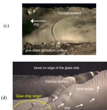
**Figure 5.50** Examples of glass glue chips. (a) shows an Alfred University demo plate covered with glue chips. (b) is a close-up of isolated glue chips on the surface. (c) shows a side view of a broken plate that shows glue chips on the bottom that affect crack propagation. (d) shows large glass disk that fractured from a glue chip caused by an epoxy bond to a metal part.
