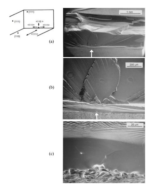
**Figure 8.15** Spinel bend bar with a {110} tensile surface and <111> tensile axis designed to cause fracture on a {111} plane. (325 MPa) (a) shows the whole fracture surface and the major crack redirection on the top half, (b) shows the "gull wing mirror," and (c) shows the grinding crack fracture origin. (Case E, table 8.2) (Courtesy R. Rice)
