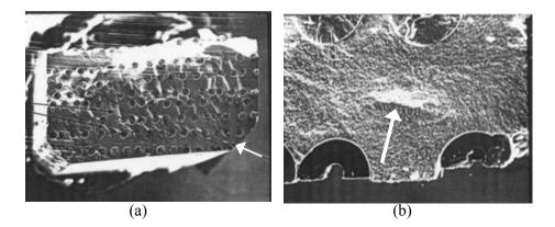
**Figure 9.3** Fracture surface of CVD SiC filament reinforced  $Si_3N_4$  bend bar. (Ref. 1) (a) shows that there was not very much fiber pullout in this case. Wake hackle in the matrix behind the filaments are telltale indicators of the local direction of crack propagation through the matrix and lead back to the origin, which is a porous seam in the matrix shown by the white arrows in (a) and (b).
