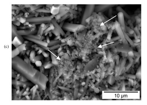
**Figure 5.67** Bend bar that was tested to fracture in cyclic fatigue loading. The material was a yttria and alumina additive sintered silicon nitride with an elongated grain structure for enhanced fracture toughness. (a) shows the bend bar fracture surfaces with the origin marked by the arrow. (b) shows a typical fast fracture portion of the fracture surface. (c) shows the origin region and fine debris (arrows) created by fatigue cycling. (courtesy T. Lube and R. Danzer)
