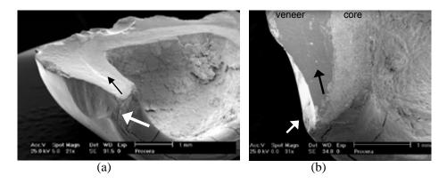
**Figure 10.27** SEM images for the Figure 10.26 Procera crown that broke from a margin chip (arrows). The final fracture that split the crown started at the bottom at the margin, from part of the margin chip, and ran as shown by the black arrows. (images courtesy of S. Scherrer)
