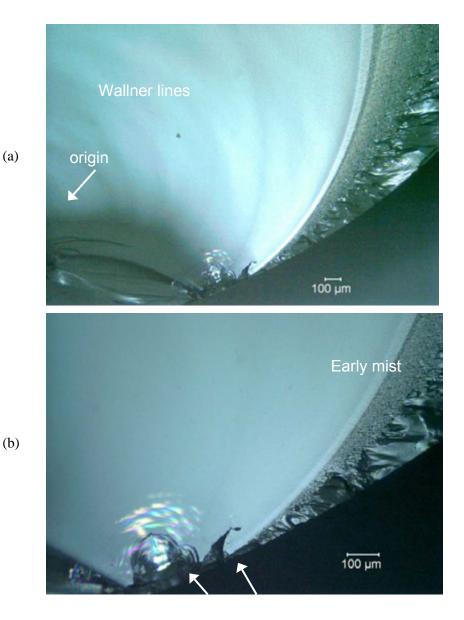
**Figure 5.6** Early mist and hackle. (a) and the enlargement (b) show an example of early formation of mist. The Wallner lines in (a) suggest the origin is off to the left in the image. The crack radiating outwards encounters other cracks in the surface shown by the arrows in (b). A strong primary Wallner line is generated and it triggers mist earlier than normal during mirror formation.
