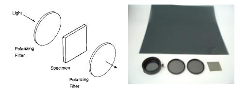
*Figure 3.23* Crossed polarizing filters or plastic sheets. Polarizers can either be dedicated accessories for the stereoscope, or can be improvised from ordinary single lens camera lens attachments or sheets of plastic polarizing film.
