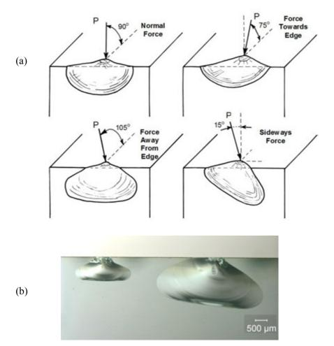
*Figure 4.26* The angle of the applied load affects the shape of edge chips. (a) is a schematic that shows the patterns and (b) shows front views of two chips in glass (at different loads and distances from the edge) made by a conical indenter tool angled away from the edge at 105°. (after J. Quinn and R. Mohan, Ref. 33).
