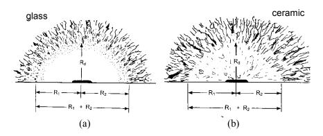
**Figure D.10** Grinding cracks and scratches can cause mirror elongations along the surface, even in bend bars with stress gradients. (a) shows a schematic of such a mirror with the mist-hackle boundary marked in glass, and (b) shows a comparable image in a polycrystalline ceramic. It has some intrinsic microstructural roughness inside the mirror and the mirror-hackle boundary is marked. Use an average radius:  $R_{avg} = \{(R_1 + R_2 + R_d)/3.$
