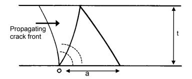
**Figure 5.46** Wallner lambda line mark. The schematic shows the advancing crack (thinner line) encountering a discontinuity at point O. An elastic pulse creates a radiating elastic wave. The intersection of the wave and the advancing crack front creates a primary Wallner line that runs upward to the top surface. When the elastic wave reflects from the opposite surface, the Wallner line continues back downward.
