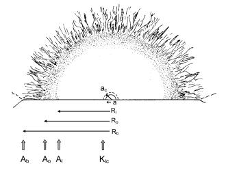
**Figure 7.7** Fracture mirror schematic.  $R_i$  is the inner or mirror-mist boundary,  $R_o$  is the mist-hackle boundary, and  $R_b$  is the branching distance. The fracture toughness  $K_{Ic}$  (discussed in section 7.5.1), the mirror constants  $A_i$ and  $A_o$  and the branching constant  $A_b$  correspond to each of these boundaries. All have units of stress Vlength.
