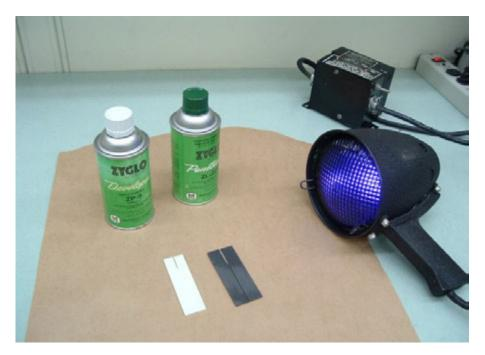
*Figure 3.55 Fluorescent dye penetration equipment. Two double torsion specimens are shown. The white one is an alumina, the black one, a silicon nitride.*
