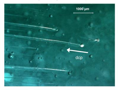
*Figure 5.24* Wake hackle, the fractographers "weather vane" for crack propagation. This shows wake hackle from bubbles in glass. The direction of crack propagation (dcp) is shown by the arrow. Many bubbles are beneath the surface in this view.
