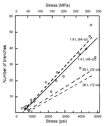
**Figure 7.2** Fragmentation of internally pressurized bottles. The number of branches (fully developed that extend more than 13 mm beyond the first fork) are shown versus the hoop stress in the glass wall for four different glass containers. Data points and a solid line are shown only for the 1.4 L (48 oz) bottles. Dotted lines show the trends for the three other sizes. Some of the scatter is due to variations in the glass wall thickness. (After Fréchette and Michalske, Ref. 3)
