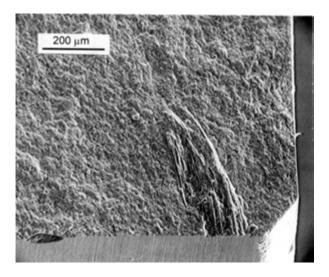
**Figure 9.1** Nonuniform dispersal of toughening agents often causes strengthlimiting flaws in ceramic composites. This figure shows a whisker clump that was the strength-limiting flaw in a siliconized SiC bend bar. The material was made by mixing chopped carbon fibers with SiC starting powders and then infiltrating with silicon. The carbon fibers were intended to react with the silicon to form dispersed silicon carbide fibers that would toughen the matrix.
