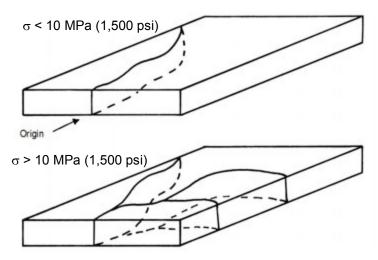
**Figure 7.1** Schematic of thermal fractures of windows. Low stress fractures  $(\sigma < 10 \text{ MPa}, 1,500 \text{ psi})$  do not cause branching. (After  $Orr^2$  and  $Fréchette^1$ )
