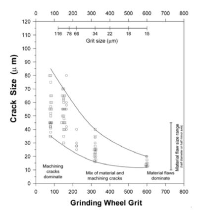
*Figure 6.41* The depth of grinding cracks as a function of grinding wheel grit in a silicon nitride. The notes show the strength-controlling flaws. Ref. 32
