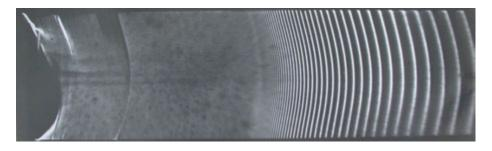
*Figure 3.52* Fracture in a glass plate. Fracture originated at the left and accelerated to the right as attested to by the increased spacing between the timing ripples. (Courtesy H. Richter)
