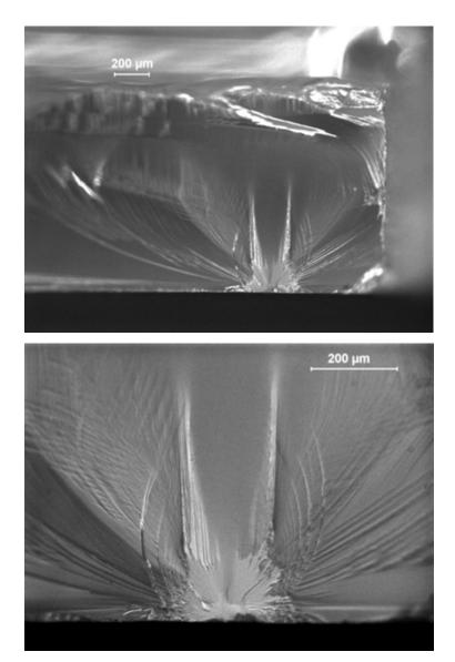
*Figure 8.16 "Batman mirror"* in a sapphire bar. (a) shows matching halves of the bend bar with a tensile surface parallel to the a-plane and bend bar sides oriented so as to cause fracture on the r-plane. The tensile direction was the r axis. The origin was grinding damage. (Specimen courtesy R. Krause.)
