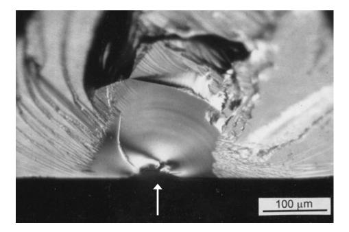
**Figure 8.19** Impact crack fracture origin in a hemispherical sapphire dome that was impacted by a small particle while the dome was under thermal stress. The impact site on the surface is missing a small divot (arrow) and the approximately 150 µm deep crack shows concentric semicircular tertiary Wallner lines that are telltale signs of impact. See Figure 4-15 on page 4-25 for views of the entire dome.
