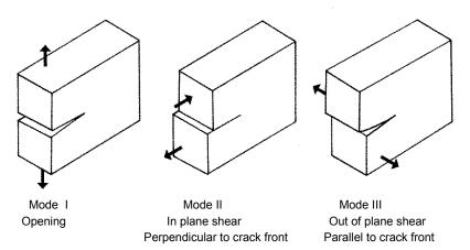
Figure 7.14 Loading modes on a crack
