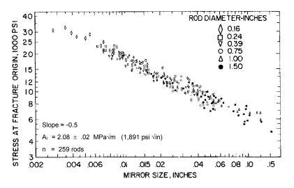
**Figure 7.10** A superb example of fracture mirror data for glass rods of many sizes and strengths. Two hundred and fifty-nine Pyrex 7740 rods varying in size by almost a factor of ten (4.1 mm to 38.1 mm) were broken in three-point flexure by Kerper and Scuderi at the National Bureau of Standards in 1964.<sup>32</sup>
