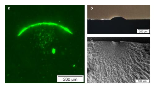
**Figure 3.57** C contact damage crack in a silicon nitride ball. (a) shows the outer surface and the crack highlighted by fluorescent dye penetrant. (b) shows one half of the notched ball after it was broken. (c) shows the fracture surface. (Courtesy T. Lube and R. Danzer, Mountain University Leoben).
