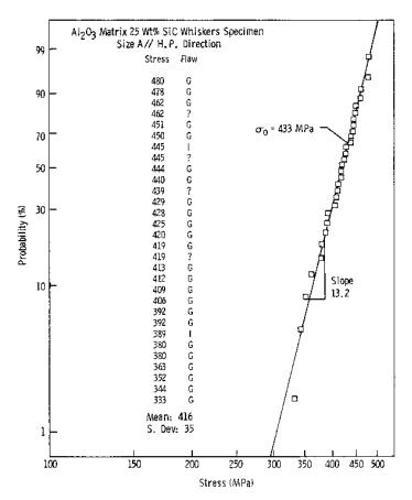
**Figure 7.39** Fractographically-labeled Weibull graph. Four-point flexural strength data for a SiC whisker-reinforced alumina. "G' is an abbreviation for a large grain origin type, "I" is for inclusion, and "?" is unknown. The slope of the fitted line is the important Weibull modulus (m) parameter. It is a measure of strength variability.
