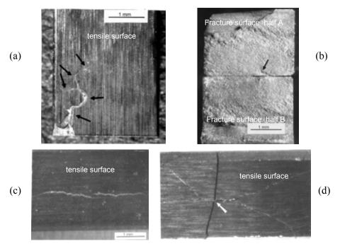
**Figure 6.48** Examples of processing cracks. (a) shows the tensile surface and (b) the fracture surface of two different silicon nitride bend bars which had an unstable boundary phase associated with yttrium silicates. (c) shows a bend bar that had a moderate strength despite a huge processing crack running perpendicular to the tensile axis. The origin was at the arrow. (d) shows another example of a firing crack in a bend bar. The origin is marked by the arrow.
