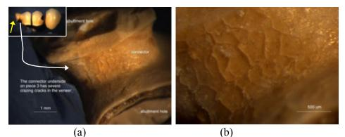
**Figure 6.72** Glazes can be preferred sites of fracture initiation. This was an in vivo broken three-unit zirconia bridge (courtesy T. Kosmac) with a crazed veneer probably from a mismatch of the veneer type to the ceramic. Fracture started on the plane on the left insert marked by the yellow arrow.
