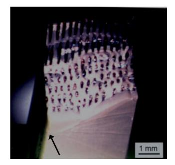
**Figure 9.2** A CVD SiC (SCS-6) filament-reinforced  $Si_3N_4$  bend bar tilted back at an angle so as to view the fracture and tensile surfaces. A series of branching cracks radiate outwards from one origin site (arrow).
