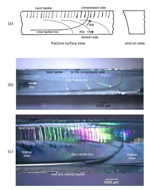
**Figure 5.34** Step hackle schematic (a). (b) and (c) show a piece of a large (1.5 m by 0.75 m) glass mirror that fell off a wall in the author's home. The mirror broke into over 100 pieces. Many fragments had evidence of bending and twisting. Notice the opposite arcs of the step hackle line and the Wallner lines (thin dashed lines in a).
