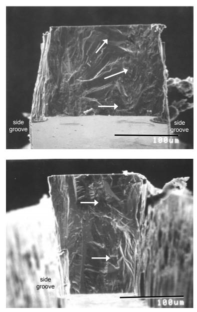
**Figure 5.30** Twist hackle in grains. (a) and (b) show fracture surfaces of chemical vapor deposition (CVD) silicon carbide micro-tensile specimens. CVD materials often have coarse, columnar grains. Such grains run from top to bottom in this view. Twist hackle in these grains in both images show that fracture propagated from left to right as shown by the arrows. Fracture occurred from cracks located at the bottom of the grooves on the left side in both cases.
