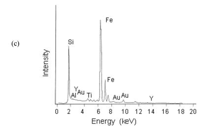
*Figure 3.45* An iron inclusion in a silicon nitride rod (684 MPa). Matching secondary electron (a) and backscattered electron images (b). (c) is the EDX pattern of the inclusion revealing it is iron.
