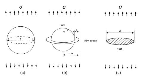
*Figure 7.26 Flaws may be three-dimensional. A flat penny shaped crack (c) is a two-dimensional approximation.*
