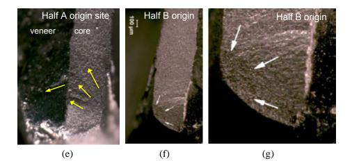
**Figure 10-25 continued.** (c) and (d) are examples of wake hackle from pores in the veneer. (c) is an optical image, and (d) is an SEM image. (e)-(g) show optical images of the margin. The origin is a subtle margin crack as marked clearly in (f) and (g). This origin crack was so flat and coplanar with the final fracture surface, that it did not stand out well in SEM images. (all images courtesy of J. Quinn and S. Scherrer)
