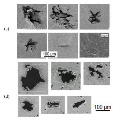
**Figure 6.78** Polished microstructural sections can aid origin interpretation. (a) Sintered alpha silicon carbide often has large grain fracture origins. The acicular or platelet shape of these and their concentration are revealed by the micrograph. (b) reaction-bonded silicon nitride sometimes fails from unreacted silicon (arrow). (c) and (d) show irregular pressing flaws on fracture surfaces and polished sections of a sintered alumina, respectively. (c and d courtesy T. Bernthaler)
