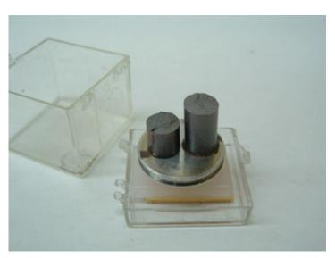
*Figure 3.38* Two matching fracture halves of a broken round tension specimen on a stub in a protective plastic box. Silver paint was used to attach the specimens to the stub. Ideally, the halves should have been cut to similar lengths to save time refocusing in the SEM.
