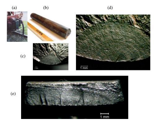
*Figure 5.65 Classic metal fatigue striations in (a-d,) a steel railroad coupler pin (see also Fig. 3.21), and (e) an aluminum bicycle bracket. An arc line does not necessarily correspond to one loading cycle.*
