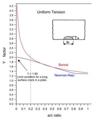
*Figure 7.24* Comparison of Bansal's approximation to the Newman-Raju solution for Y of semielliptical flaws in uniform <u>tension</u>. The approximation is only suitable for a/c > 0.2.
