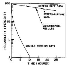
**Figure 10.3** Reliability versus time showing reliability predictions based on three different types of laboratory test data (solid lines) versus the actual outcomes for six rotors that failed.(Refs. 1,2) The actual failure times matched the predictions based on stress rupture data. The two solid points correspond to rotors that were fractographically analyzed by the author.
