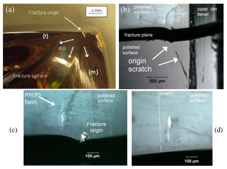
*Figure 10.38* The second refractor lens also broke from damage on the rounded surface, but from a scratch. (a) shows the fracture surface. (b) shows the scratch on the outer polished surface. It curves at the origin site. With careful lighting in (c) and (d), "micro-twins" near the origin site are revealed.
