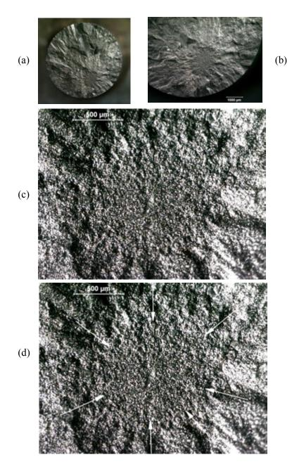
**Figure D.2** Silicon carbide tension strength specimen (371 MPa) with a mirror centered on a compositional inhomogeneity flaw shown in Figure 6.20a,b. Note how clear the mirror is in the low power images. The mirror boundary (arrows in d) is where systematic new hackle forms and there is an obvious difference compared to the roughness inside the mirror region.
