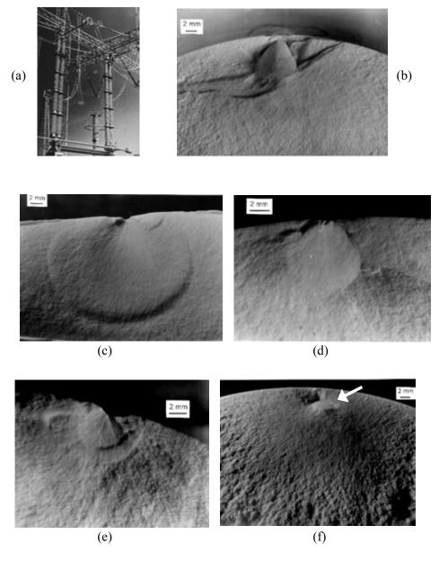
**Figure 6.33** Blunt impact origins in electrical insulator porcelains. (a) shows the installed insulators. (b) and (c) are blunt impact damage from "BB" gun projectiles. (d) is damage from a sling shot projectile. (e) and (f) are impact origins from contact with support structures. Note the partially exposed cone in (f) (arrow). (Photos courtesy of J. J. Taylor and R. W. Rice)
