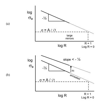
**Figure D.15** Plot of  $\log \sigma_a$  versus  $\log R$  for residual stress-free parts (a) and parts with residual stress (b). Compressive residual stresses move the locus upwards, but with a different slope and intercept. Tensile residual stresses move the loci below the baseline curve (not shown).
