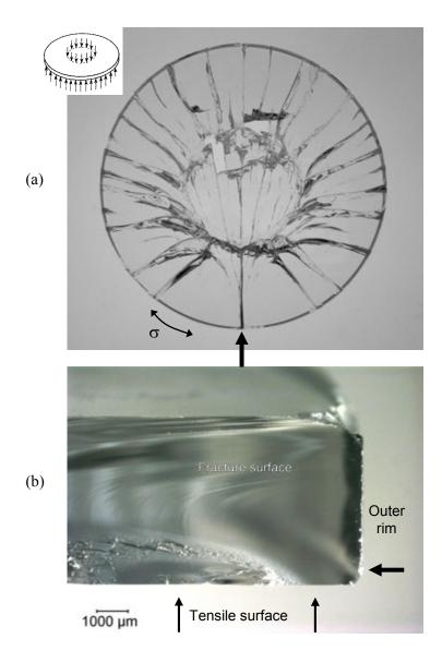
**Figure 4.13** A fractured glass ring-on-ring tested disk. (a) shows the overall breakage pattern. Fracture started on the rim (large arrow) in response to the uniaxial hoop stress  $\sigma$  (small arrows), propagated towards the middle, and branched in response due to the greater biaxial stresses in the middle. (b) shows the fracture surface. The origin is a grinding crack on the outer rim (large arrow).
