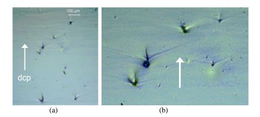
**Figure 5.39** Gull wings are a variant of primary Wallner lines. (b) is a closeup of (a). Most of these pores also have wake hackle as well. These images are from obsidian with crack propagation from bottom to top as shown by the arrows. The wing angles can be used to measure crack velocity (section 7.9). (specimen courtesy A. Tsirk)
