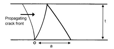
*Figure 7.31* The spacing between the lambda line legs can be used to estimate crack velocity.
