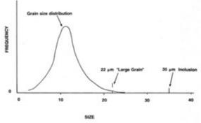
*Figure 6.67* Careful processing may eliminate severe flaws such as inclusions or gross pores. In the absence of such flaws, the material may fail from "baseline microstructure" origins.
