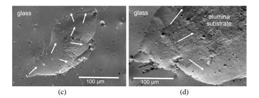
**Figure 5.51** Glue chipping damage in a thick-film resistor that cracked during thermal cycling. (a) shows the component in its epoxy encapsulant. (b) shows the exposed electrical circuitry. Scallop cracks (white-colored reflective patches) formed in an inner glass encapsulating layer. (c) and (d) show two glue chips in the glass. The arrows show the direction of crack propagation. (all photos and interpretation courtesy R. Tandon and S. Monroe)
