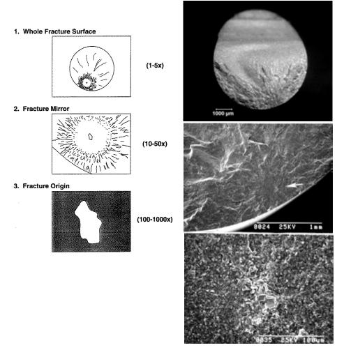
*Figure 6.79 Multiple photos should be taken showing whole fracture surface, the mirror region and the origin. The right side shows an example for an inclusion in a silicon nitride rod flexural strength specimen.*
