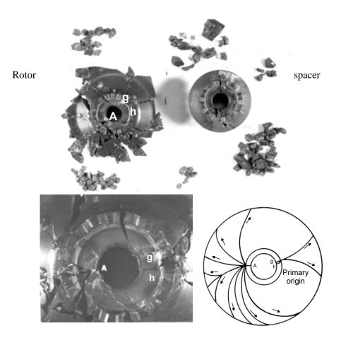
**Figure 10.4** Reconstructed model rotor and spacer. Fracture initiated either at location "A" on the left side of the bore of the rotor or at two locations "g" or "h" on the opposite side. Fracture started at "h." Fracture "g" occurred later. The lower schematic shows the overall fracture pattern in the rotor.
