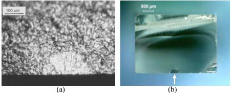
**Figure 6.53** Examples of nice, clean Knoop indentation flaws. (a) shows a precrack in a sintered alpha silicon carbide bend bar. (b) shows a BK-7 borosilicate crown glass bend bar. (c)-(h) are on the next page
