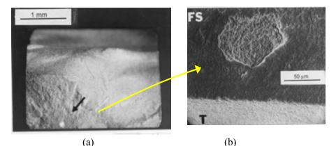
**Figure 6.3** Wherever possible, describe flaws by what they are, not how they appear. (a) shows a white spot at the origin in a reaction-bonded silicon nitride bend bar. The SEM image of the origin in (b) shows the origin is a pore. FS denotes fracture surface and T denotes tensile surface.
