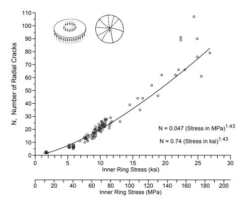
**Figure 7.3** The number of radial cracks that reach the outer rim as a function of fracture stress for 76 mm diameter by 5.4 mm thick borosilicate crown glass disk broken in ring-on-ring flexure. Data for this graph included only fractures that initiated inside the inner loading ring.
