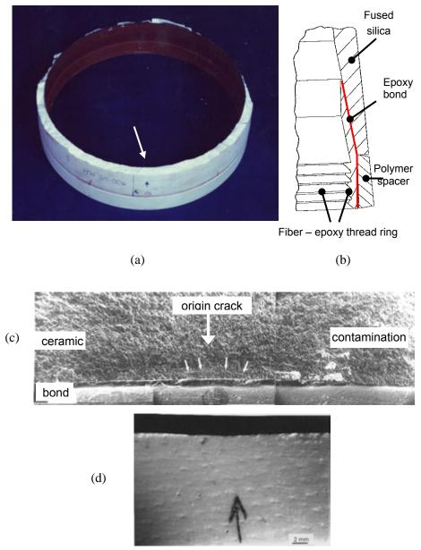
**Figure 10.19** Sintered fused silica radome that fractured during a proof test. (a) is a top view with the origin region marked by the arrow. The ceramic is bonded on the inside to a fiber epoxy attachment ring. (b) is a schematic showing the bottom of the radome where it was attached to the thread ring. Fractures in the ceramic typically occurred near the top of the thread ring. (c) shows a grinding crack at the origin area (arrows). (d) shows a grinding pattern on the inside ceramic surface.
