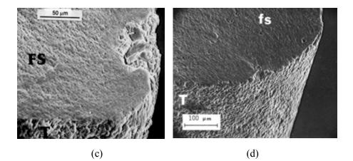
**Figure 6.26** Examples of pit fracture origins. (a) - (c) are in oxidized hotpressed silicon nitride. (b) is a close-up of (a). (d) is a reaction-bonded silicon nitride.
