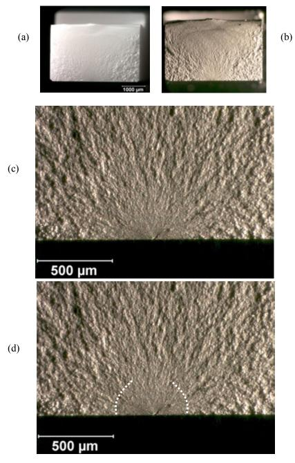
**Figure D.5** Fracture mirror in a 3Y-TZP zirconia flexural strength specimen (3M-ESPE Lava, 798 MPa). (a) and (b) are uncoated and gold coated images of the whole fracture surface, respectively. (Images courtesy J. Quinn)
