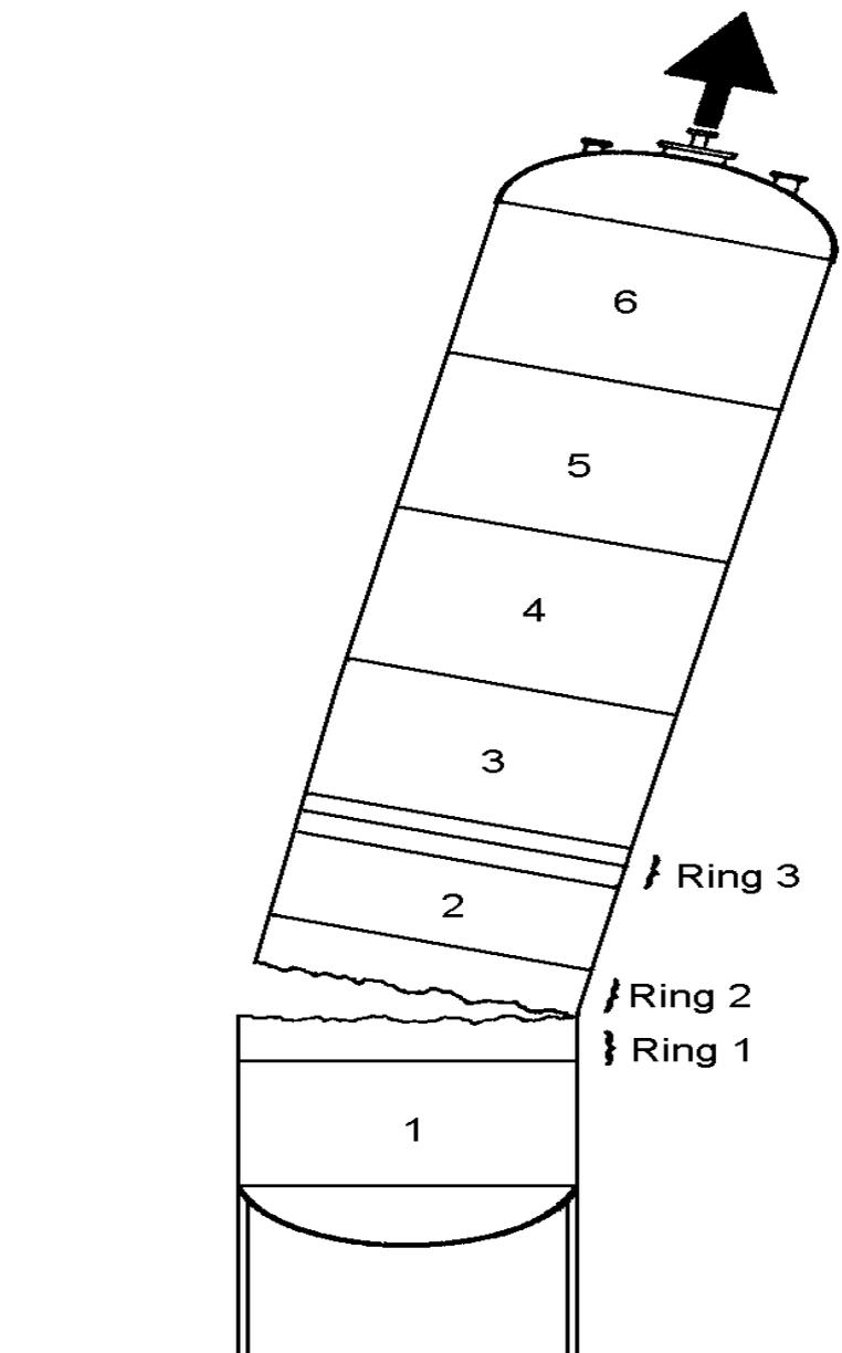
Fig. 2. The pressure vessel ruptured adjacent to the repair weld joining Courses 1 and 2.
