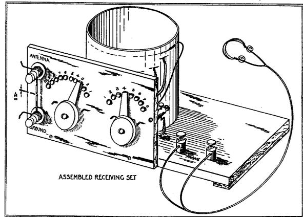
Fig 1. The crystal radio described in Circular 120.
