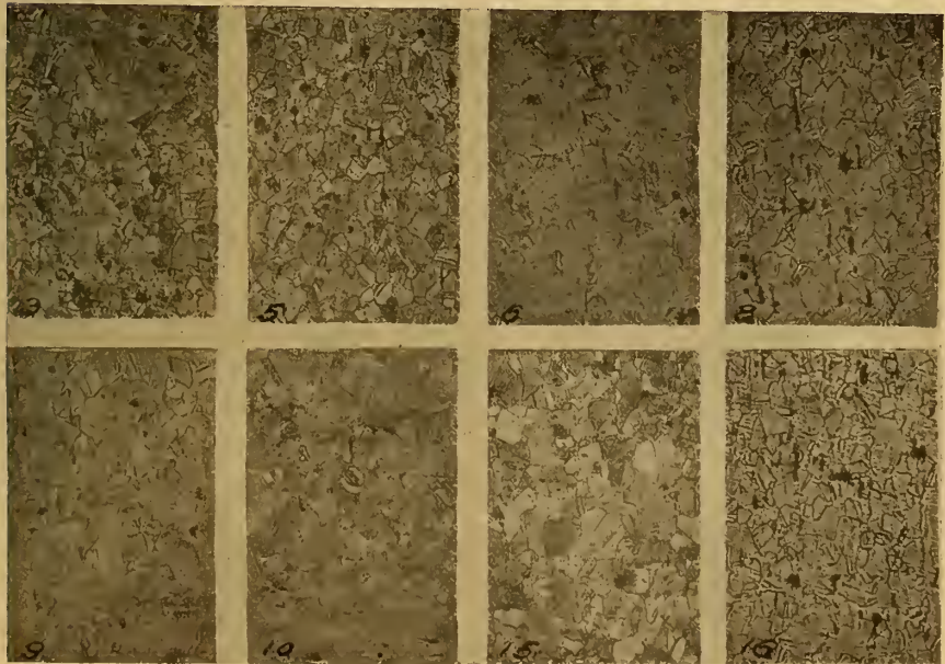
FIG. 23.—Microstructure of cold-drawn monel metal rod (alloy 34, Table I). \times 100
