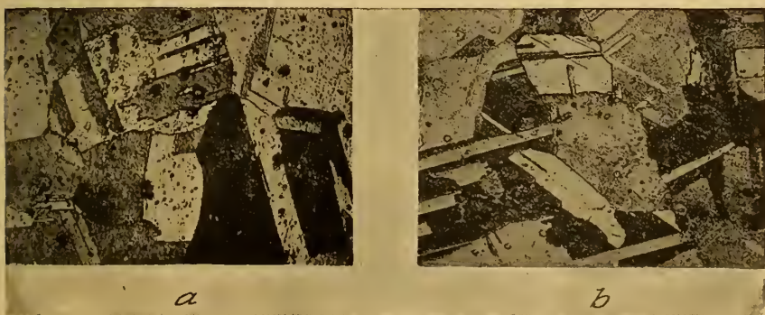
FIG. 4.—Microstructure of annealed \alpha brass illustrating the importance of a surface film produced by oxidation in producing contrast. \times 100
