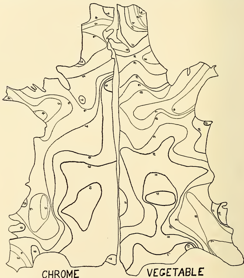
FIG. 9.—Topographical illustration of the difference and variation in thickness of a side of chrome tanned sole leather and a side of vegetable tanned sole leather, both tanned from the same hide. Series 2
