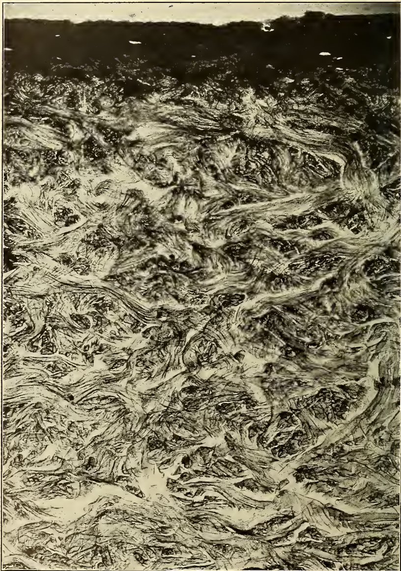
FIG. 3.— Cross section of chrome tanned sole leather from water buffalo hide comparison with commercial vegetable tanned material, which was made from steer hides. Accordingly in series 4 the leather from three chrome tanned buffalo hide bends was compared with the
