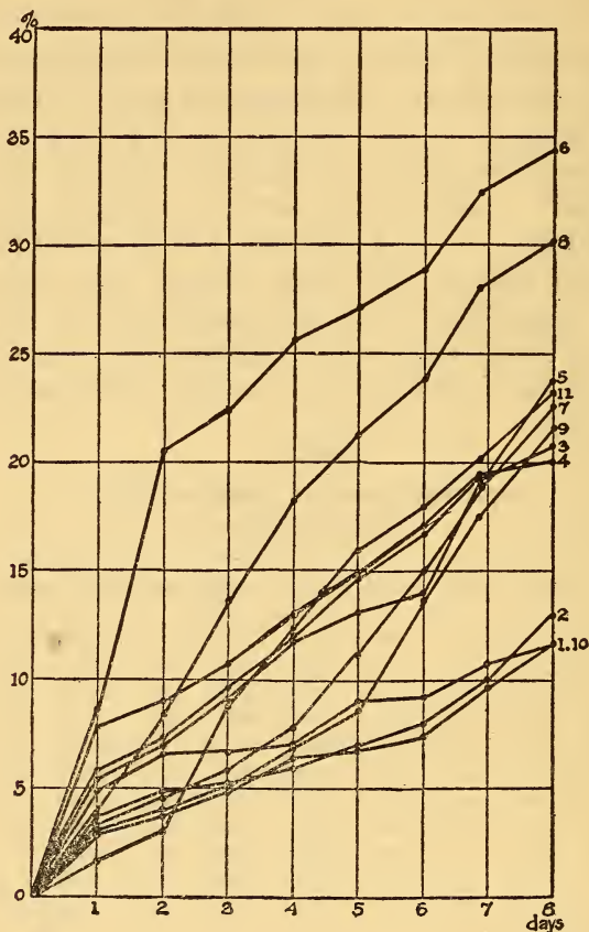
FIG. 4.—Percentage losses in weight at 110^{\circ} C. Samples 1 to 11
