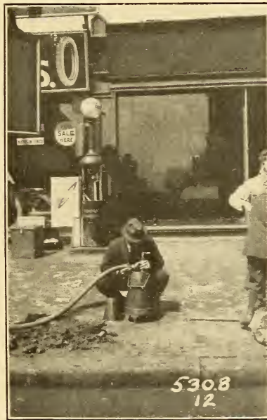
FIG. 21.—In testing outfits which have a low hose connection, care must be taken to insure drainage to a constant level if complete drainage of the hose is not feasible. In this illustration the inspector is supporting the discharge cock at the level of the top of his standard measure. A stand or support might well be supplied for use in such cases. Note that the pump in the background must force the measured liquid through a long pipe line under the sidewalk
