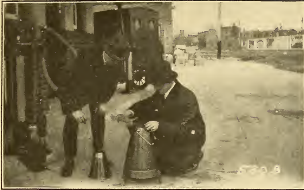
FIG. 20.—Testing with a 5-gallon standard, slicker plate, and graduated cylinder. A conical 1-gallon measure is seen at the left
