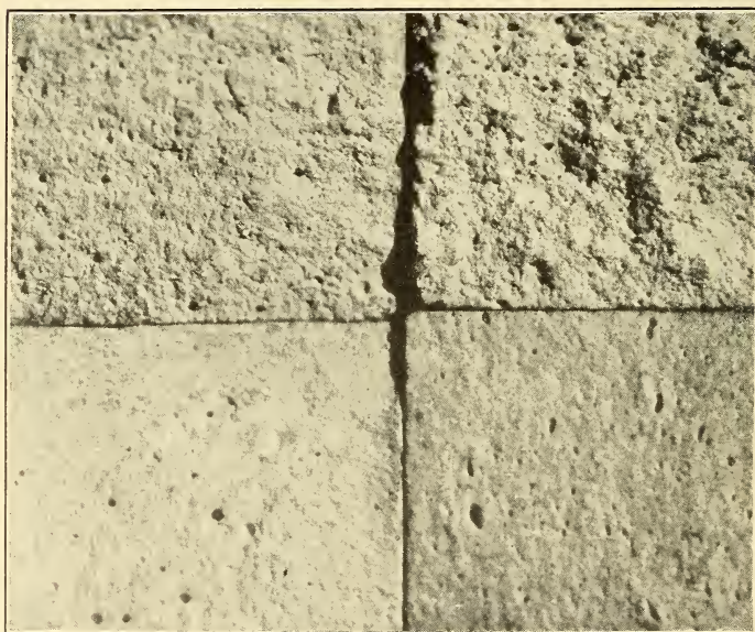
FIG. 19.— Fractures obtained in breaking some of the briquettes of burns 35 and 36
