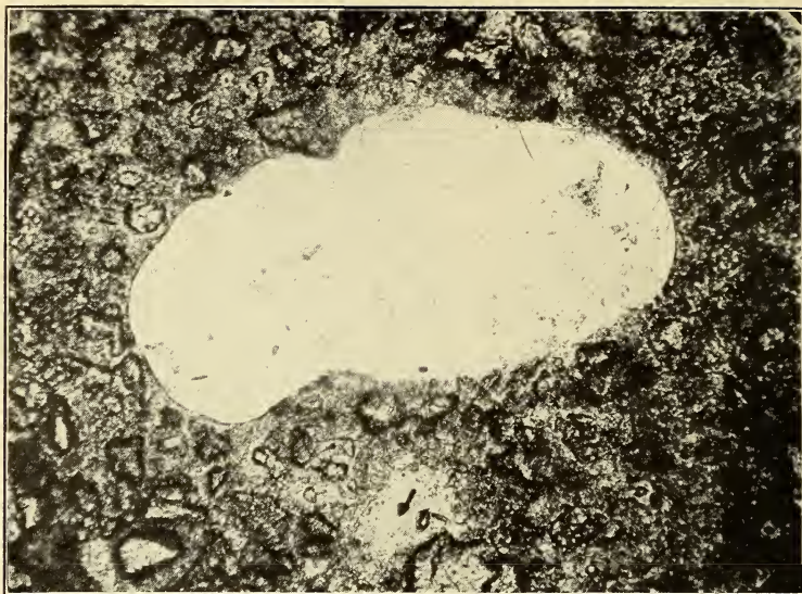
FIG. 16.—A thin section of a one-year briquette of 3SS
