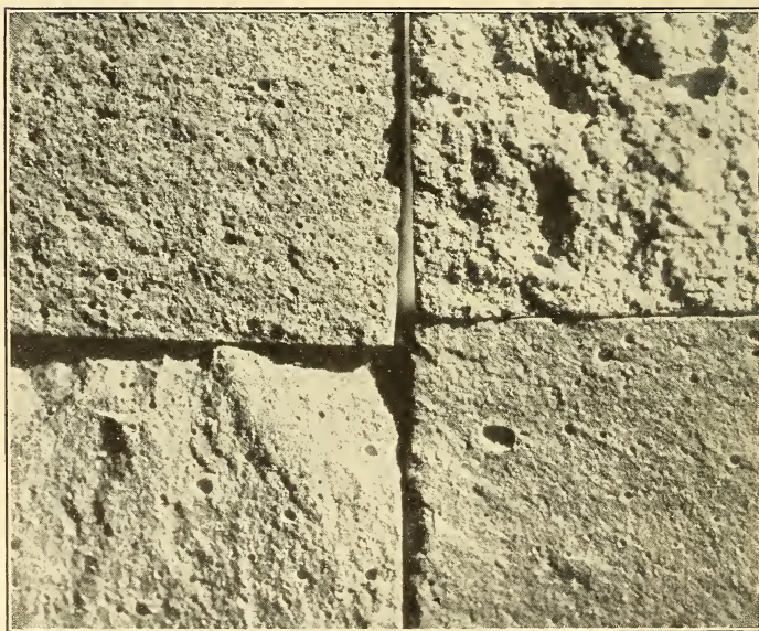
FIG. 21.—Fractures obtained in breaking at different periods neat briquettes of a commercial Portland cement
