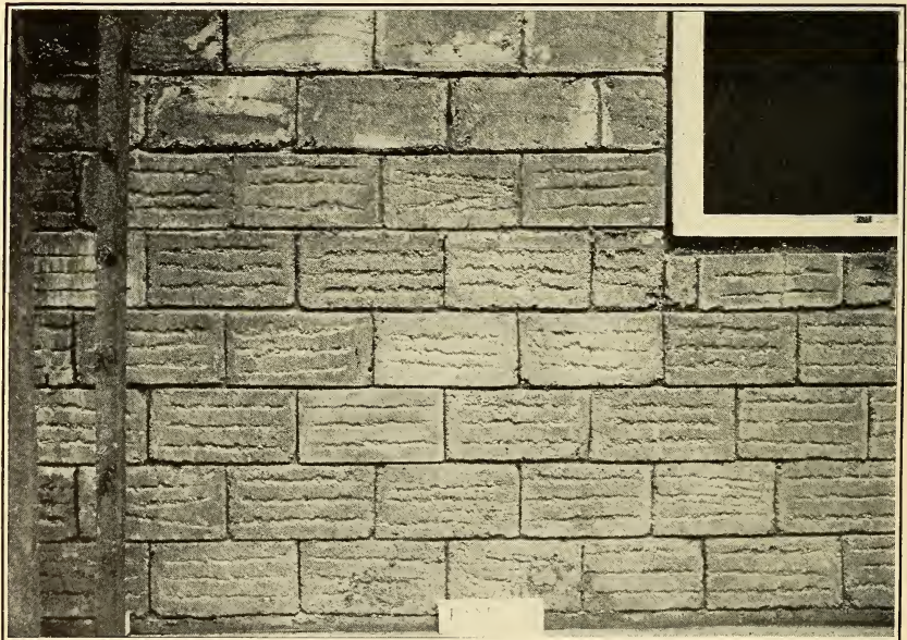
FIG. 20.—Concrete block panel No. 30, rough block on lower half, smooth block on upper half, two courses of which are shown
