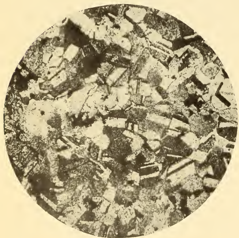
C , Specimen 418; 100X. Part of the recrystallized peripheral layer of A
