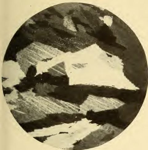
A, Specimen 524; 5X. Poured as a chill bar at 1285° C.
