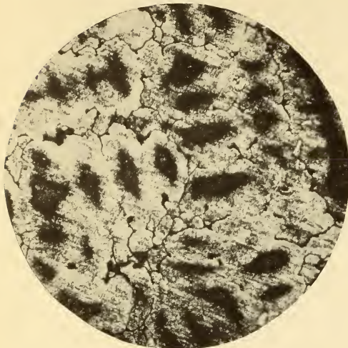
A, Specimen 475; 100X. The dark network is the film of oxide
