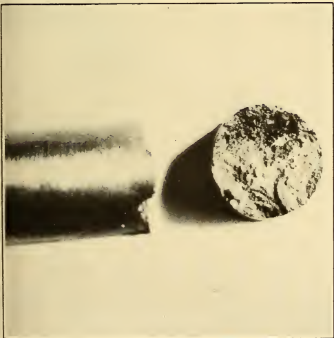
C, Specimen 475; 2X. Ultimate tensile strength, 19,800 pounds per square inch; elongation in 2 inches, 3 per cent; reduction of area, 2 per cent
