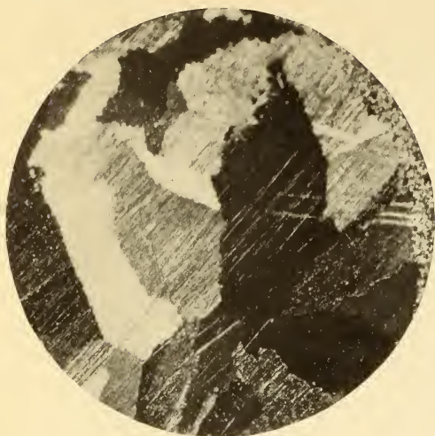
A , Specimen 418; 5X. The right edge shows a trace of the peripheral layer of fine recrystallized metal due to the surface distortion of the tensile bar while being machined; heated for 30 minutes at 700° C. and cooled in the furnace. The macroscopic crystalline appearance of the greater part of the bar has been unchanged
