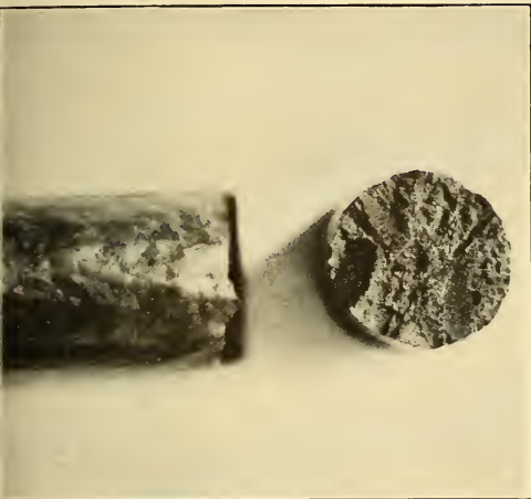
A, Specimen 36; 2X. Ultimate tensile strength, 42,450 pounds per square inch; elongation in 2 inches, 20.5 per cent; reduction of area, 20 per cent
