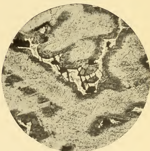
D, Specimen 568; 250X. The cracks (black) in the eutectoid (white) are at right angles to the direction of the strain
