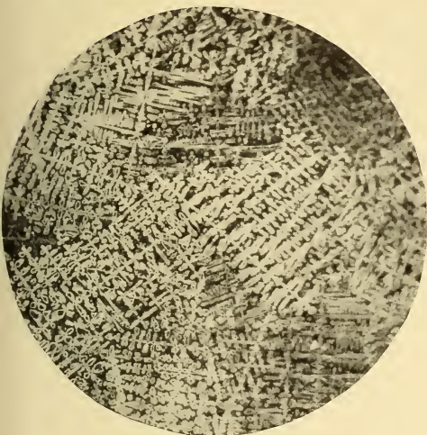
A, Specimen 19; 5X. Remelted and allowed to cool in the furnace. The difference in orientation of the dendritic structure marks out the various crystals
