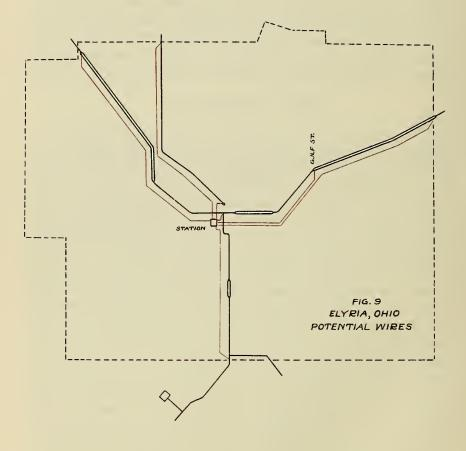
company to determine in a general way the conditions of their tracks at any time by simply taking measurements on these lines at frequent intervals. Any sudden or abnormal change in the resistance of the unknown return system can at once be detected and repairs promptly made.
