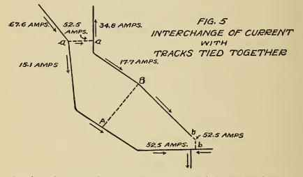
tribution of current flow on the tracks thus tied together is shown in detail below for average conditions of traffic.
