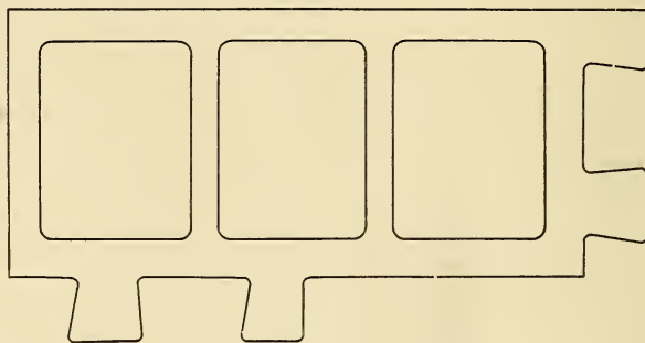
FIG. 5.—Cross section of corner tile
