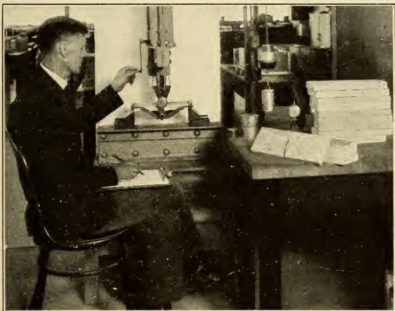
FIG. 9.—Apparatus for making transverse strength and elasticity tests
