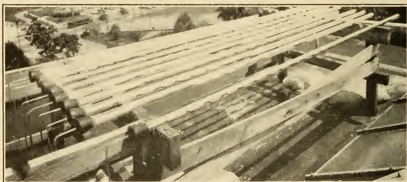
FIG. 3.—Tubes used for exposing samples in a vacuum to sunlight
