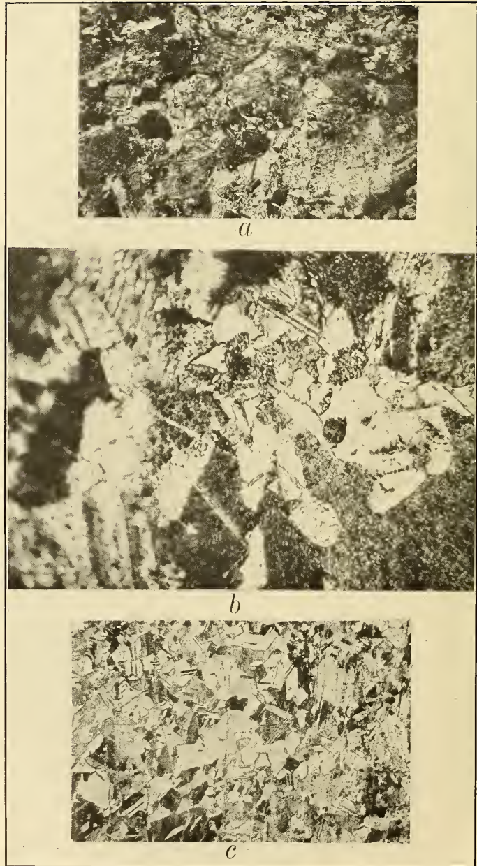
FIG. 12.—Effect of heating for long periods of time on the microstructure of Lot C tubing. (Compare fig. 11)
