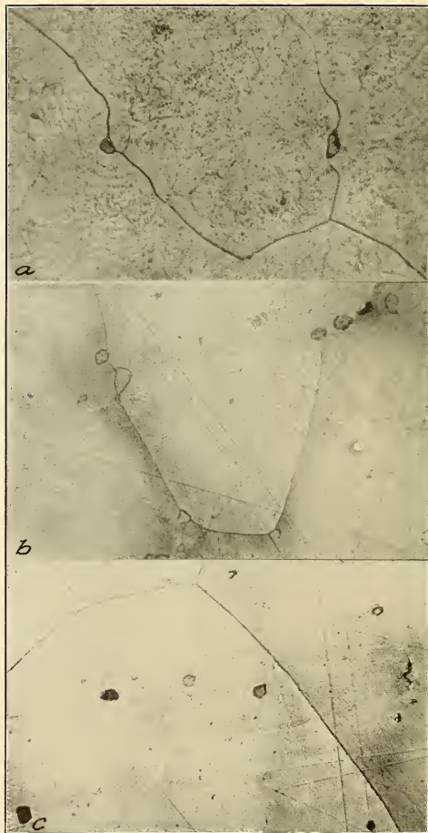
FIG. 6.—Occurrence of sulphur in a commercial melt of Monel metal as affected by metallurgical treatment, X500
