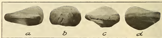
FIG. 1.—Appearance of a set of forged nickel specimens illustrating the effect of additions upon malleability, \times 1
