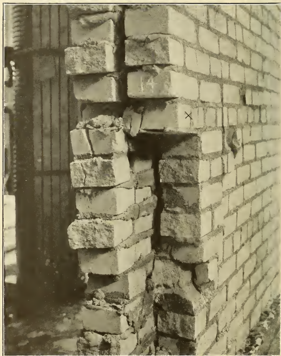
FIG. 3.—Wall No. 14 after ultimate load had been reached, 8 inches thick, cement mortar
