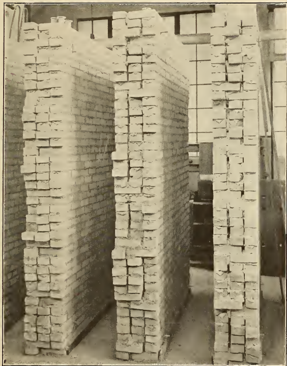
FIG. 2.—Brick walls 12½ inches thick, cement mortar
