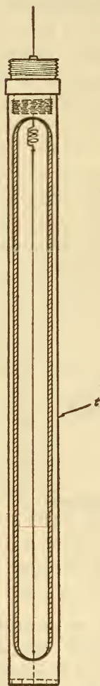
FIG. 24.—Separable mounting for conductivity cell.
