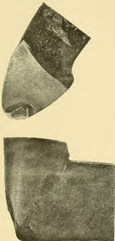
FIG. 1.—Showing tool with "Cutting edge still good but deep groove worn or guttered in the lip surface by the pressure of the chip," from Taylor's Art of cutting metals , Fig. 17e. In other cases, small particles of the chips scraped from the forging are pressed or welded into a compact pile on the lip surface of the tool
