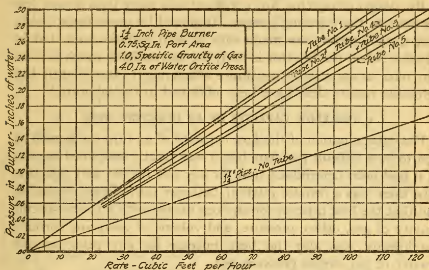
FIG. 15.—Relative air injection with injecting tubes of different designs as indicated by the pressure in the burner
