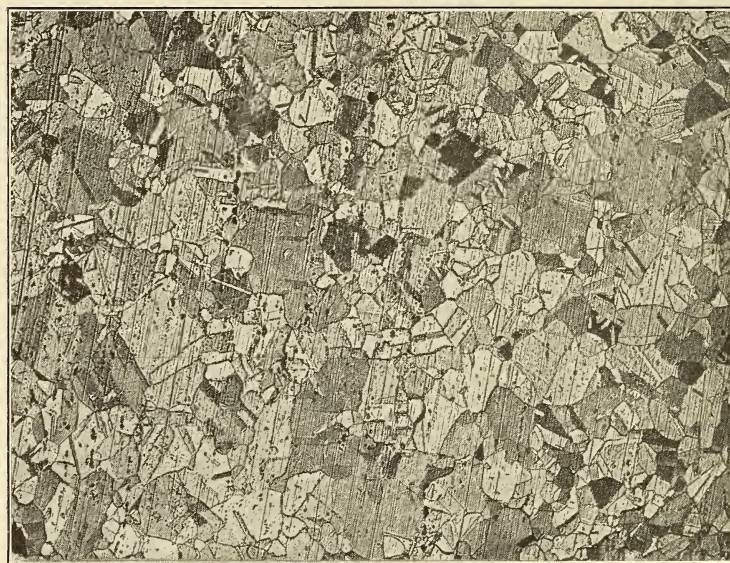
FIG. 9.—Longitudinal section of copper cylinder annealed at 650° C. \times 100
