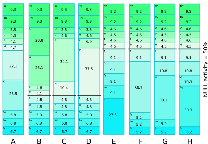
Fig. 6. Error division diagrams for eight recognizers showing, from top to bottom, the percentage of frames that were true positives, true negatives, overfills, underfills, fragmentations, merges, insertions, deletions, substitution-fragmentations, substitution-merges, and substitutions. The dark horizontal bar in each column indicates the division between severe errors and those that may be tolerable.
