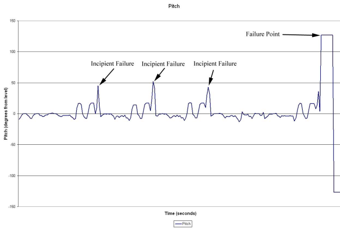
Fig. 5. Plot of pitch over time for robot 1 showing a failure presaged by fluctuations in pitch angle.
