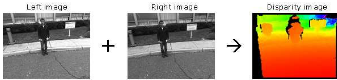
Fig. 2. Compute depth map from the stereo images.
