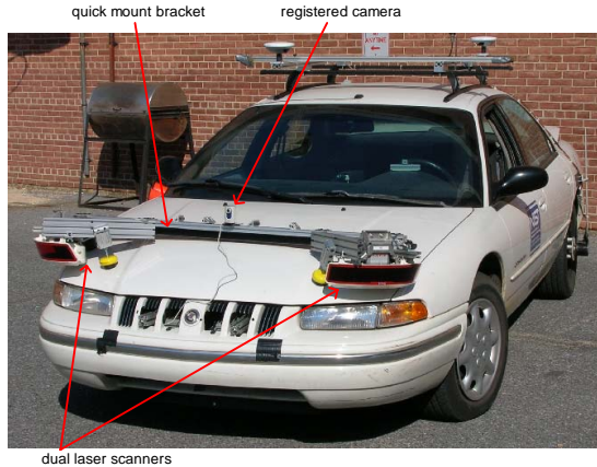
Figure 1 NIST/DOT test bed vehicle with dual-head laser-range scanner mounted on front hood.
