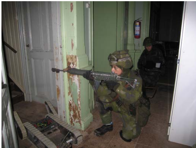
Figure 2. To the lower left the PackBot Scout robot, the robot assistant in the center and the robot operator in the upper right. The robot is about to drive up the staircase to the left, the assistant is ready to act in the most hazardous direction which is in this case considered to be the staircase. The operator is controlling the robot from a previously secured area.
