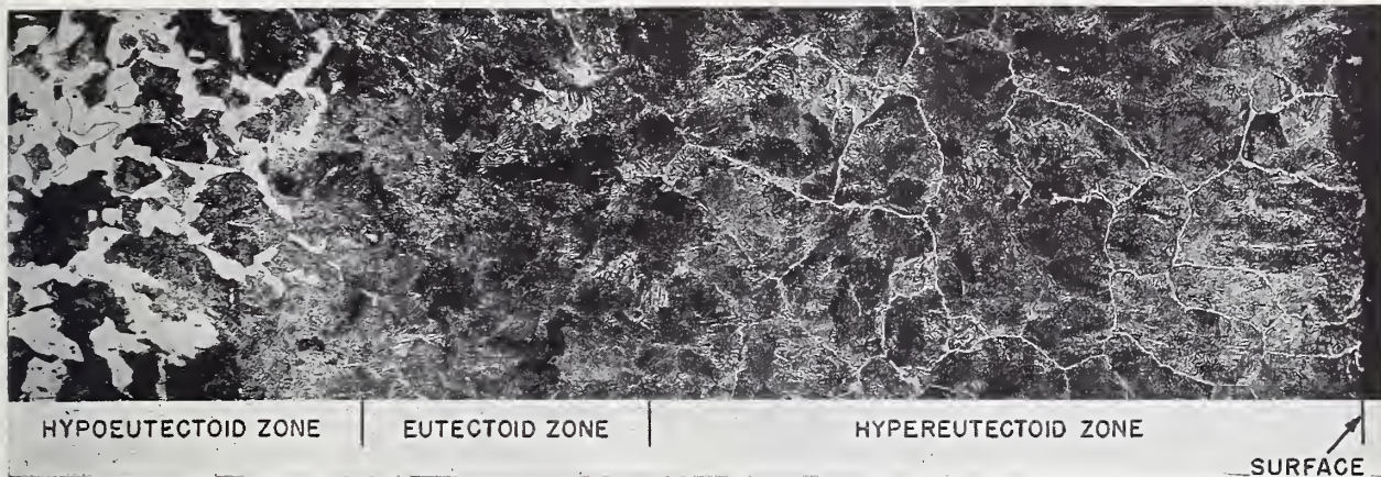
FIGURE 18. Structure of a carburized steel.
