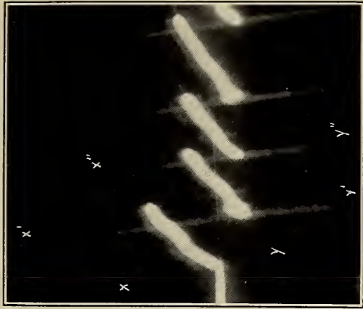
FIGURE 18.—Magneto circuit arrangement similar to that used in Figure 15 with sphere gap in air replacing spark plug in \text{CO}_2 . The sloping lines indicate improper adjustment of the cathode tube.
