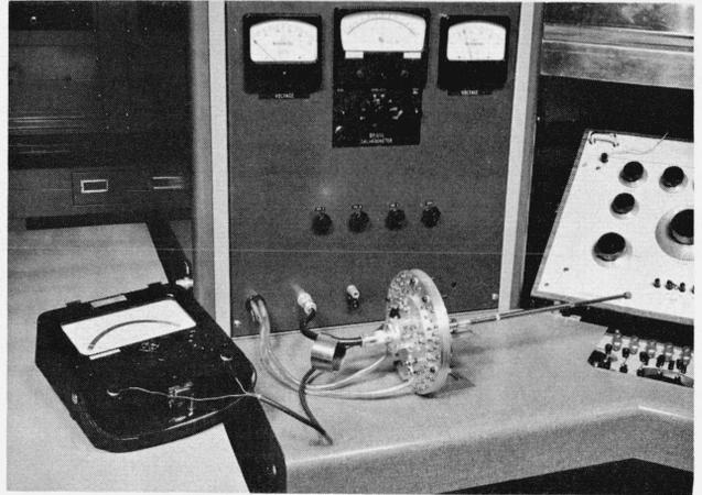
FIGURE 9j. Bolovac set up to calibrate thermoelement.
