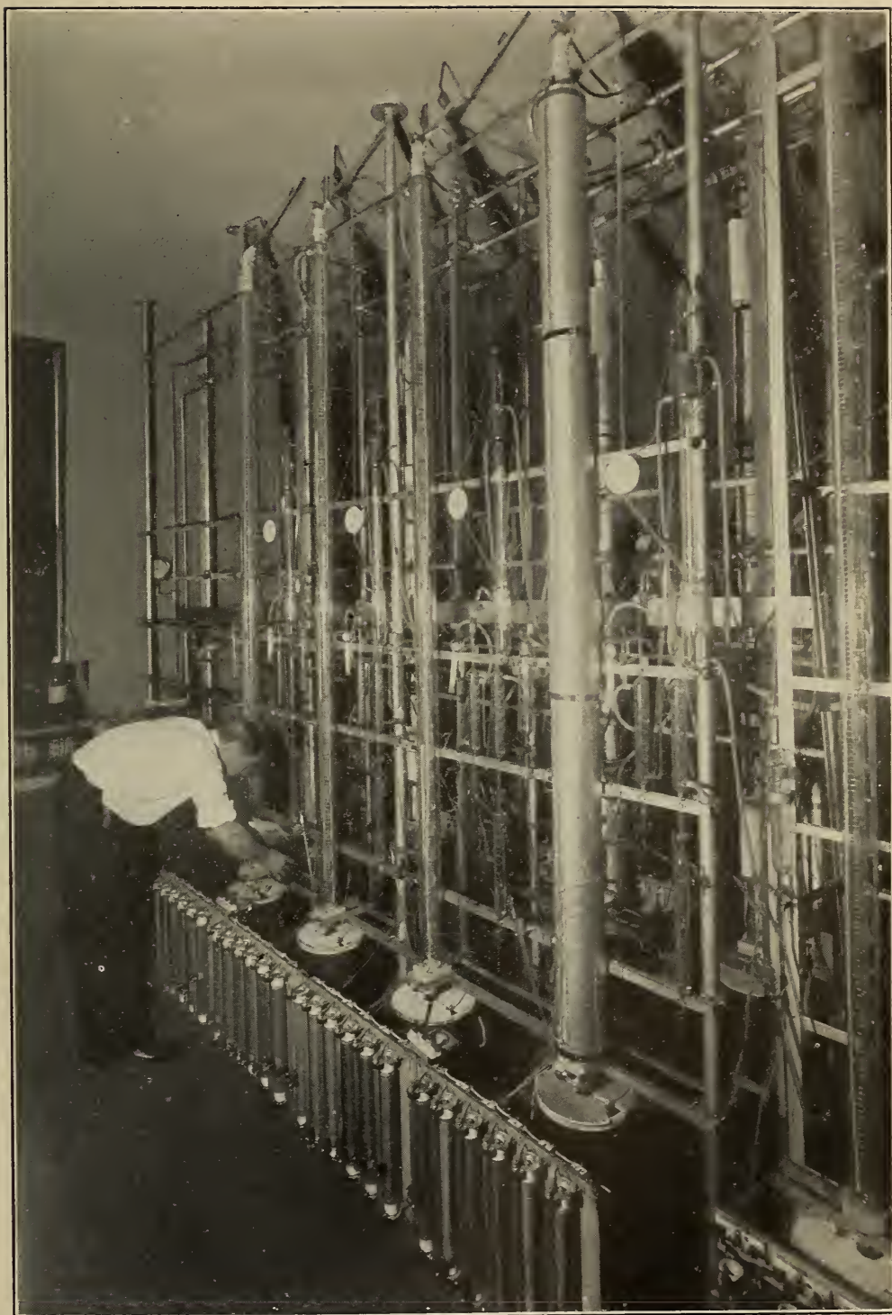
FIGURE 16.— Assembly of five 30-plate bubbling cap stills mounted on a single frame
