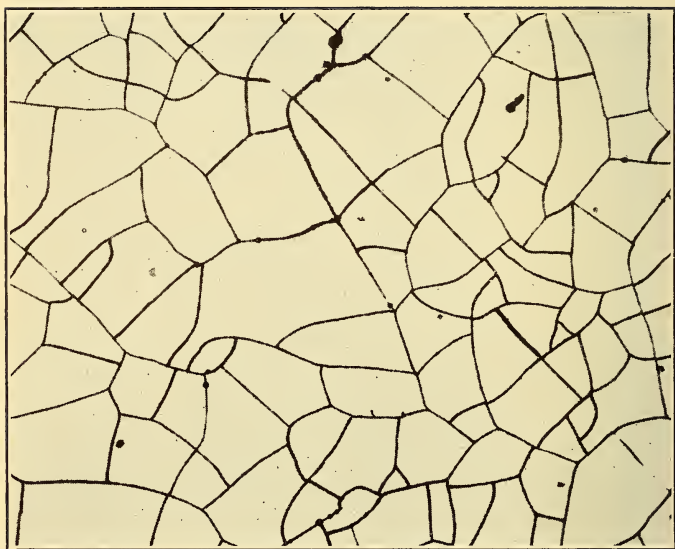
FIGURE 3.— Random cracks in thick chromium coatings on nickel ( \times 100 )
