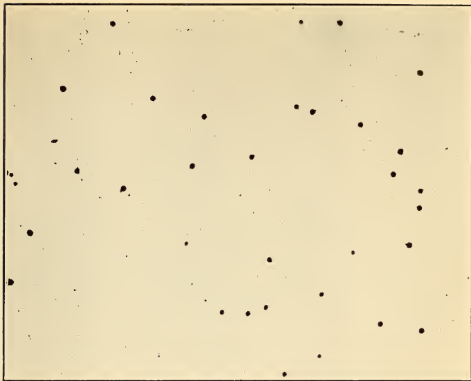
FIGURE 1.— Pores in thin chromium coatings on nickel ( \times 40 )
