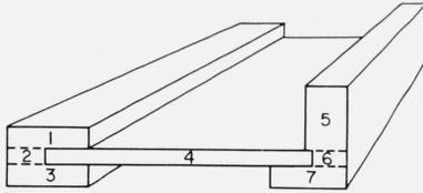
FIGURE 8. A conductor of complicated cross-sectional area divided into elements whose inductances can be calculated.
