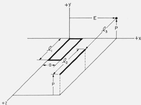
FIGURE 2. A filament parallel to a thin tape whose mutual inductance is given by eq (6).
