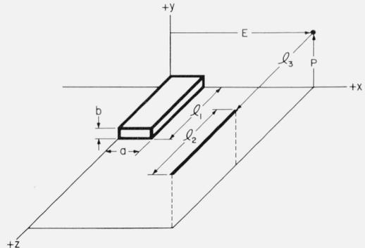
FIGURE 5. A filament parallel to a rectangular bar whose mutual inductance is given by eq (12).
