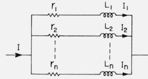
FIGURE 9.—An equivalent circuit of the conductor shown in figure 8.
