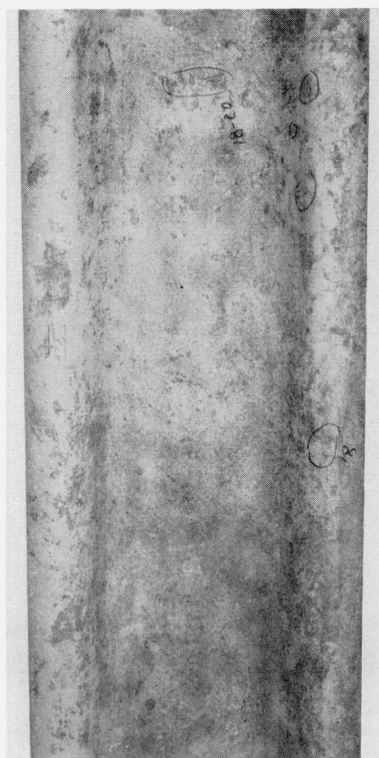
FIGURE 2. Sandblasted 3-ft section from the 40-year-old piling extracted from an abutment wall in the Corps of Engineers Dam and Lock No. 8 on the Ouachita River near El Dorado, Arkansas.
