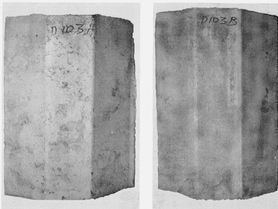
FIGURE 3. Sections (1.5 ft by 1 ft) cut from a piling which was pulled from the north upstream wingwall of the Grenada Dam Spillway at Grenada, Mississippi, after exposure for 12 years.
