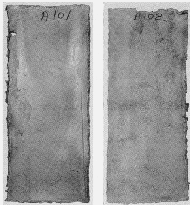
FIGURE 5. Steel sheet piling sections (2 ft by 1 ft) cut from two locations on the Memphis Floodwall after exposure for 6.3 years.
