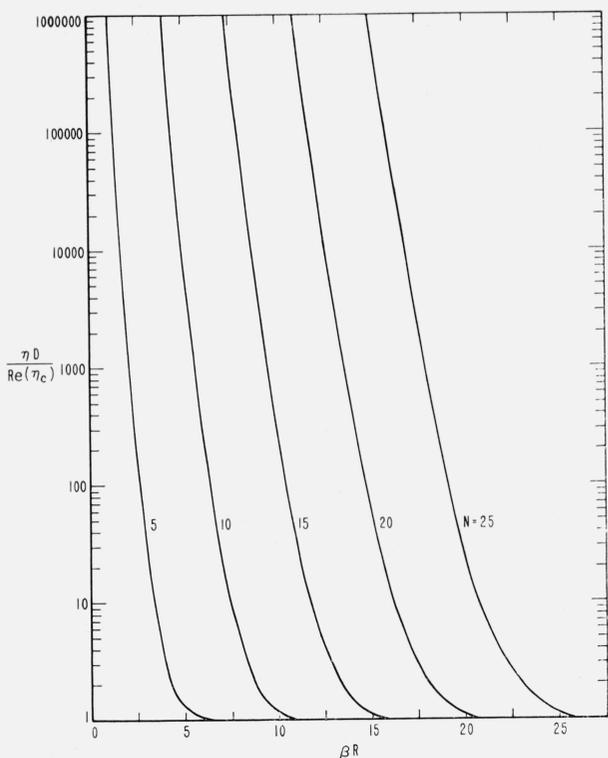
FIGURE 6. Dissipation factors ( $D$ ) for ideal lossy antennas adjusted for maximum gain at infinity, using wave functions of order  $n \leq N$ .
