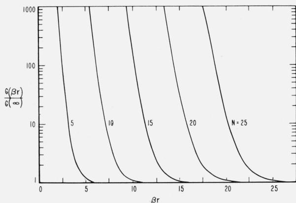
FIGURE 3. Ratio of the maximum gain at a distance  $r$  to the maximum gain at infinity, using wave functions of order  $n \leq N$ .
