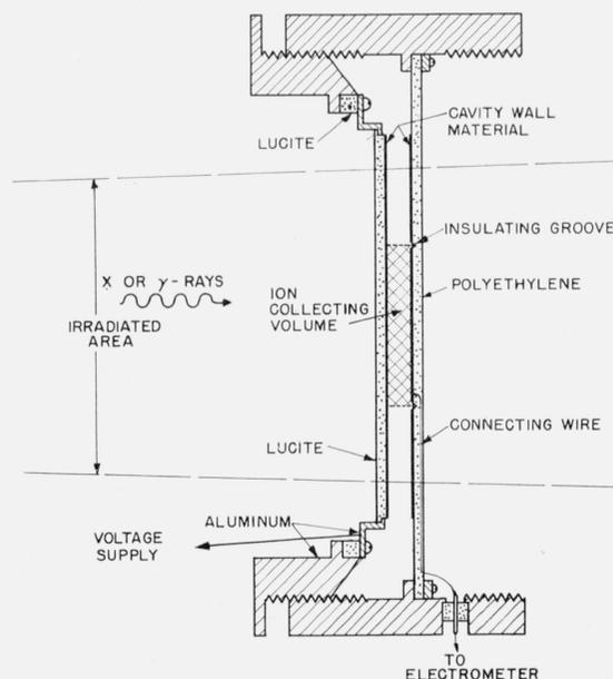
FIGURE 1. Cross section of experimental ionization chamber.
