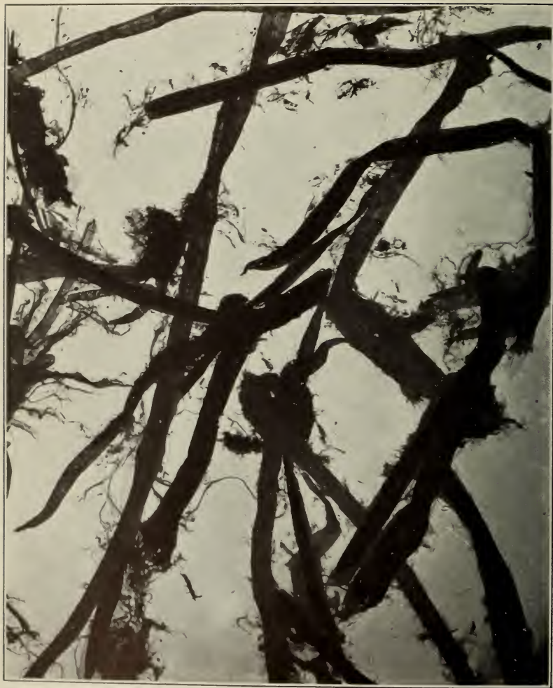
FIGURE 6.—Fibers from sulphite bond paper after being ground in paper disintegrator. \times 100
