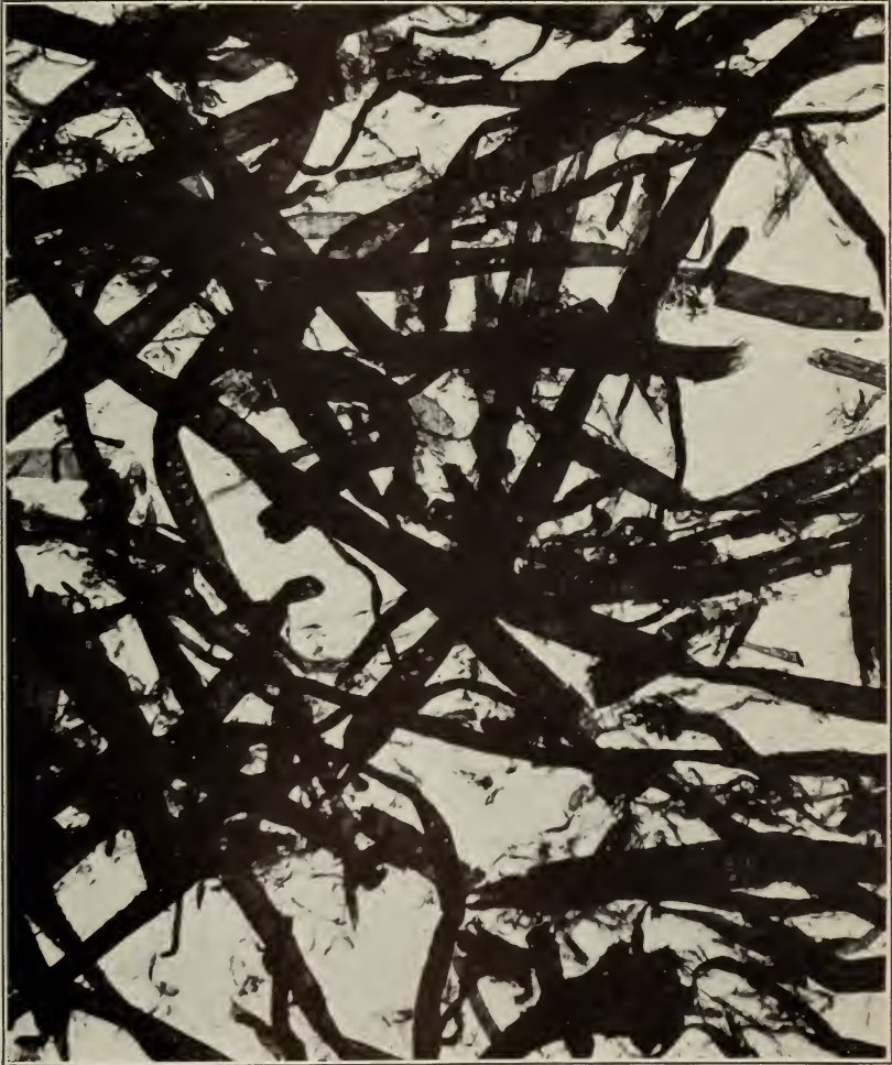
FIGURE 5.—Fibers from unground sulphite bond paper. \times 100
