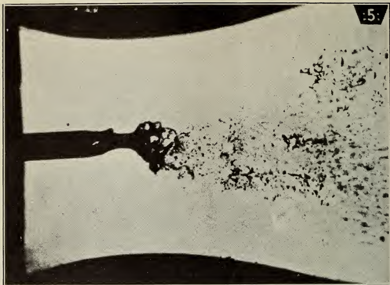
FIGURE 2.—Atomization of water in model of carburetor throat (Scheubel). Air speed about 5,300 cm/sec.
