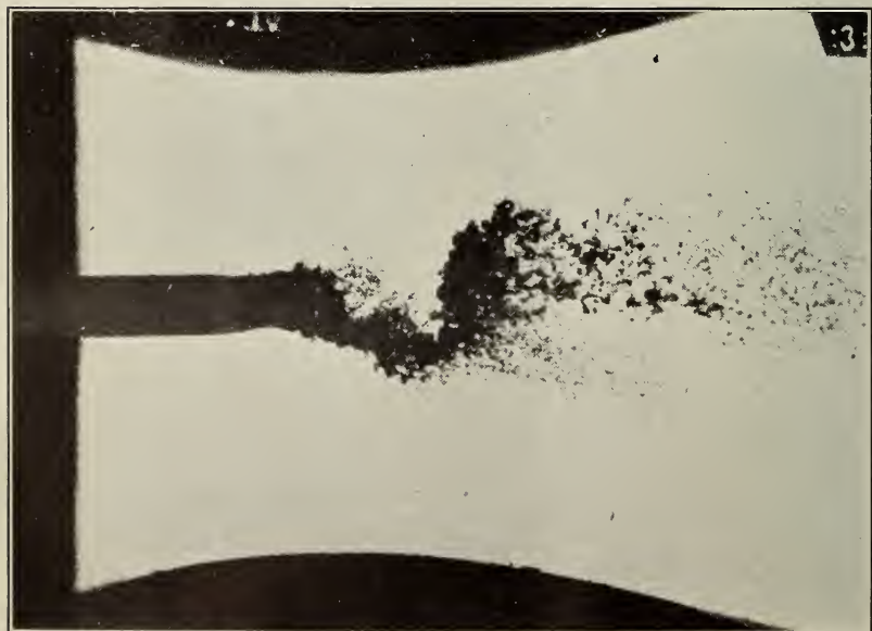
FIGURE 3.—Atomization of water in model of carburetor throat (Scheubel). Air speed about 10,500 cm/sec.
