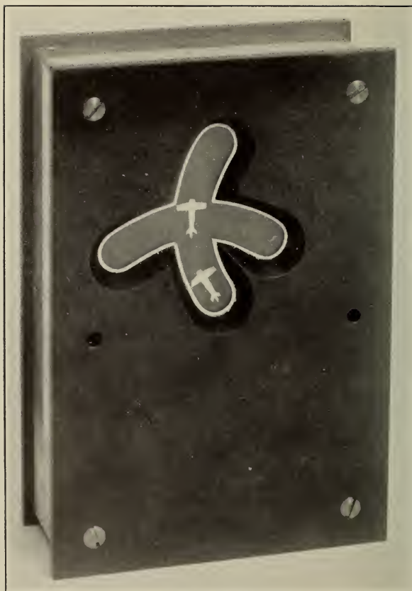
FIGURE 14.— Combined instrument giving indications of the relative position of the airplane with respect to the runway and also with respect to the high-frequency landing beam path
