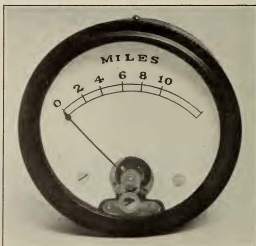
FIGURE 10.—Rough distance indicator used on the pilot's instrument board to show the approximate distance of the airplane from the runway localizing beacon transmitter
