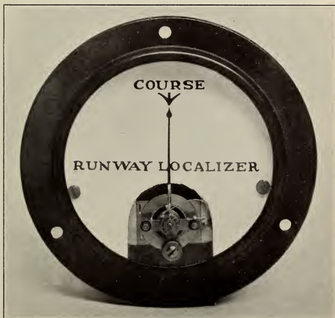
FIGURE 13.— Pointer type localizing beacon course indicator
