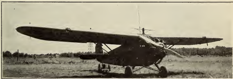
FIGURE 8.—Bureau of Standards' experimental airplane showing horizontal doublet antenna used for receiving the landing beam signals
