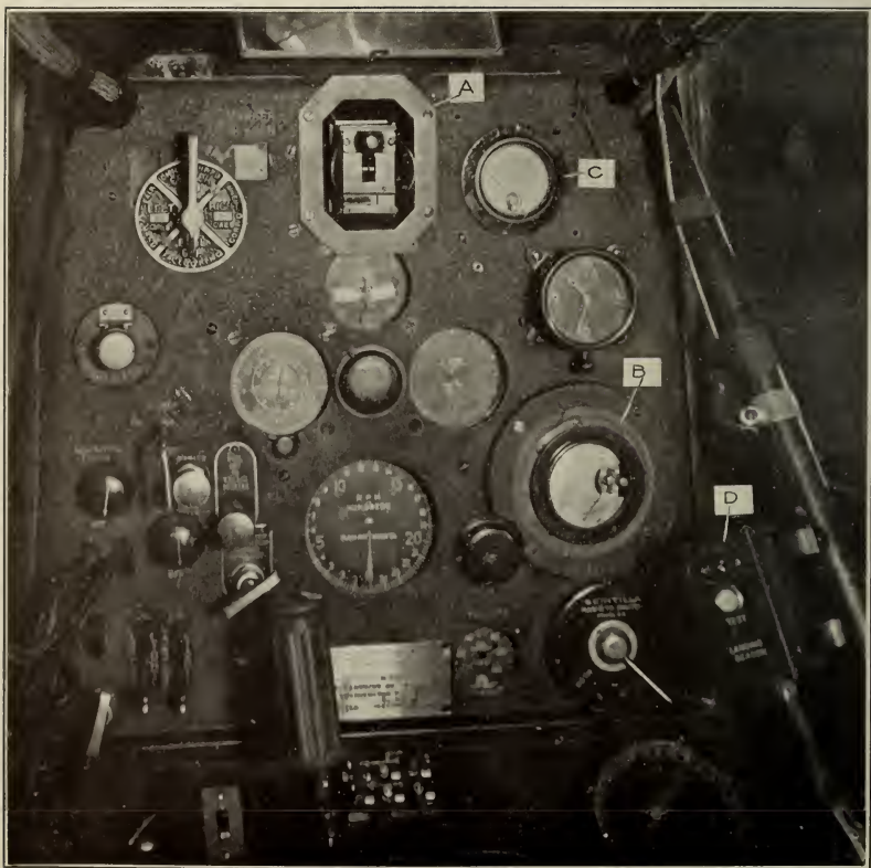
FIGURE 12.—Instrument board on Bureau of Standards' experimental airplane, showing vibrating reed-course indicator A, landing beam indicator B, rough distance indicator C, and landing beam runway set control and test panel D
