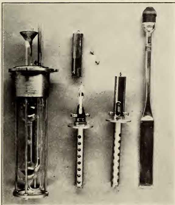
FIGURE 8.— Mounted electrolytic cell, two thermoregulators one with cover removed, and heating element
