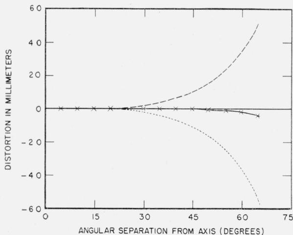
FIGURE 7. Linear distortion of camera lens, rectifying system, and final rectified print.
