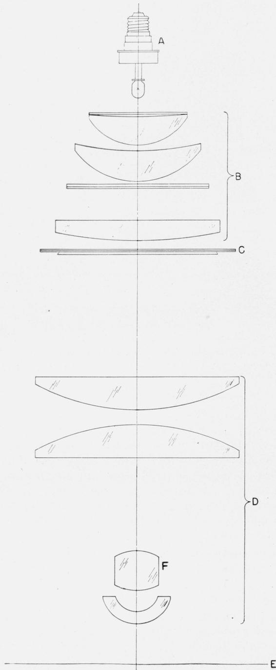
FIGURE 6. Optical system of the Pleon rectifier.
