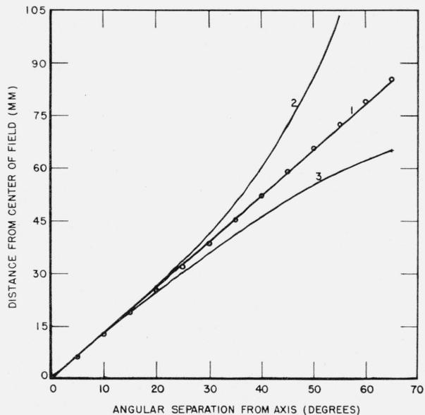
FIGURE 3. Relation between distance of image point from center of negative and angular displacement of corresponding object point from the axis for the Pleon lens.
