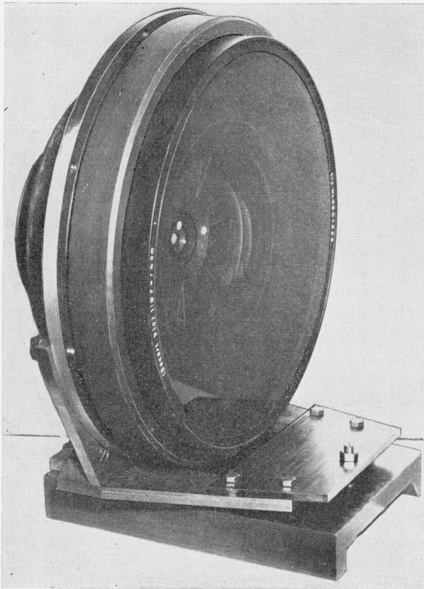
FIGURE 1. Pleon lens as mounted on a laboratory support for testing.
