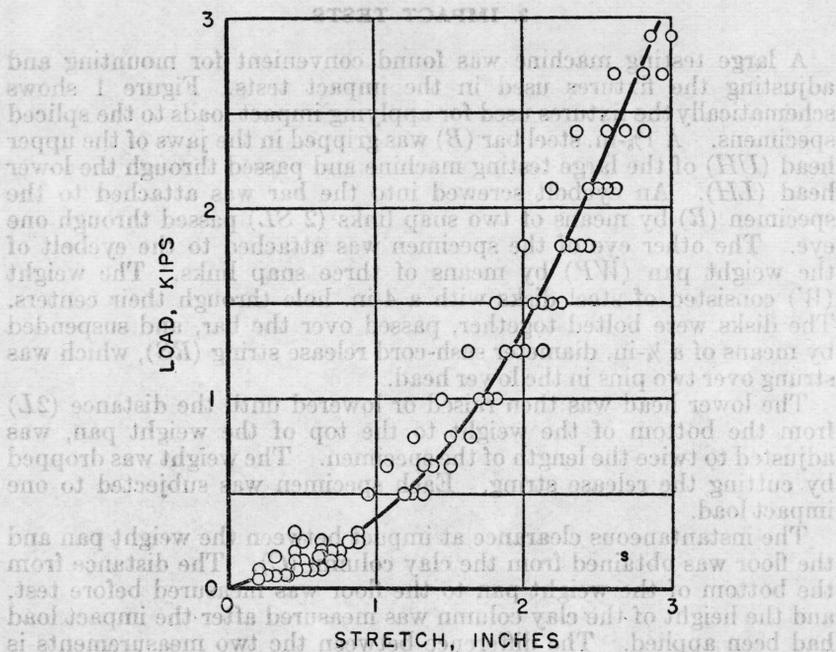
FIGURE 2.—Load-stretch curve for eye and splice lengths of sisal static-test specimens
