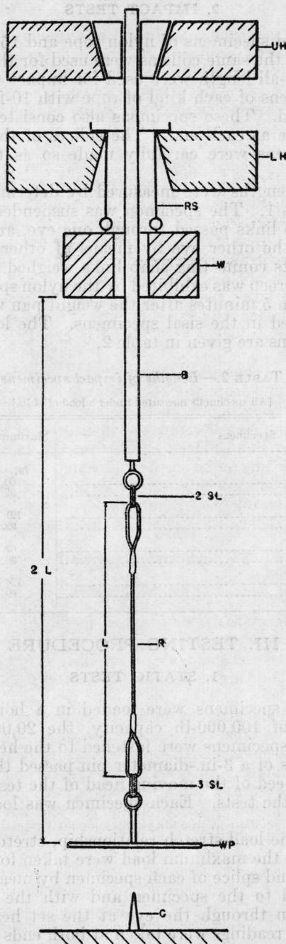
FIGURE 1.—Schematic diagram of impact-test setup.
