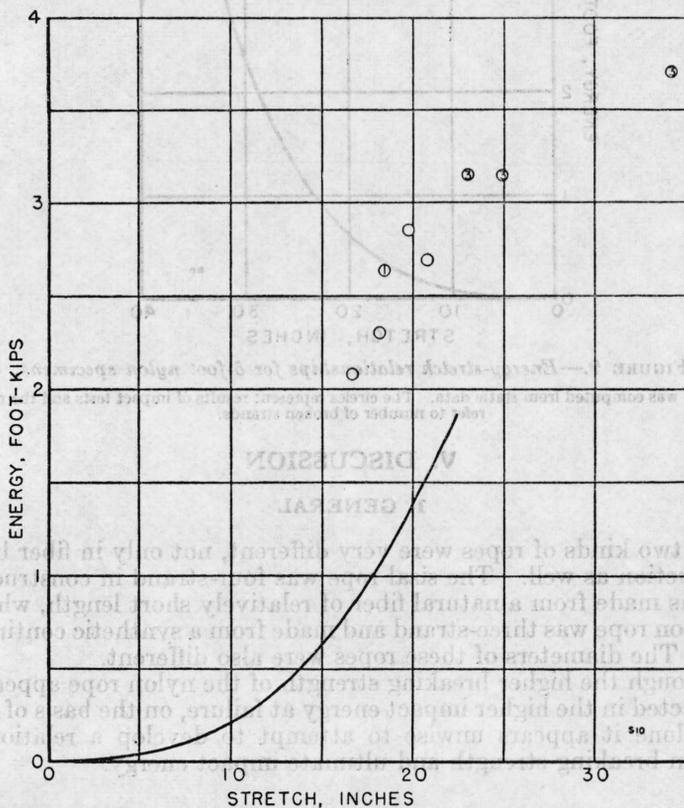
FIGURE 8.—Energy-stretch relationships for 10-foot sisal specimens.
