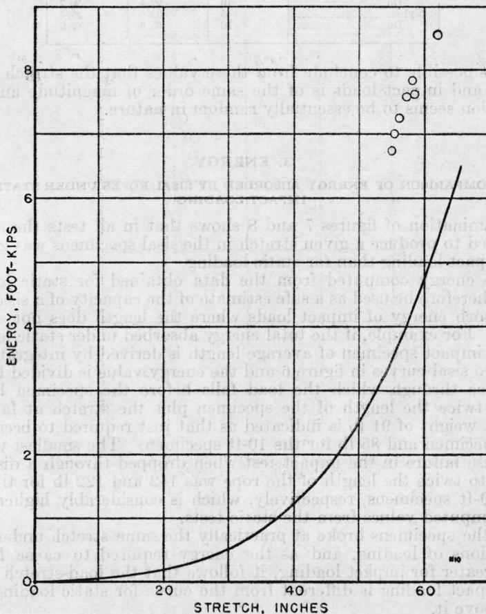
FIGURE 10.—Energy-stretch relationships for 10-foot nylon specimens.
