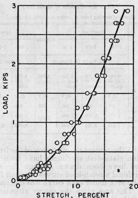
FIGURE 4.—Load-stretch curve for free length of sisal static-test specimens.
