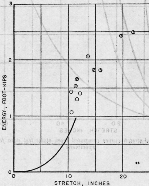
FIGURE 7.—*Energy-stretch relationships for 5-foot sisal specimens.*
