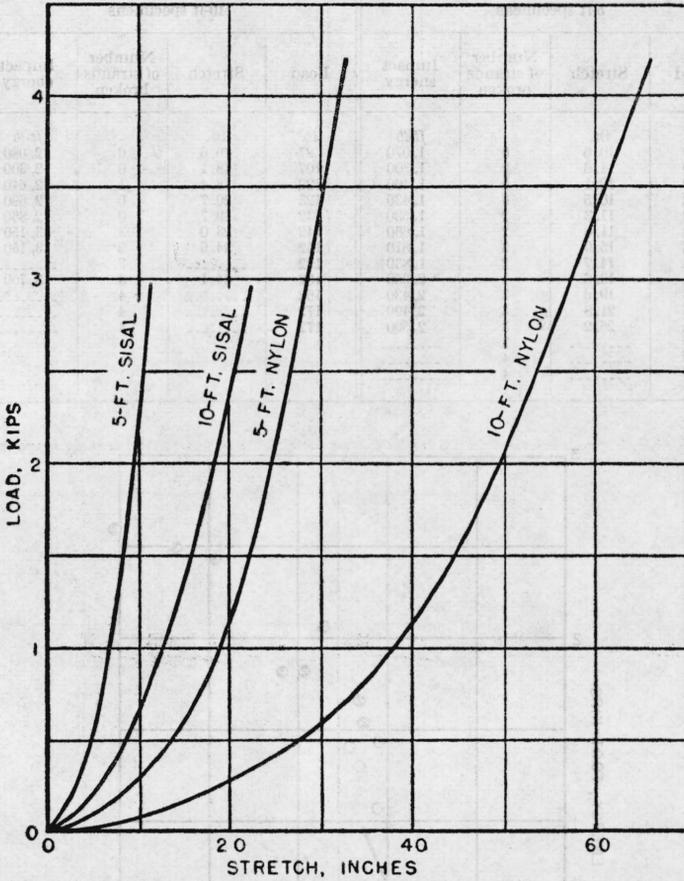
FIGURE 6.—Load-stretch curves computed from static-test data for impact-test specimens.
