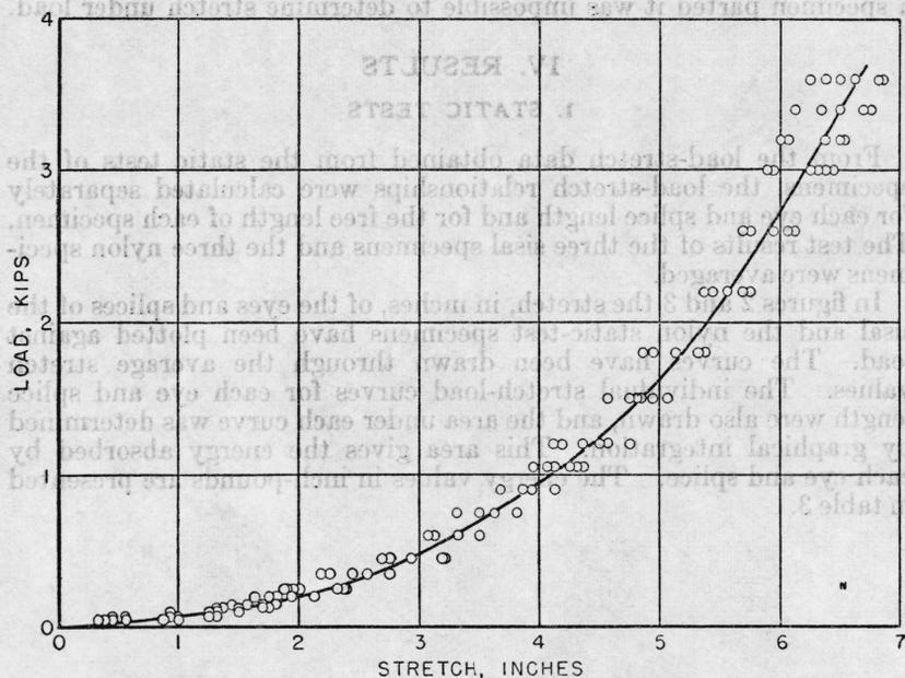
FIGURE 3.—Load-stretch curve for eye and splice lengths of nylon static-test specimens.
