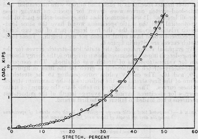
FIGURE 5.—Load-stretch curve for free length of nylon static-test specimens.
