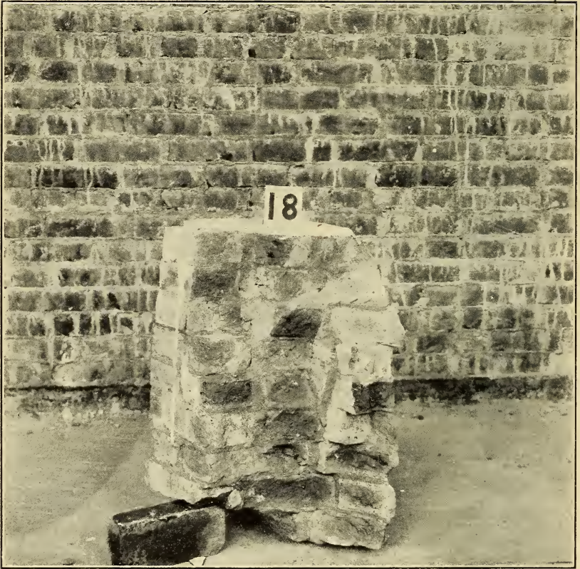
FIGURE 13.— A portion of wall 18 after test
