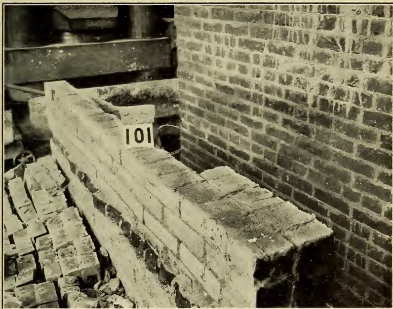
FIGURE 10.— The mortar bed in a wall of series 2
