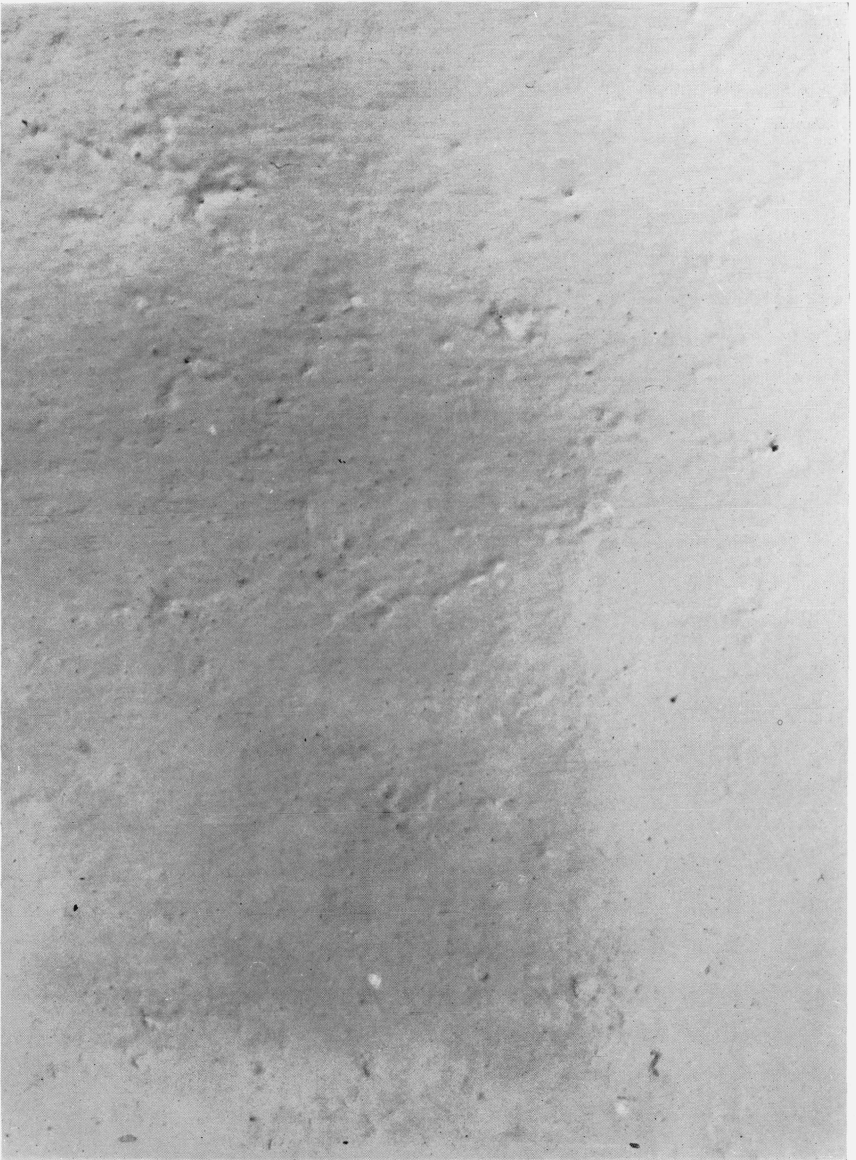
FIGURE 18.— Surface appearance of sample 8a when brush painted five additional coats and magnified two-thirds times.
