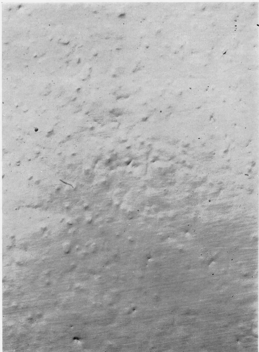
FIGURE 20.— Surface appearance of sample 9a when brush painted five coats and magnified 1\frac{2}{3} times.
