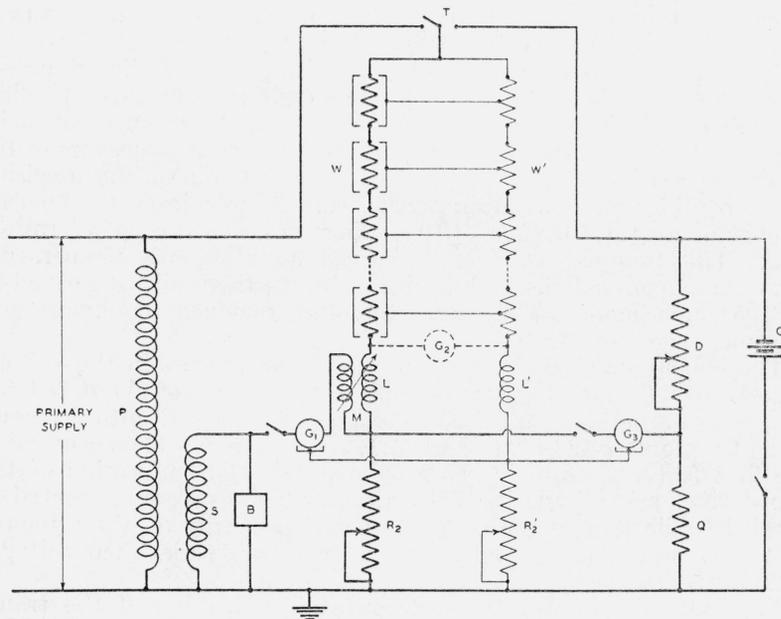
FIGURE 2.—Circuit used in measuring the ratio and phase angle of voltage transformers.
