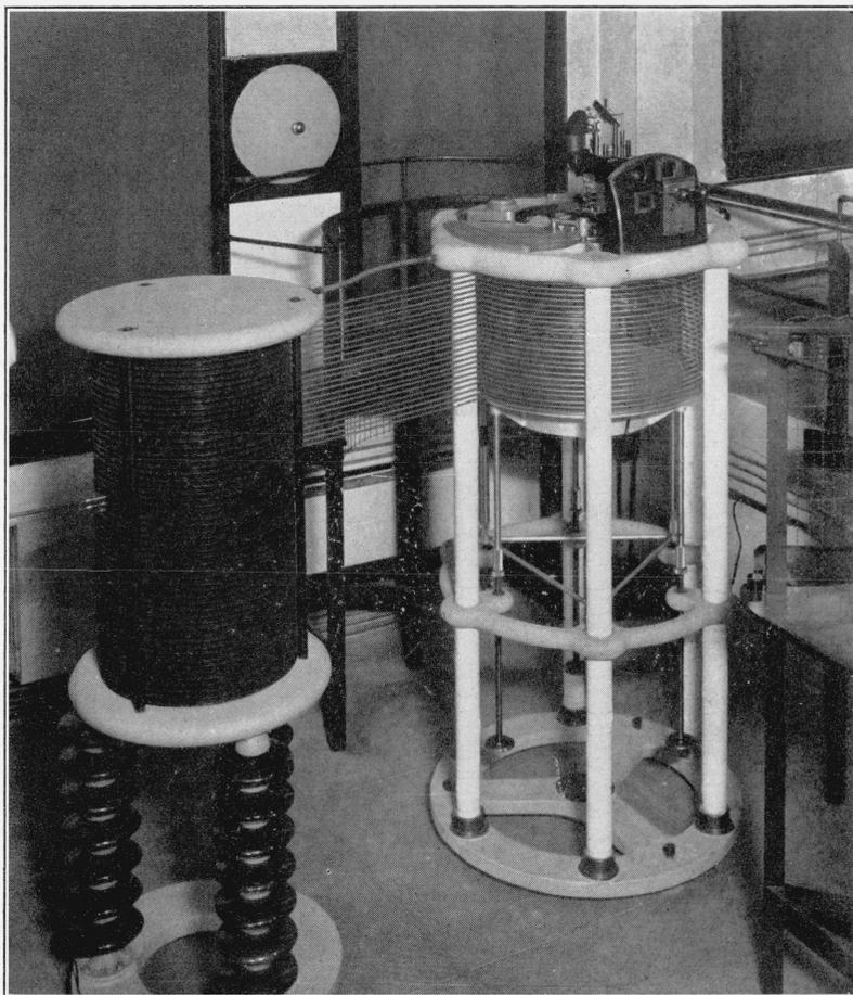
FIGURE 4.—*Brooks absolute electrometer.*
