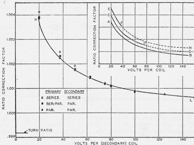
FIGURE 3.—Ratio correction factor as a function of secondary voltage.
