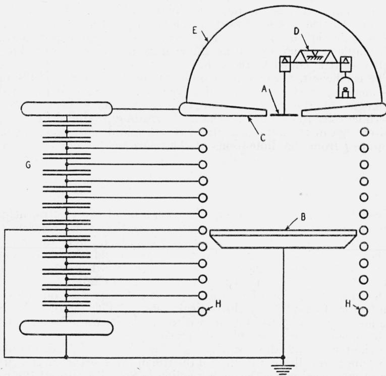
FIGURE 5.—Schematic cross section of Brooks absolute electrometer.
