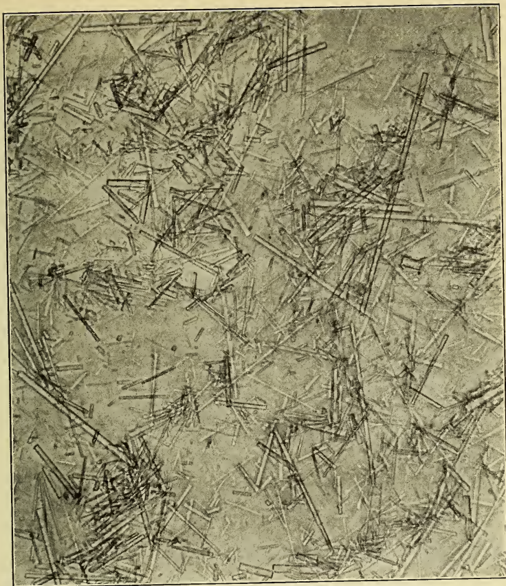
FIGURE 1.— Calcium sulphoaluminate needles. High sulphate form. Analyzer out. \times 200
