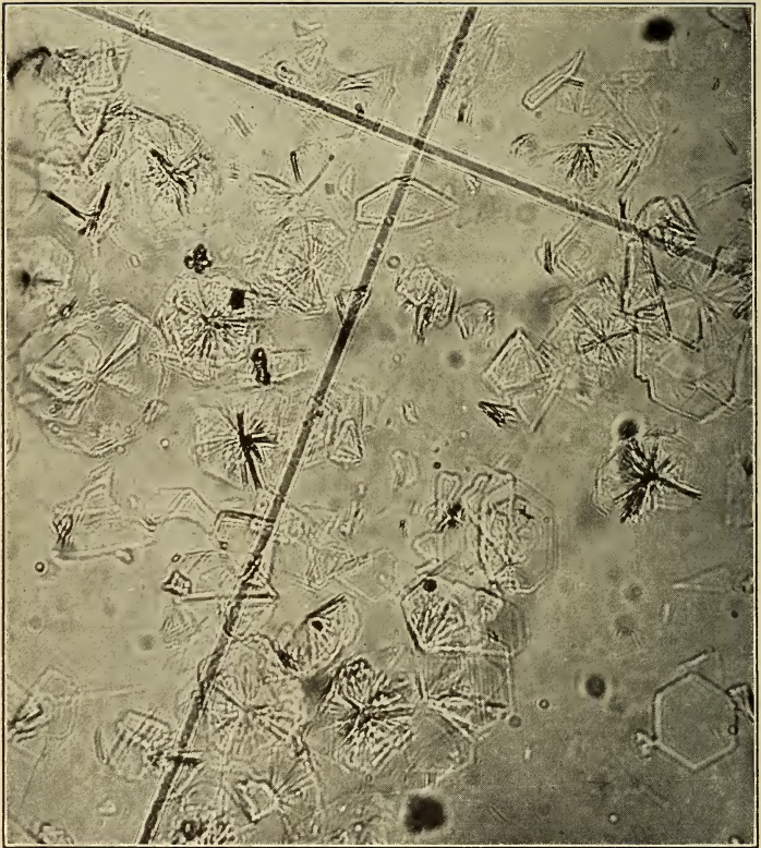
FIGURE 6.— Low sulphate calcium sulfoaluminate showing the platy form. Analyzer out. \times 200
