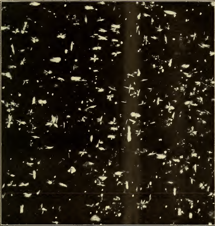
FIGURE 5.— Low sulphate calcium sulphoaluminate. Crossed nicols. × 200
