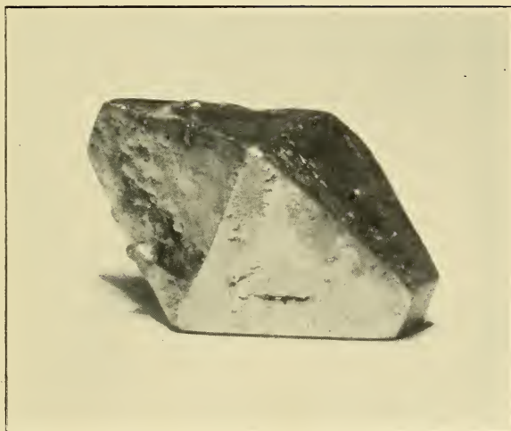
FIGURE 1.— Crystal of gallium, weighing 2.2 grams. Approximately 4 times actual size.
