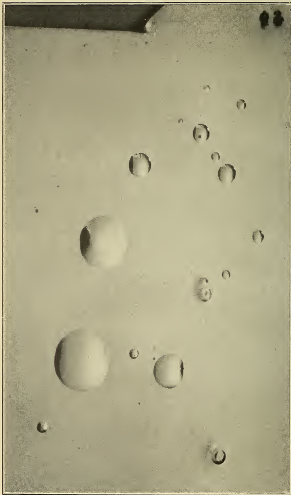
FIGURE 6.—Large blisters that formed on storage of many of the specimens with a zinc or cadmium layer under the nickel. Natural size.
