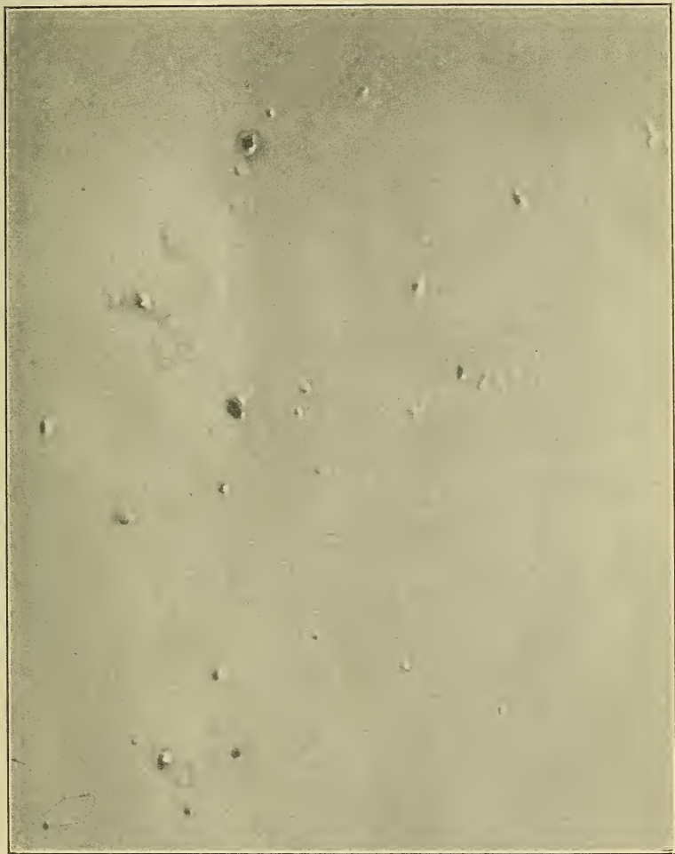
FIGURE 5.— Small blisters observed after long exposure of many chromium-plated specimens, especially in marine locations. \times 5 .
