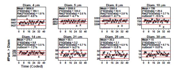
Fig. 17. Results of SRM 2806b final material step 3: homogeneity and stability plots. Axis labels for all plots are the same as those given on the lower-left plot. The horizontal axis represents the 40 measurements (40 bottles) which are distributed over the approximate 2 h sampling time.
