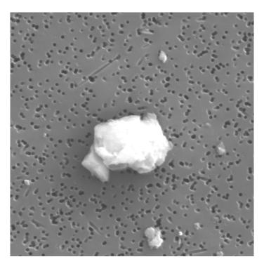
Fig. 4. SEM micrograph of particles filtered from the refrigerated hydraulic oil for SRM 2806b. The image has a magnification of  $5000\times$ . The image is  $25.6~\mu m$  on side, and the filter pore size is a nominal  $0.4~\mu m$ .
