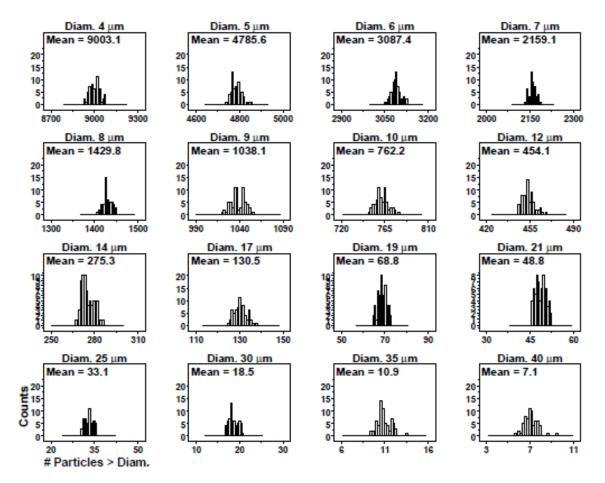
Fig. 10. Results of SRM 2806b later on-line data step 1: distributional check: histogram. Axis labels for all plots are the same as those given on the lower-left plot.
