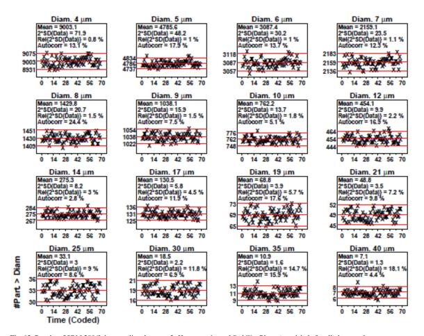
Fig. 12. Results of SRM 2806b later on-line data step 3: Homogeneity and Stability Plots. Axes labels for all plots are the same as those given on the lower left plot. The horizontal axis is the 68 measurements which are spaced over the approximate 2 h sampling time.
