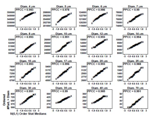
Fig. 6. Results for SRM 2806b early on-line data step 2: distributional check: normal probability plots. Axis labels for all plots are the same as those given on the lower-left plot.
