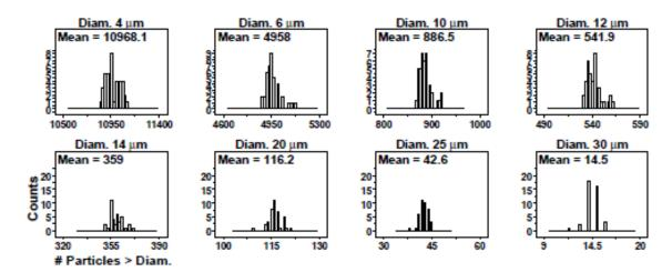
Fig. 20. Histogram plots for data collected on 40 bottles by IFTS for SRM 2806d step 1: distributional check: histogram. The vertical axis is the frequency or counts, and the horizontal axis is the cumulative particle concentration > specified diameter; axis labels for all plots are the same as those given on the lower-left plot.
