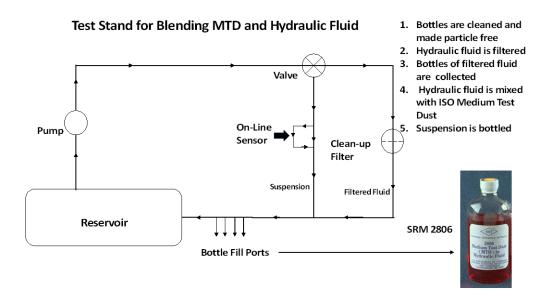
Fig. 1. Schematic of the IFTS process for manufacturing SRM 2806. The test stand system is equipped with an on-line particle sensor and ports to fill individual bottles with the hydraulic fluid medium—test dust (MTD) suspension. The purpose is to provide bottle-to-bottle homogeneity with regard to the cumulative particle concentration.
