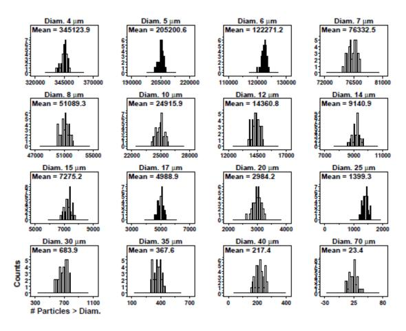
Fig. 5. Results for SRM 2806b early on-line data step 1: distributional check: histogram. Axis labels for all plots are the same as those given on the lower-left plot.
