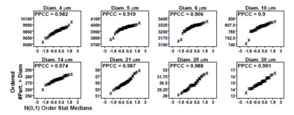
Fig. 16. Results of SRM 2806b final material: Step 2: Distributional check: normal probability plots. Axis labels for all plots are the same as those given on the lower-left plot.
