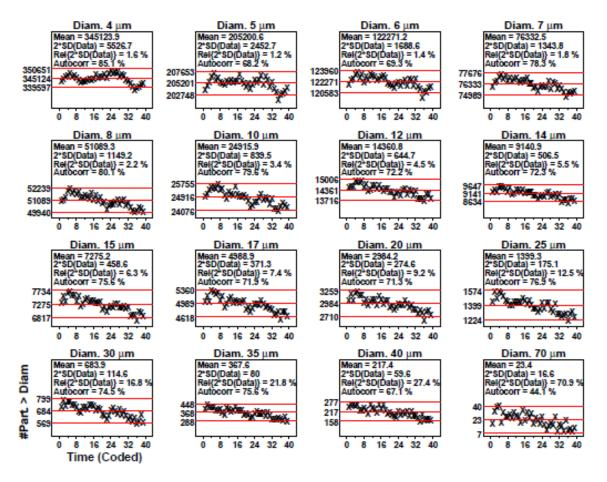
Fig. 7. Results for SRM 2806b early on-line data step 3: homogeneity and stability plots. Axis labels for all plots are the same as those given on the lower-left plot. The horizontal axis represents the 39 measurements which are distributed over the approximate 2 h sampling time.
