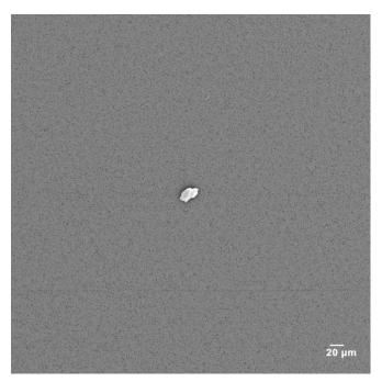
Fig. 2. SEM micrograph of filtered clean oil with image field of 0.5 mm.
