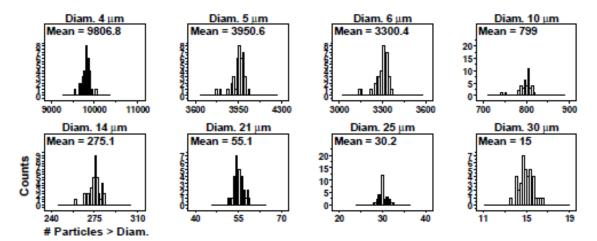
Fig. 15. Results of SRM 2806b final material step 1: distributional check: histogram. Axis labels for all plots are the same as those given on the lower- left plot.
