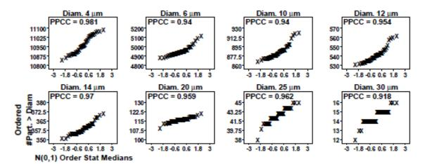
Fig. 21. SRM 2806d final material step 2: distributional check: normal probability plots, showing the cumulative particle concentration > specified diameter on the vertical axis and sorted theoretical values for a normal N(0,1) distribution on the horizontal axis. Axis labels for all plots are the same as those given on the lower-left plot.
