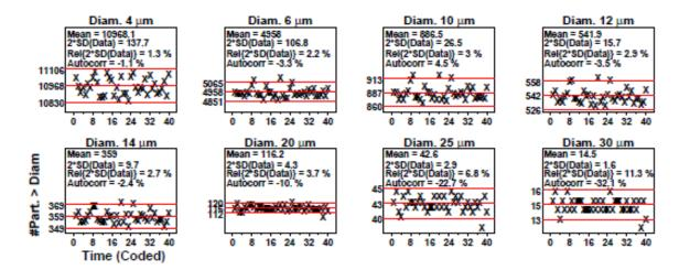
Fig. 22. SRM 2806d final material step 3: homogeneity and stability plots showing cumulative particle concentration > specified diameter on the vertical axis and the horizontal axis is the 40 measurements (40 bottles) which are distributed over the approximate 2 h sampling time.
