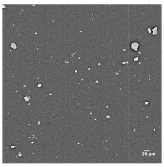
Fig. 3. SEM micrograph of filtered candidate SRM 2806b with image field of 0.5 mm.
