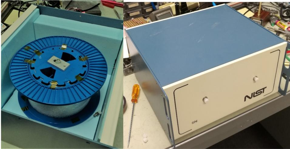
**Fig. 1.** Photographs of the NIST-built reference spool containing an approximately 10 km length of G.652 single-mode optical fiber.
