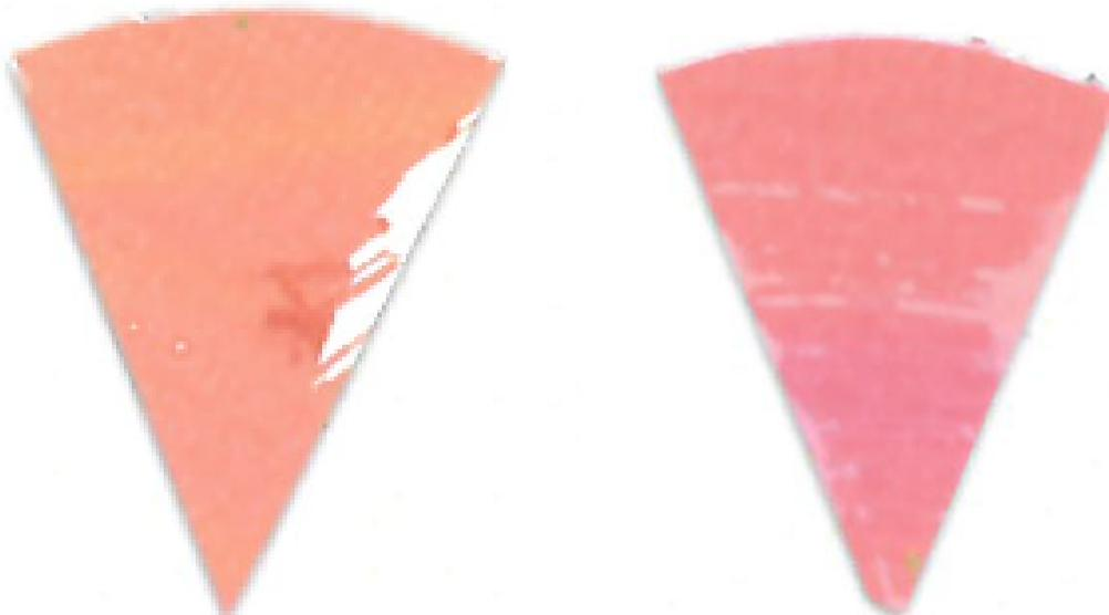
**Fig. 10.** Difference in color between top (left) and bottom (right) positions on a process challenge device in a polished aluminum foil experiment under 15 min exposure to UV-C light.
