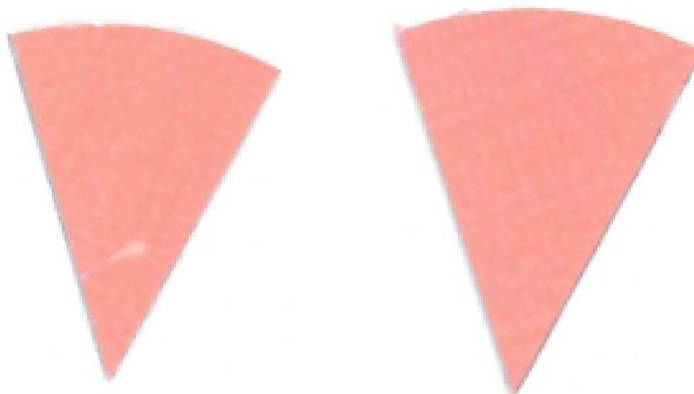
**Fig. 11.** Difference in color between top (left) and bottom (right) positions on a process challenge device in a PTFE experiment under 15 min exposure to UV-C light.
