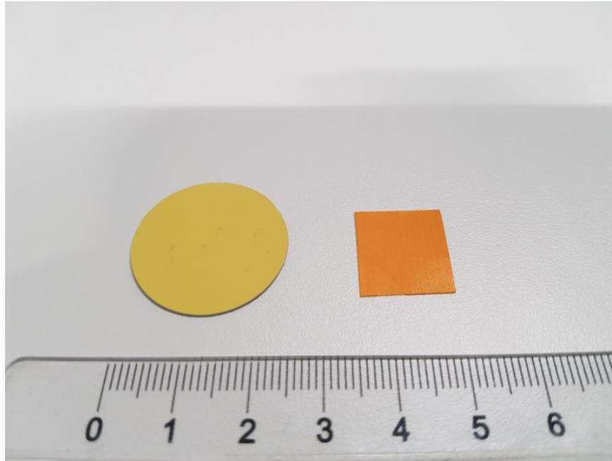
**Fig. 5.** UV-C indicators: Intellego Technologies UVC 100 (left) and Excelsior Scientific CPI-UV1E (right). Ruler is provided for scale purposes in cm.
