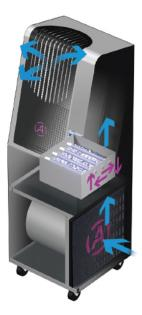
Fig. 15. Mobile UV-C air disinfection cart [29].
