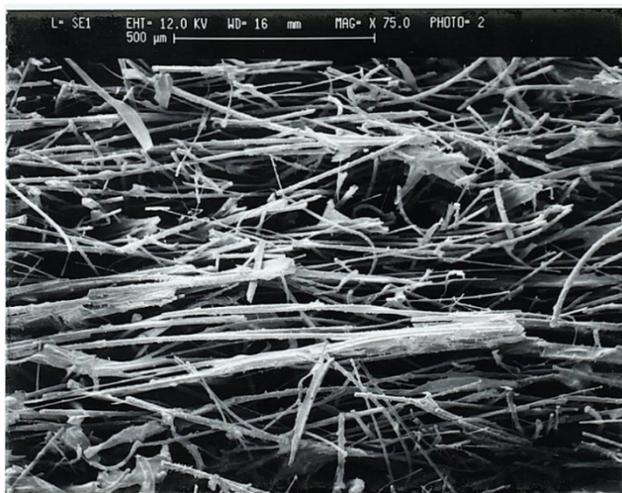
Fig. 2. SEM micrograph of part of SRM 1450c showing the shape of the fibers [29].
